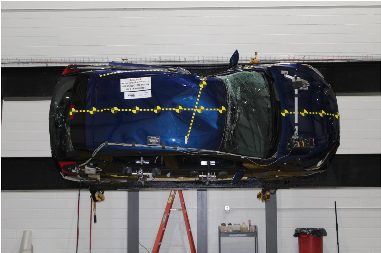
Figure A-64: FMVSS No. 301 Static Rollover 90 Degrees
