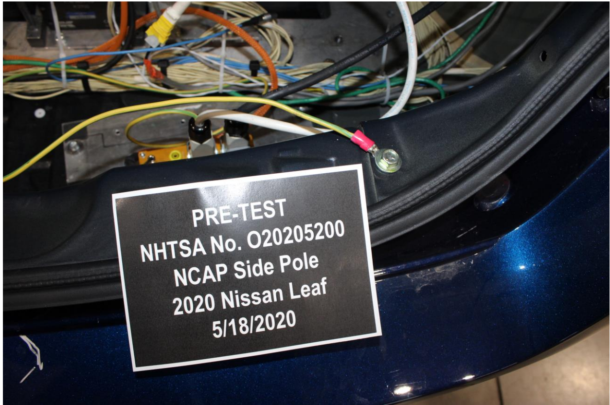
Figure 305-21: Pre-Impact View of Ground Lead Attached
