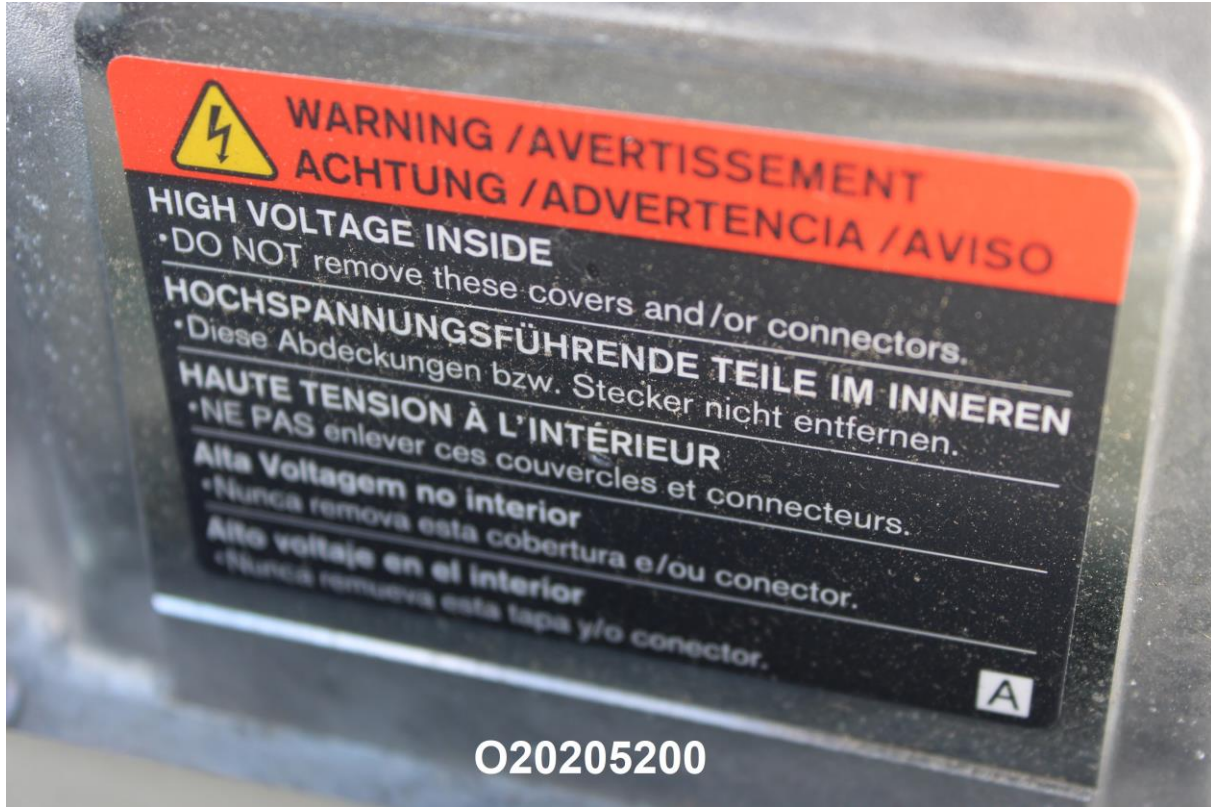
Figure 305-1: Auxiliary Power Module Warning Label
