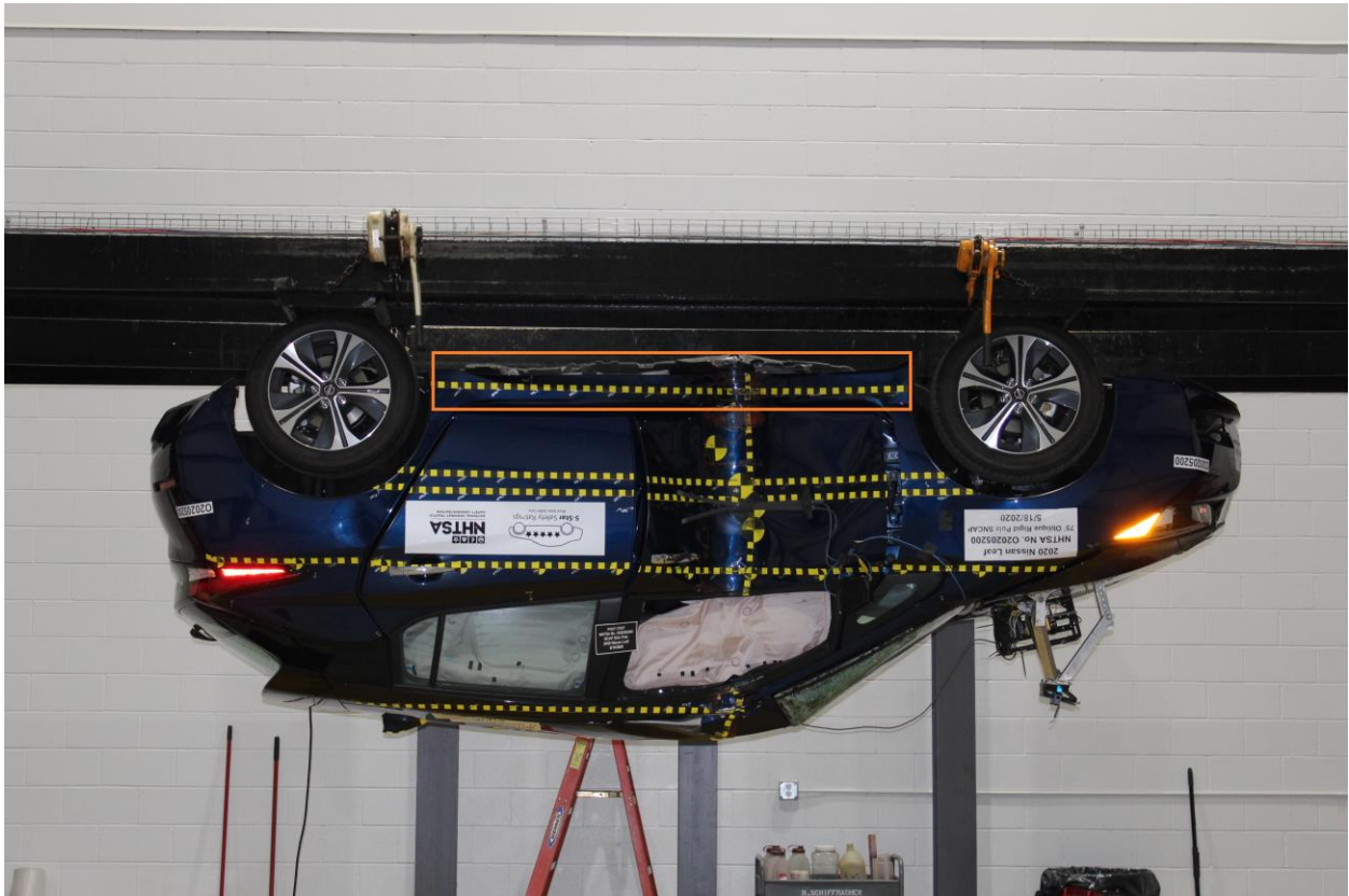
Figure 305-29: FMVSS No. 305 Static Rollover 180 Degrees
