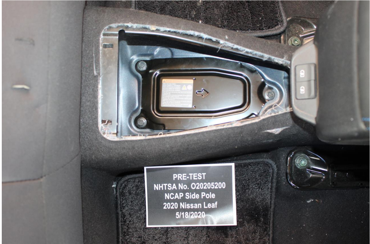
Figure 305-8: Manual High Voltage Service Disconnect Removed Location
