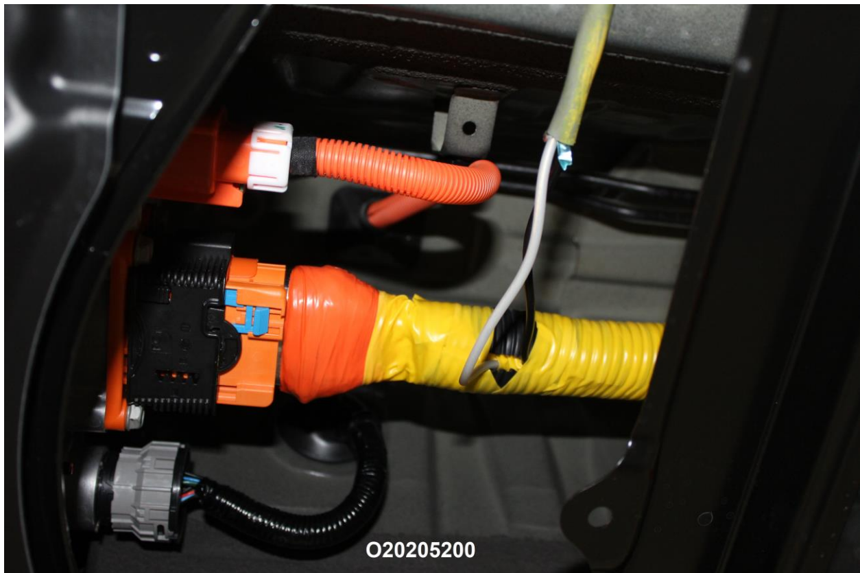
Figure 305-22: Pre-Impact View of High Voltage Leads Attached
