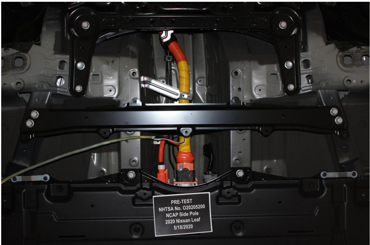
Figure 305-18: Pre-Impact View of High Voltage Interconnects
