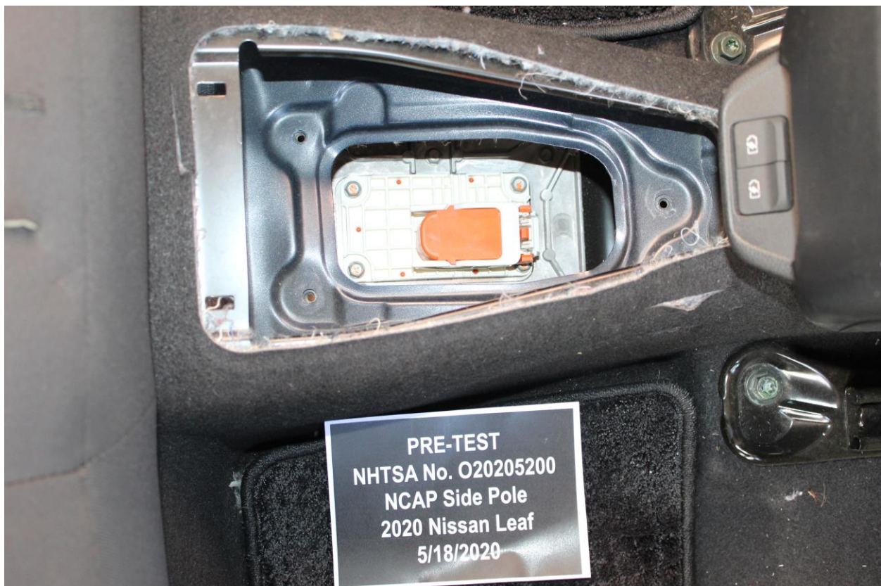
Figure 305-6: Manual High Voltage Service Disconnect in Place
