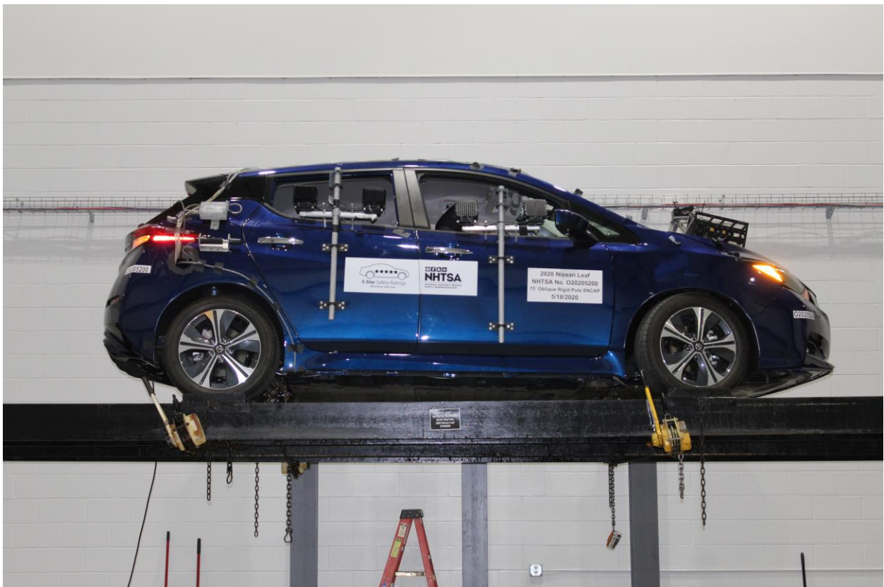
Figure A-67: FMVSS No. 301 Static Rollover 360 Degrees
