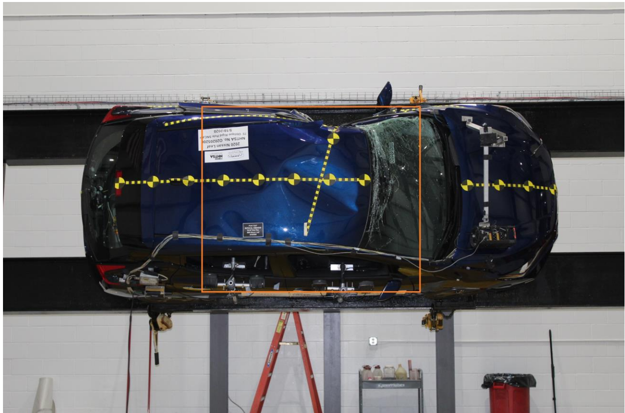
Figure 305-28: FMVSS No. 305 Static Rollover 90 Degrees
