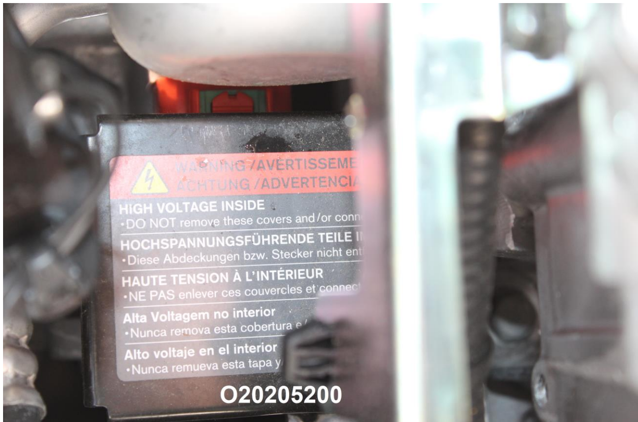
Figure 305-2: Power Inverter Warning Label
