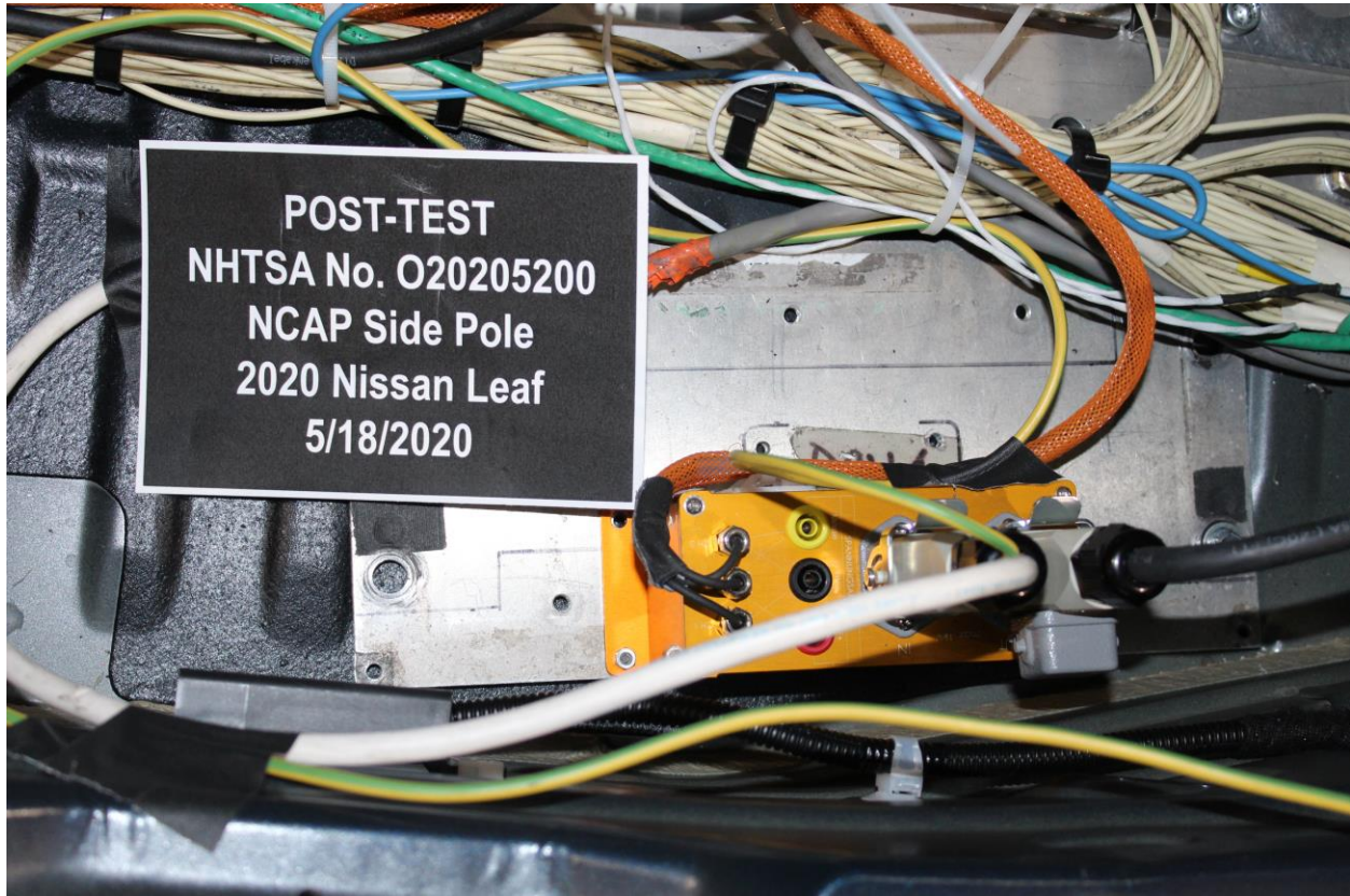
Figure 305-25: Post-Impact View of Installed Test Interface Port
