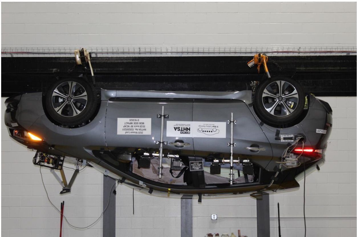
Figure A-98: FMVSS No. 301 Static Rollover 180 Degrees
