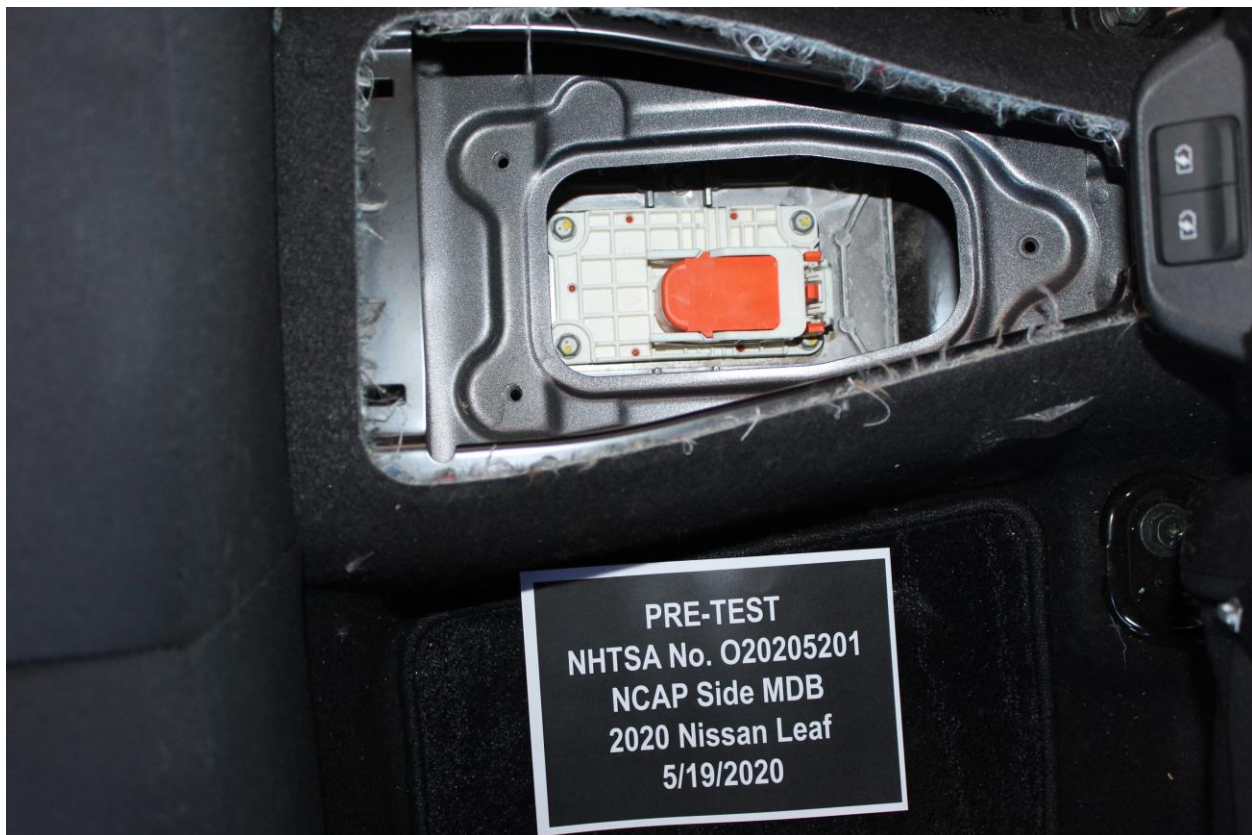
Figure 305-6: Manual High Voltage Service Disconnect in Place
