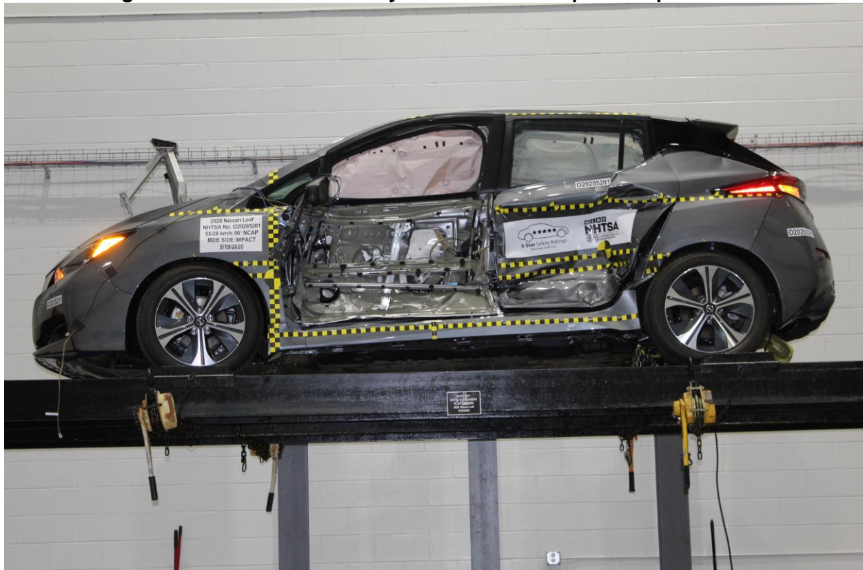
Figure A-96: FMVSS No. 301 Static Rollover 0 Degrees
