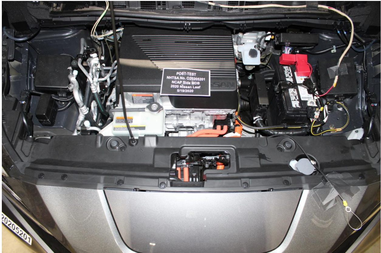
Figure 305-17: Post-Impact View of Electric Propulsion Drive
