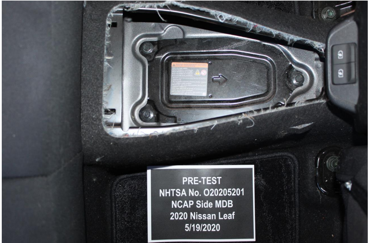
Figure 305-8: Manual High Voltage Service Disconnect Removed Location
