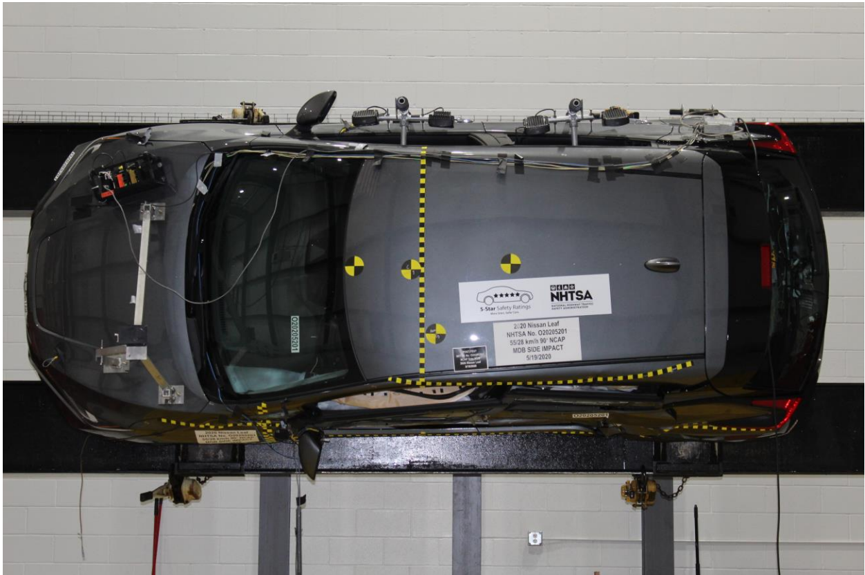
Figure A-99: FMVSS No. 301 Static Rollover 270 Degrees
