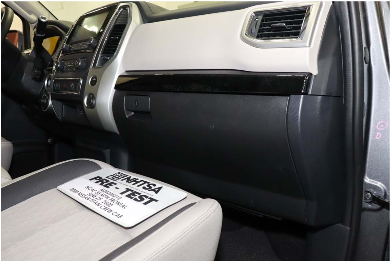
Photo No. 067 - Pre-Test Passenger Side Knee Bolster
