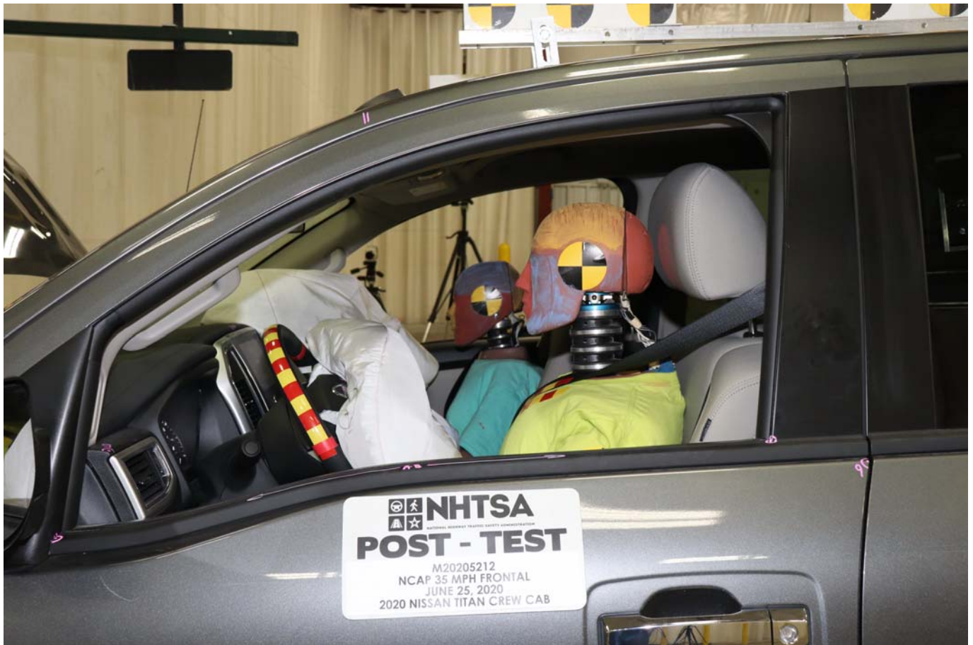
Photo No. 033 - Post-Test Driver Dummy Window View
