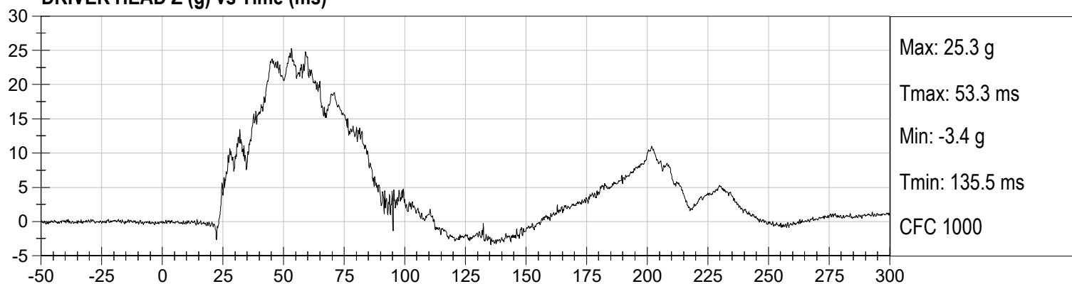
DRIVER HEAD Resultant (g) vs Time (ms)
