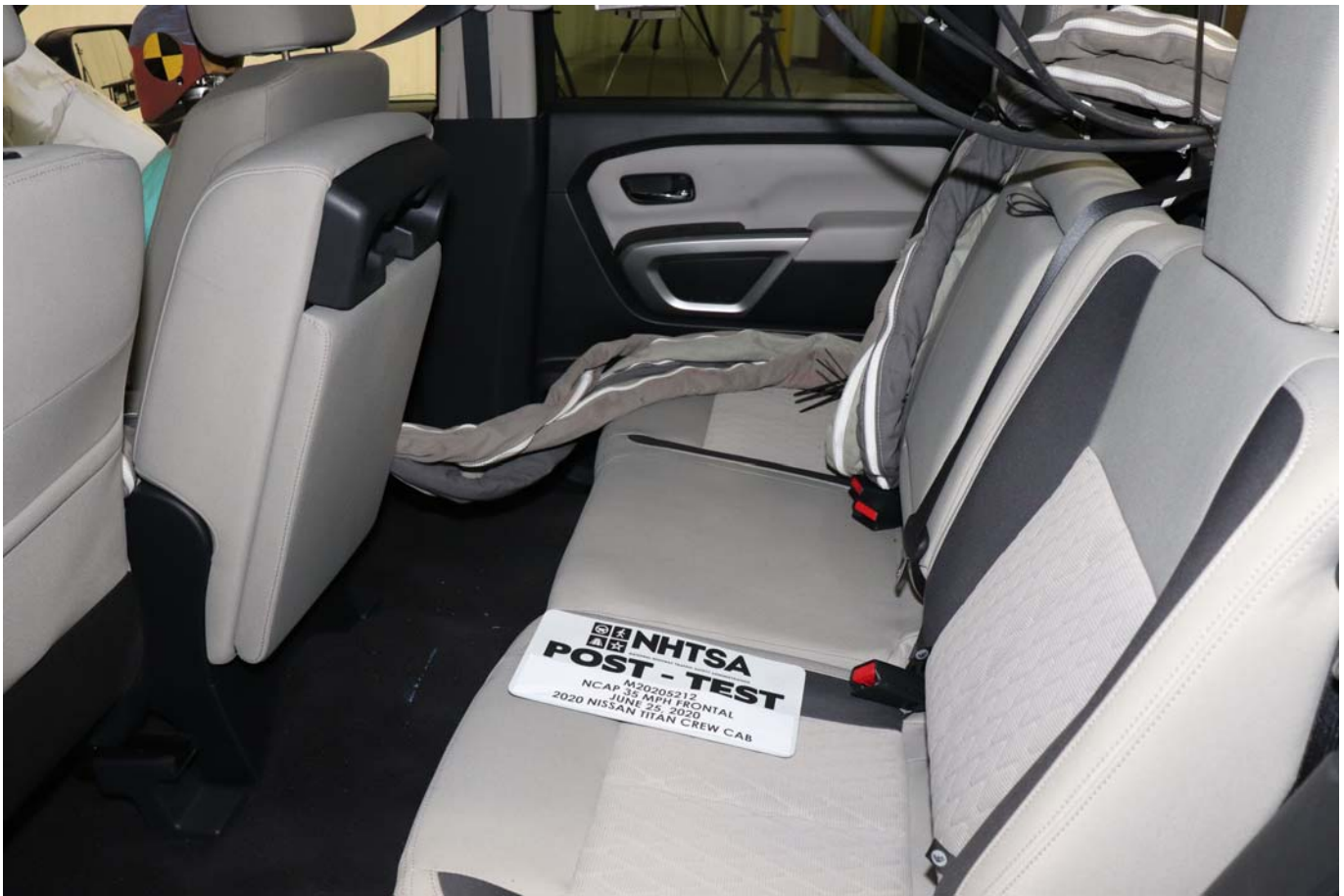
Photo No. 029 - Post-Test Dummy Cable Routing
