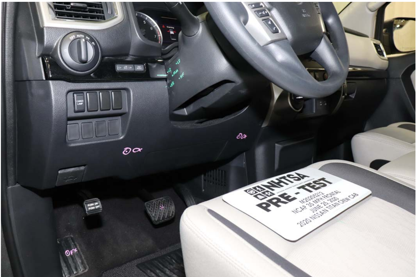
Photo No. 044 - Pre-Test Driver Side Knee Bolster
