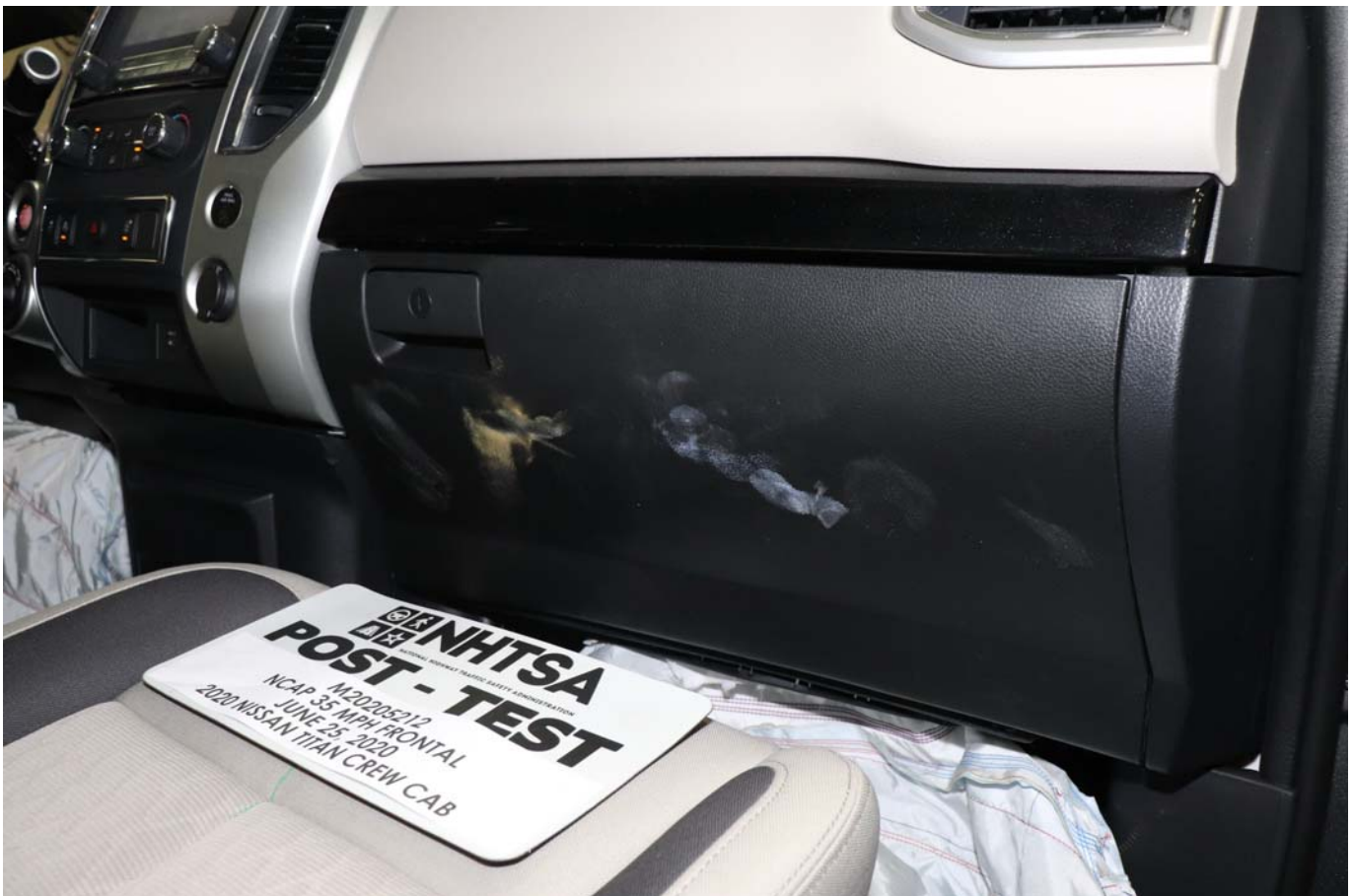
Photo No. 068 - Post-Test Passenger Side Knee Bolster
