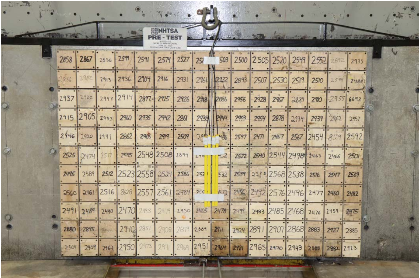
Photo No. 002 - Pre-Test Load Cell Wall
