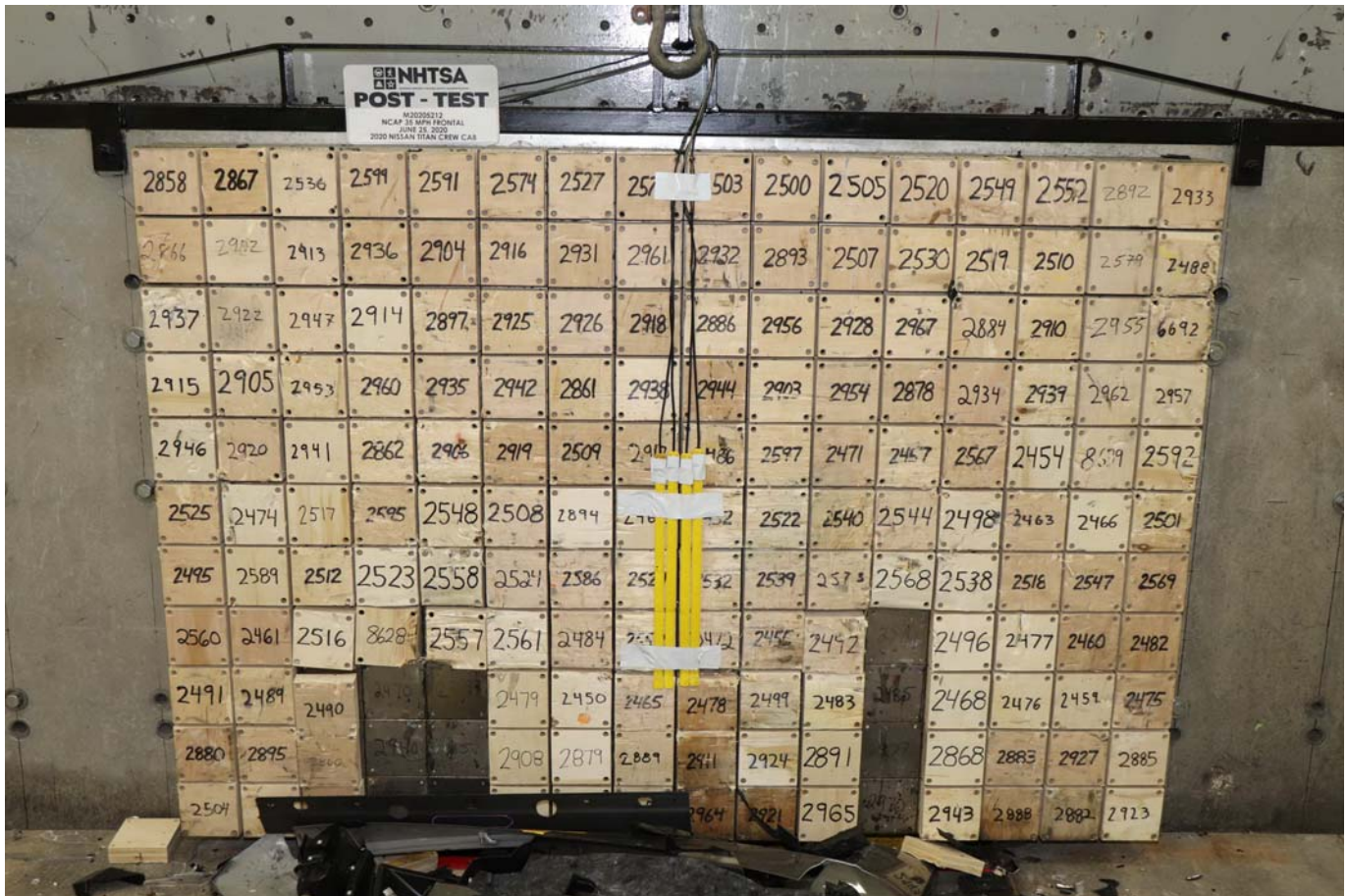
Photo No. 003 - Post-Test Load Cell Wall
