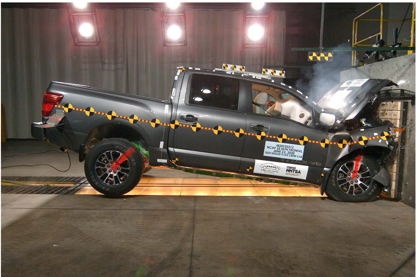
Photo No. 082 - 2020 Nissan Titan SV 4x4 Crew Cab Truck Frontal Impact Event
