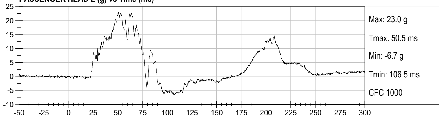
PASSENGER HEAD Resultant (g) vs Time (ms)
