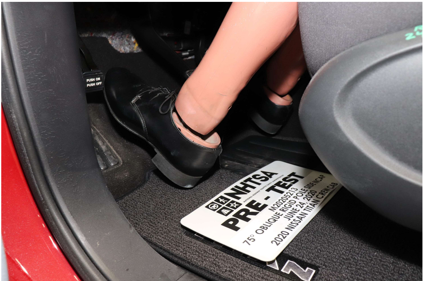
Photo No. 032 - Pre-Test Placement of Dummy Feet
