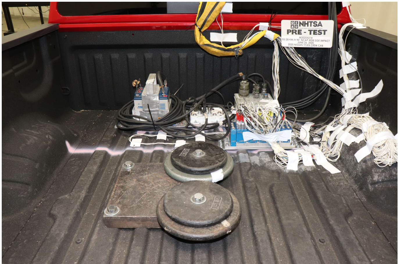
Photo No. 094 - Pre-Test Ballast View
