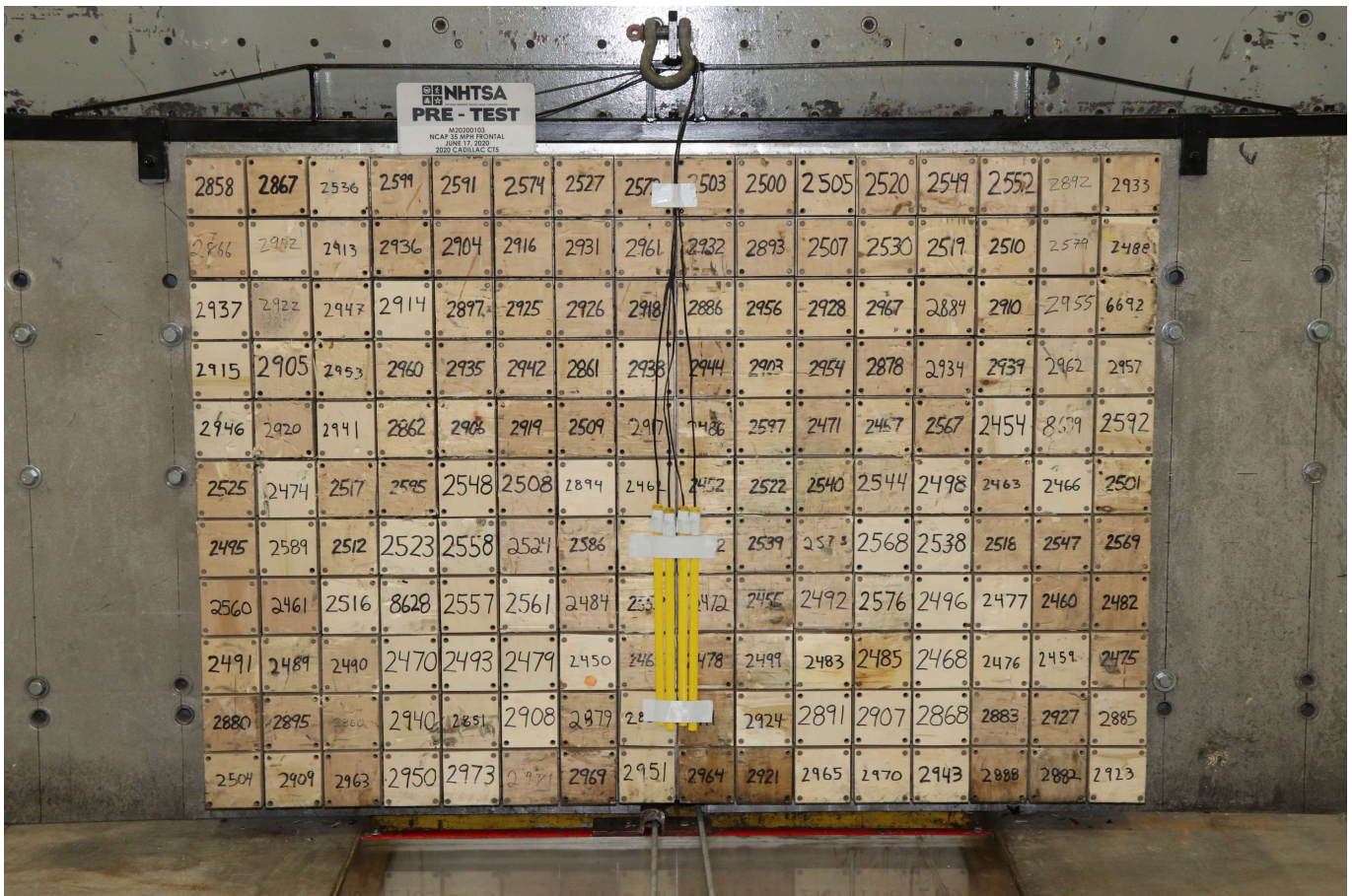
Photo No. 002 - Pre-Test Load Cell Wall
