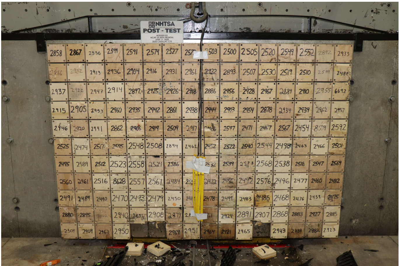
Photo No. 003 - Post-Test Load Cell Wall
