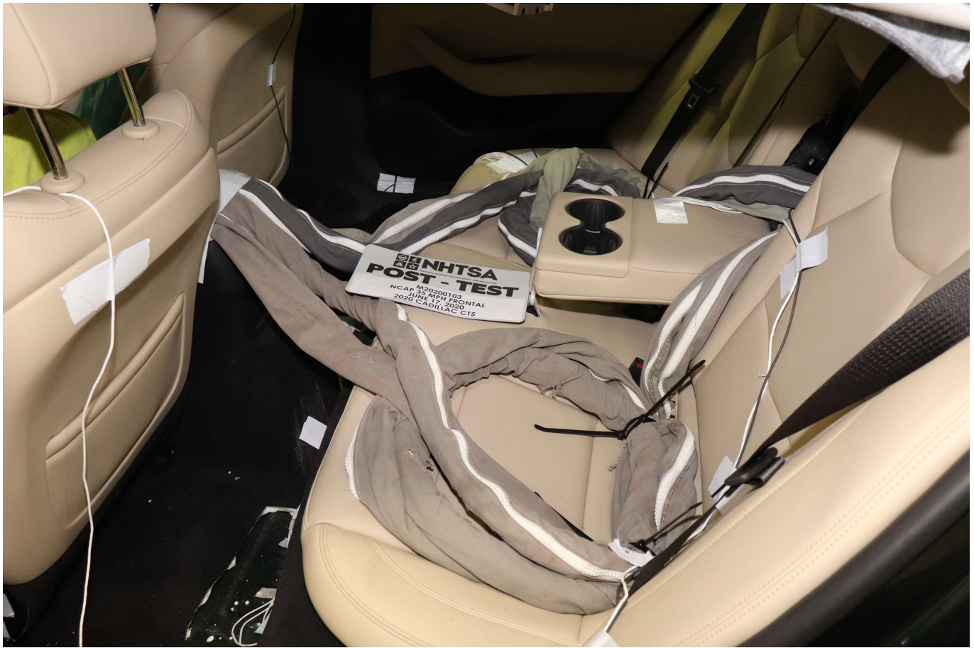
Photo No. 029 - Post-Test Dummy Cable Routing
