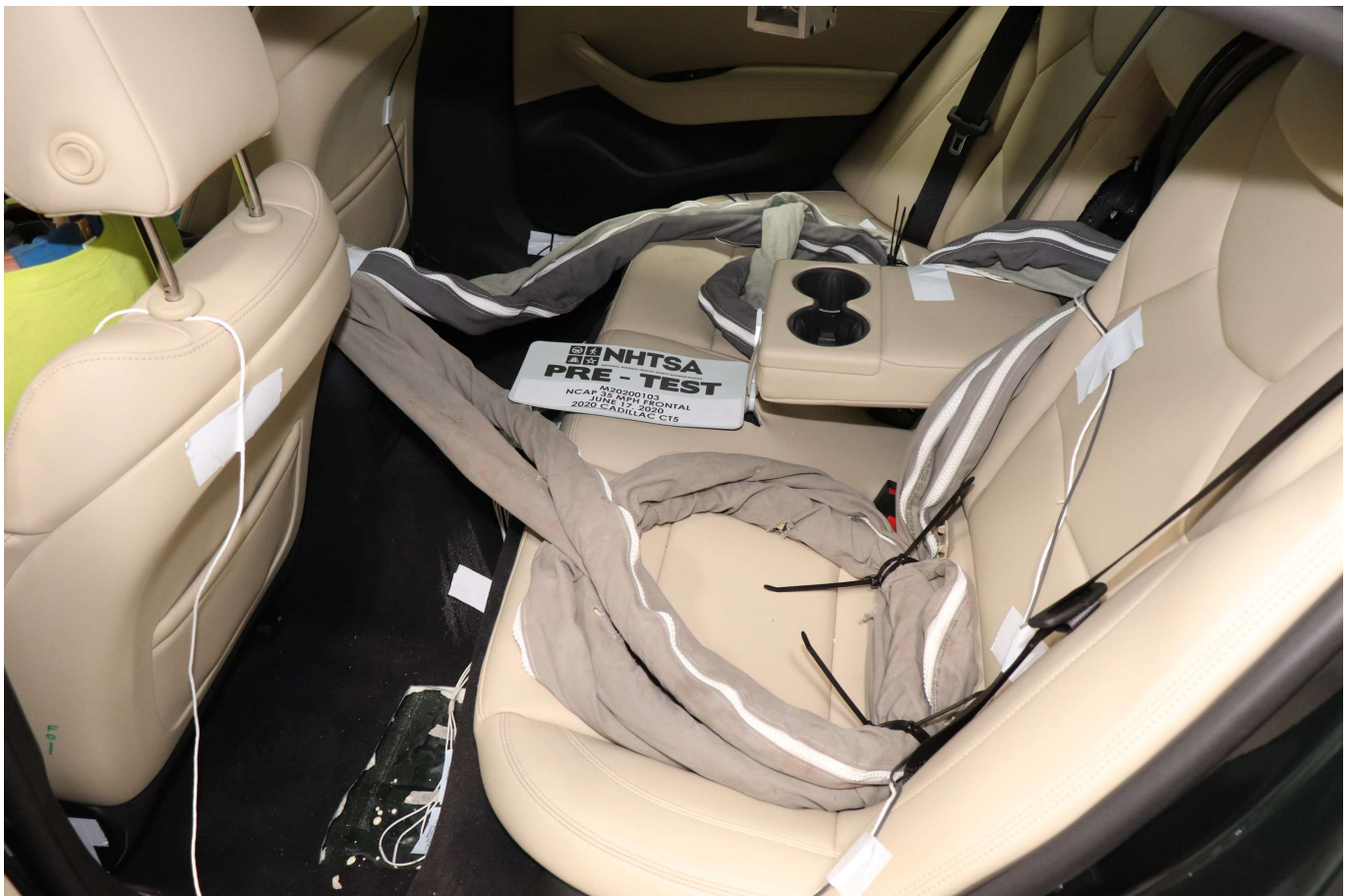
Photo No. 028 - Pre-Test Dummy Cable Routing
