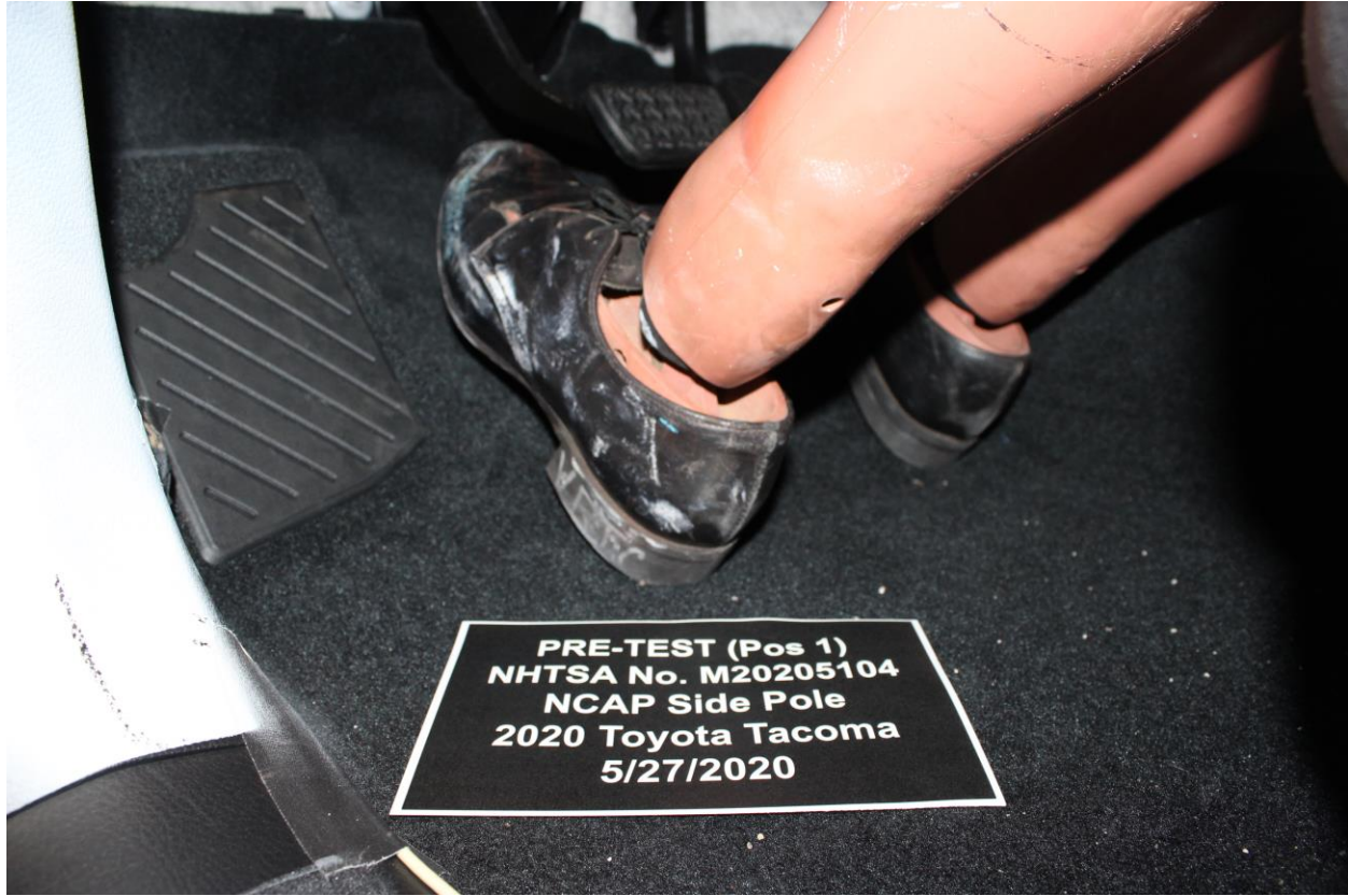
Figure A-32: Pre-Test Placement of Dummy's Feet
