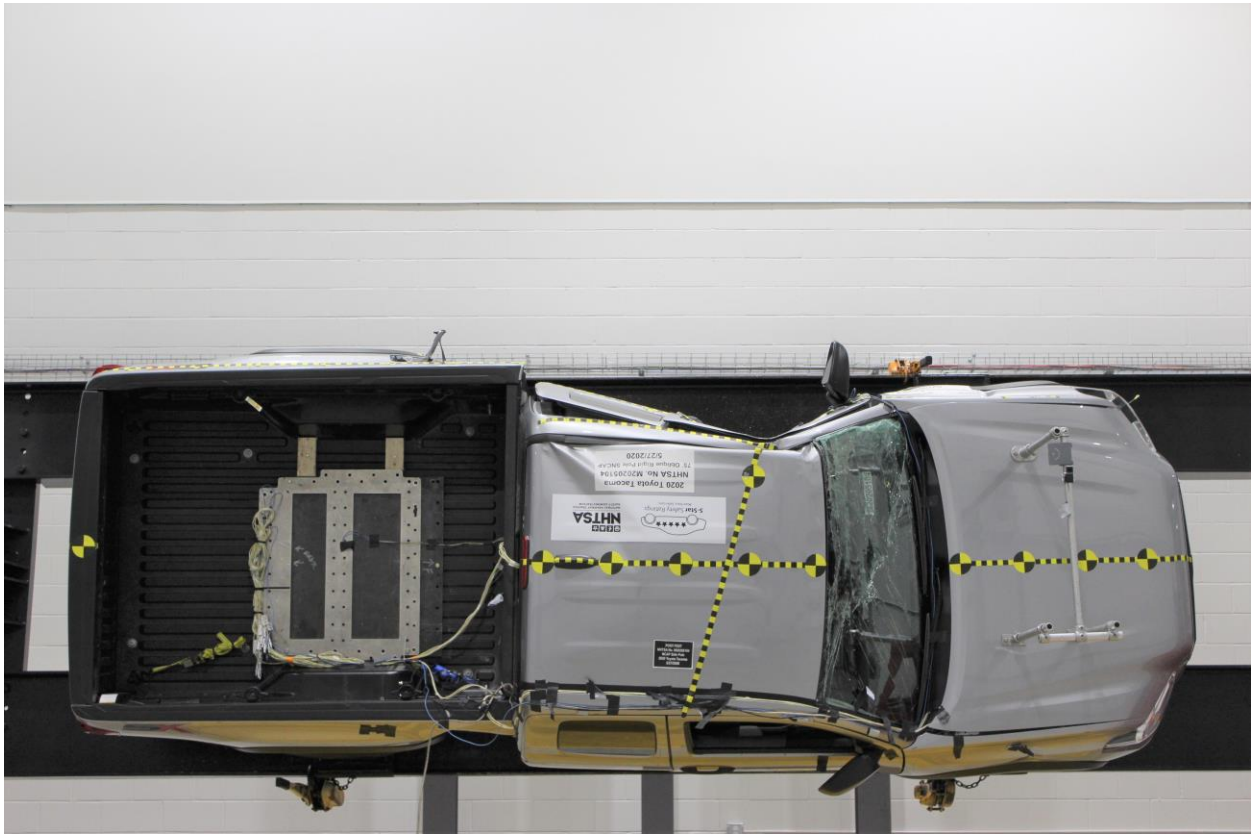
Figure A-66: FMVSS No. 301 Static Rollover 270 Degrees
