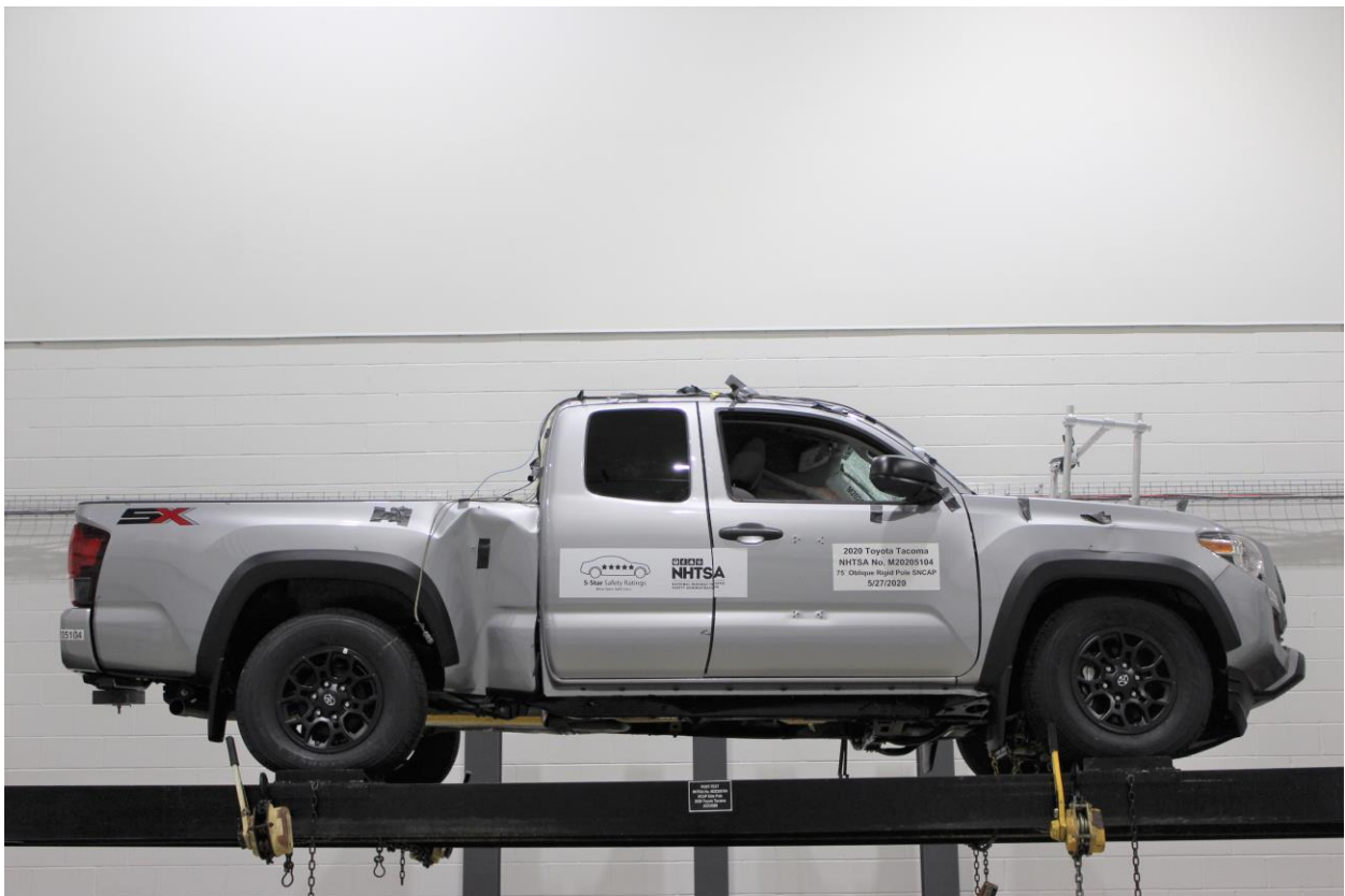
Figure A-67: FMVSS No. 301 Static Rollover 360 Degrees
