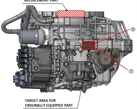
**XVIN** plate for originally equipped part will be attached to either ① or ②.
