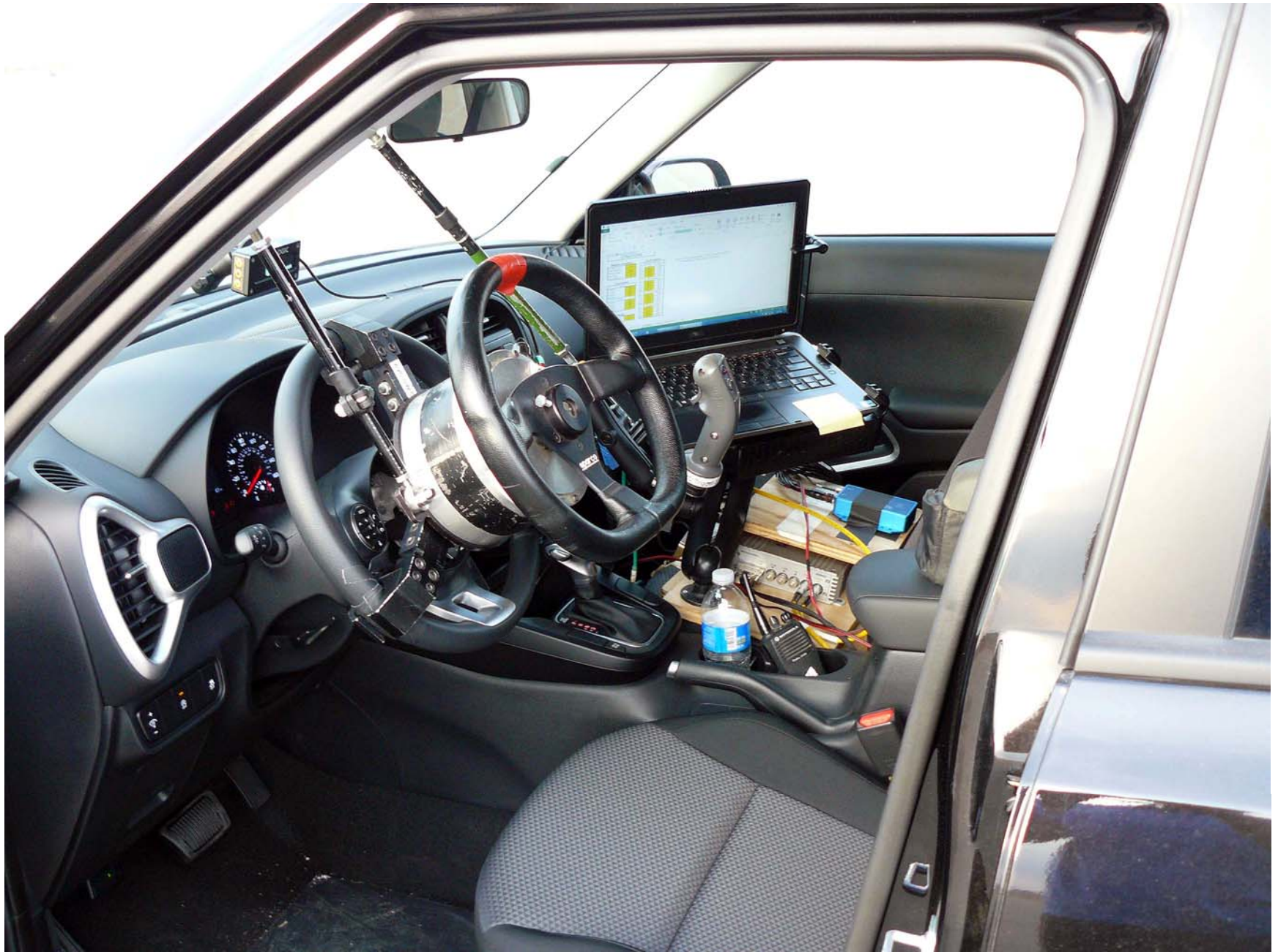
Figure A9. Steering Controller and Computer
