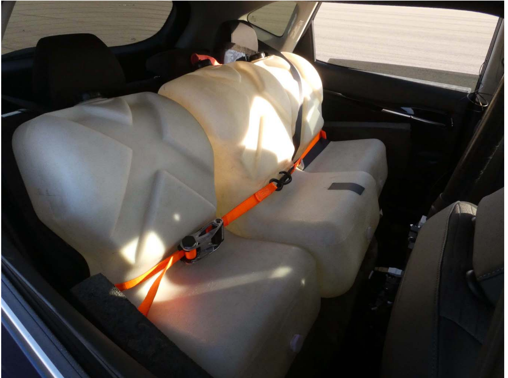
Figure A10. Ballast Condition
