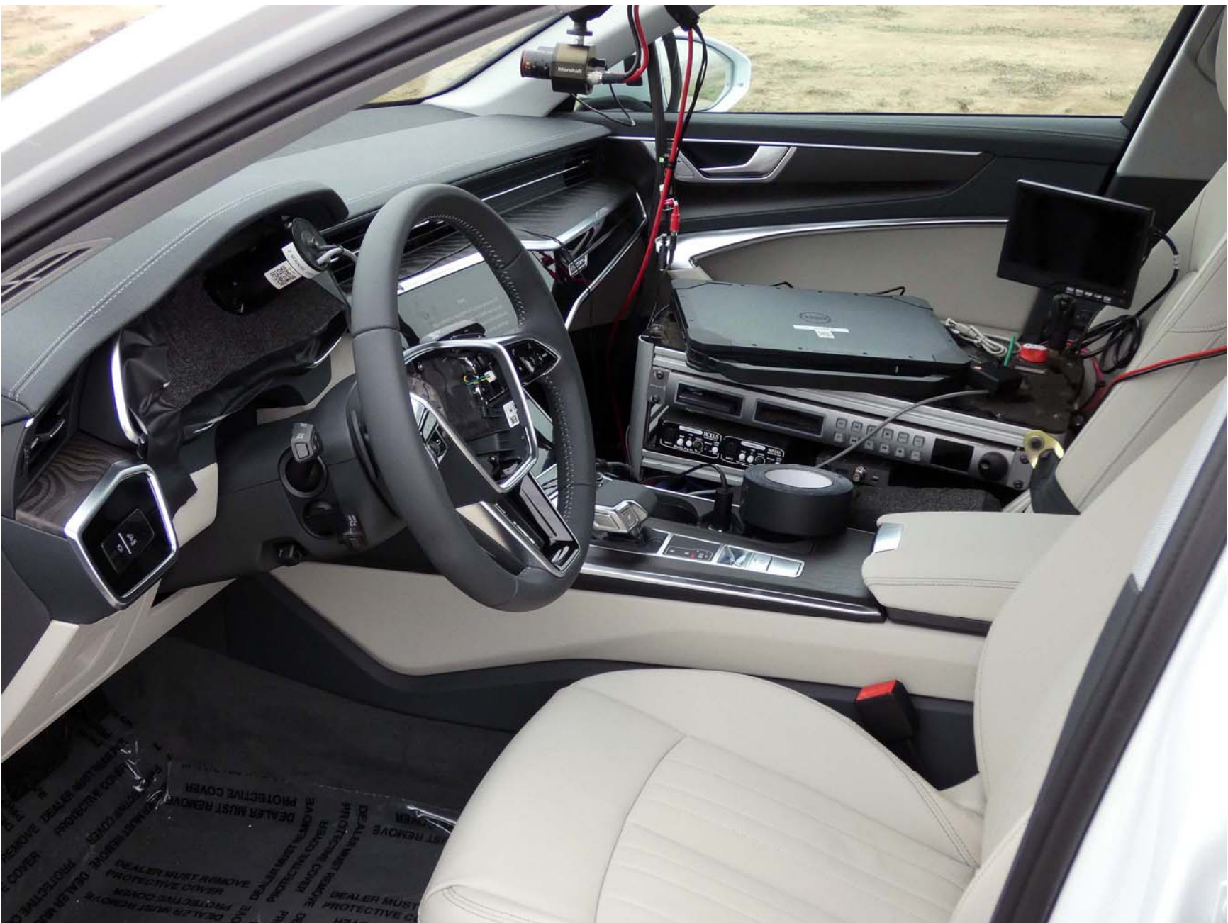
Figure A11. Computer Installed in Subject Vehicle
