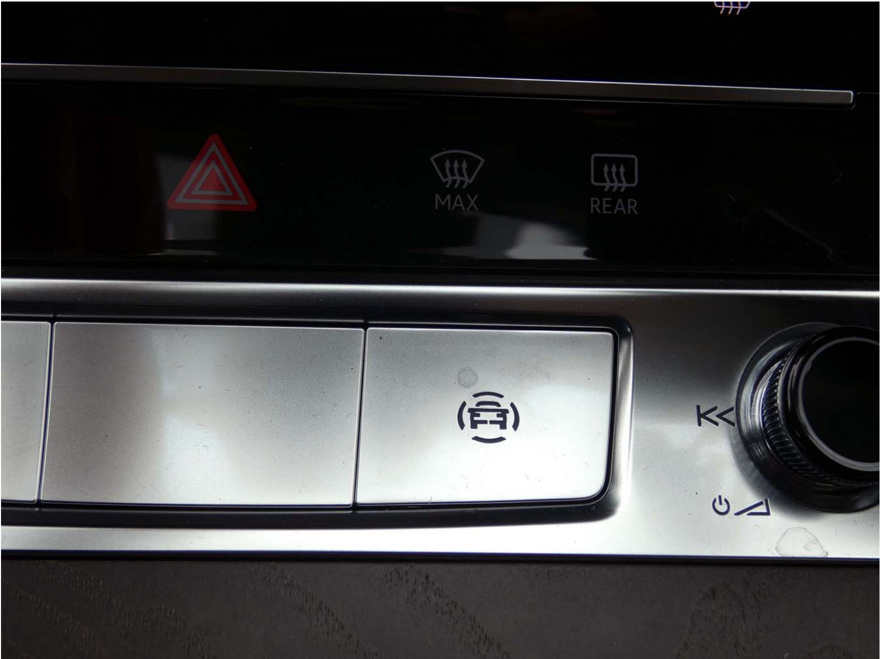
Figure A15. Button for Directly Accessing Driver Assistance Settings Menus
