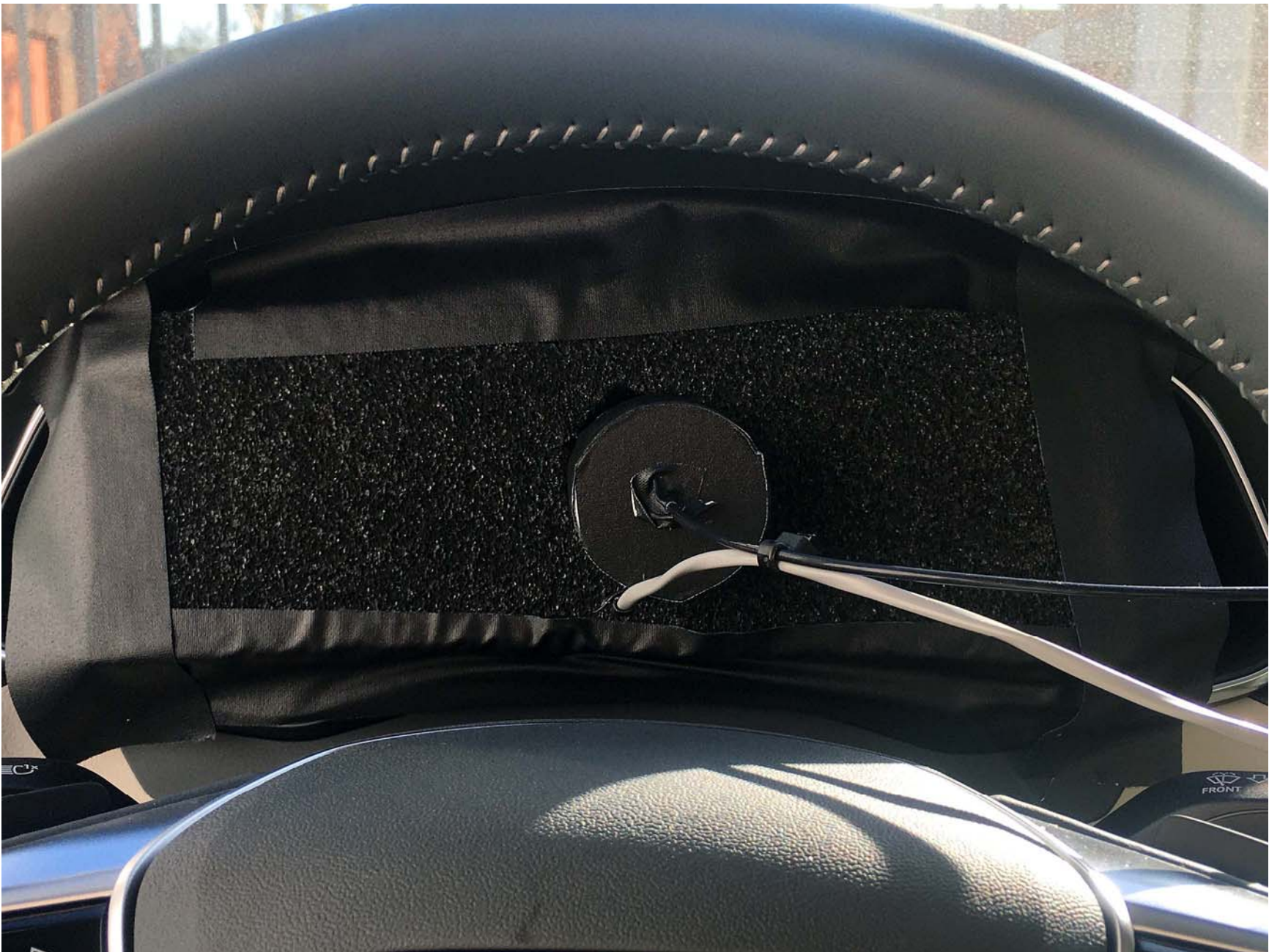
Figure A9. Sensor for Detecting Visual Alerts
