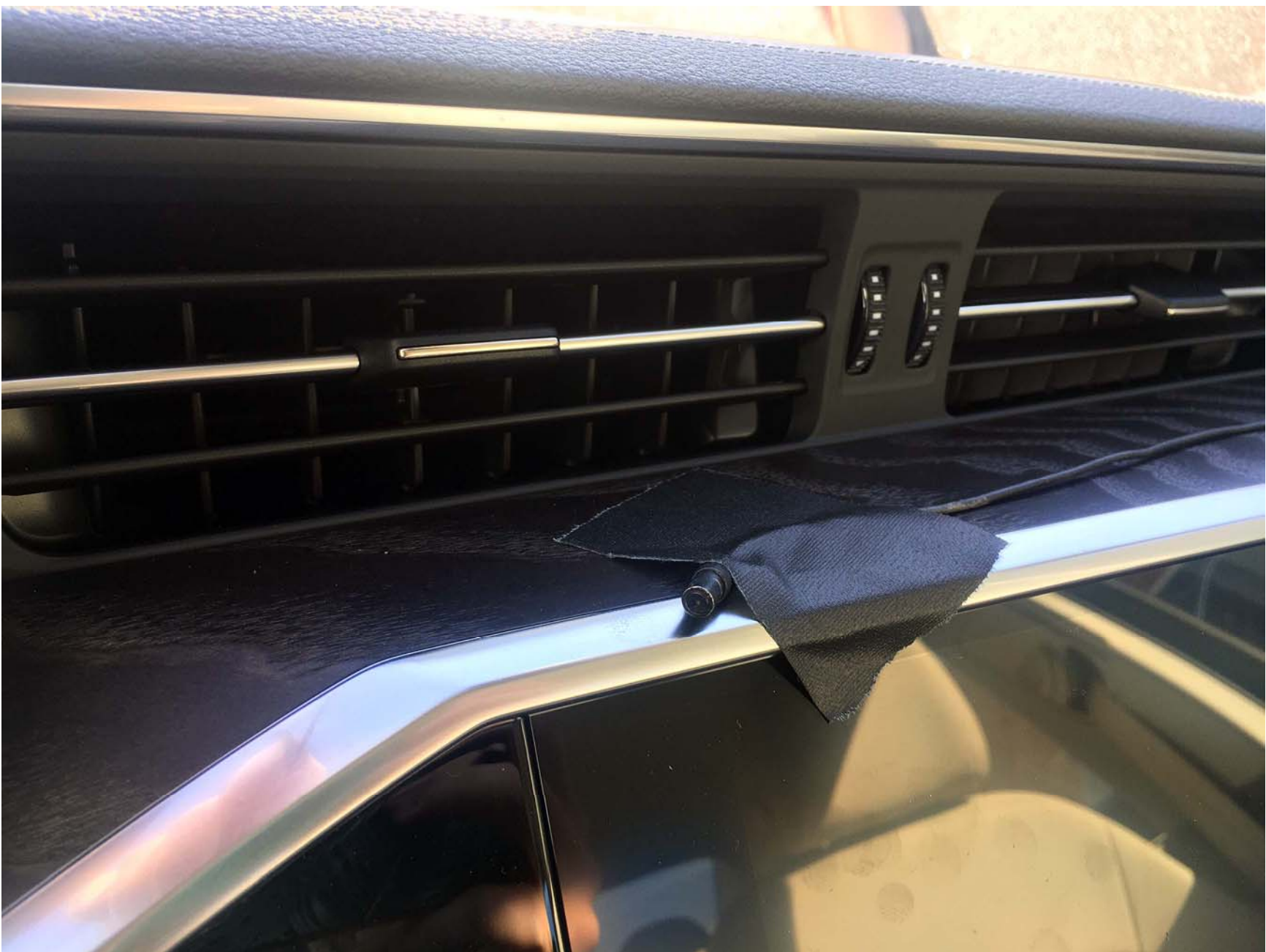
Figure A10. Sensor for Detecting Auditory Alerts
