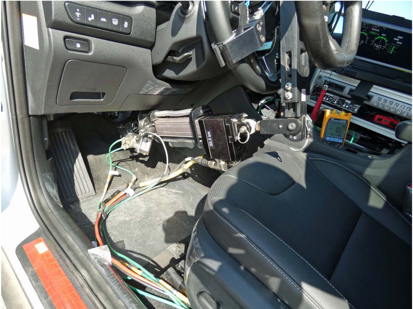
Figure A14. Brake Actuator Installed in Subject System
