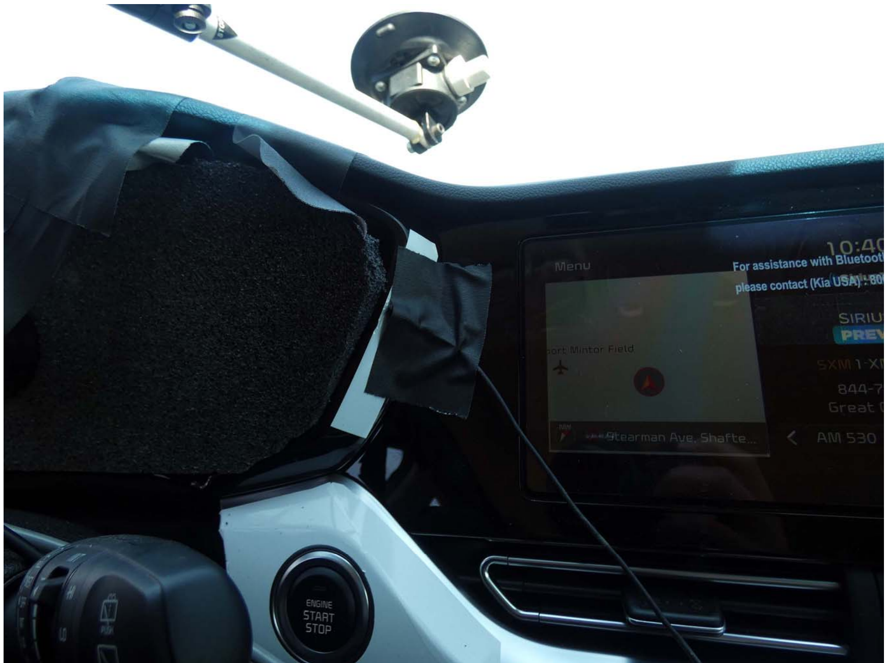
Figure A11. Sensor for Detecting Auditory Alerts
