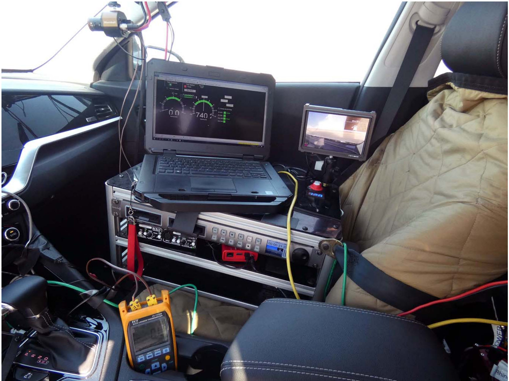
Figure A13. Computer Installed in Subject Vehicle
