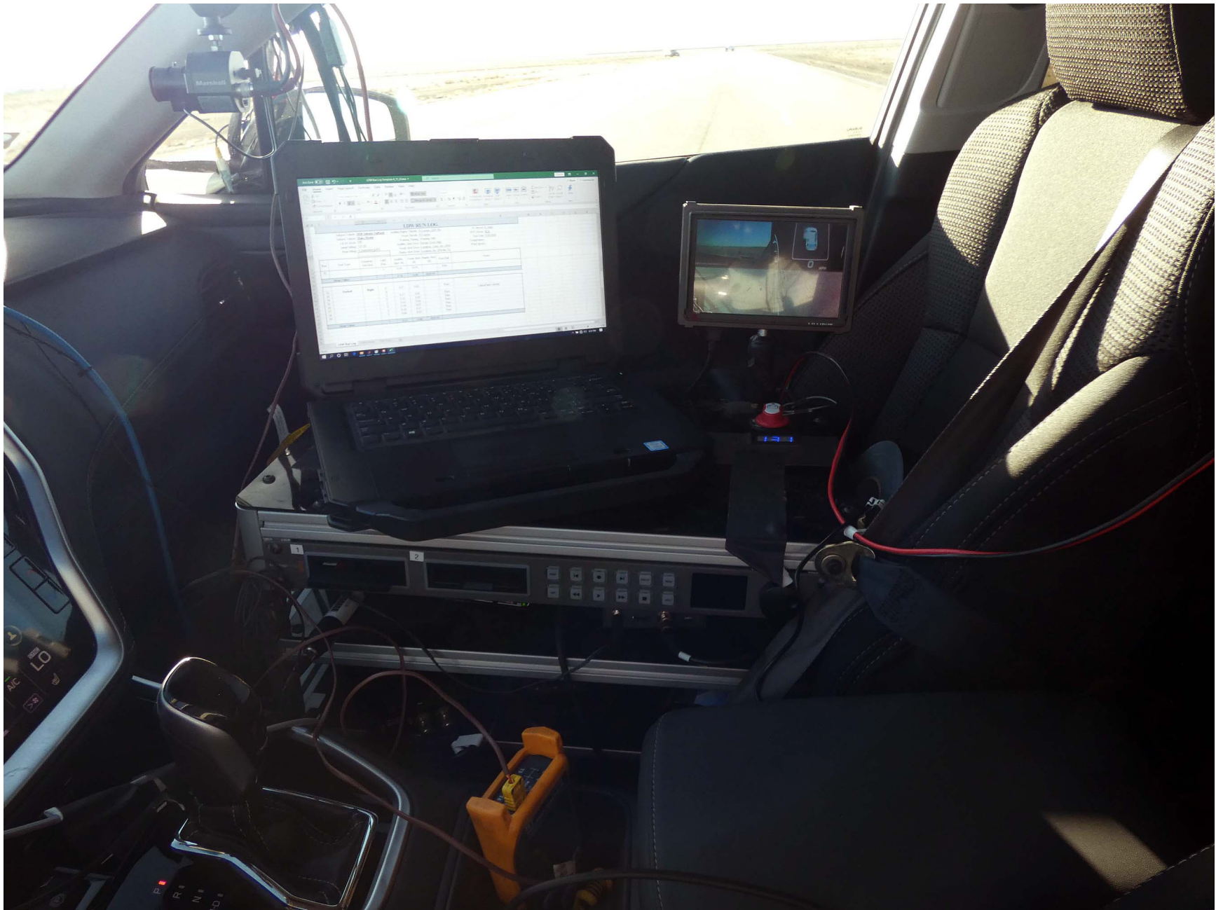
Figure A13. Computer Installed in Subject Vehicle
