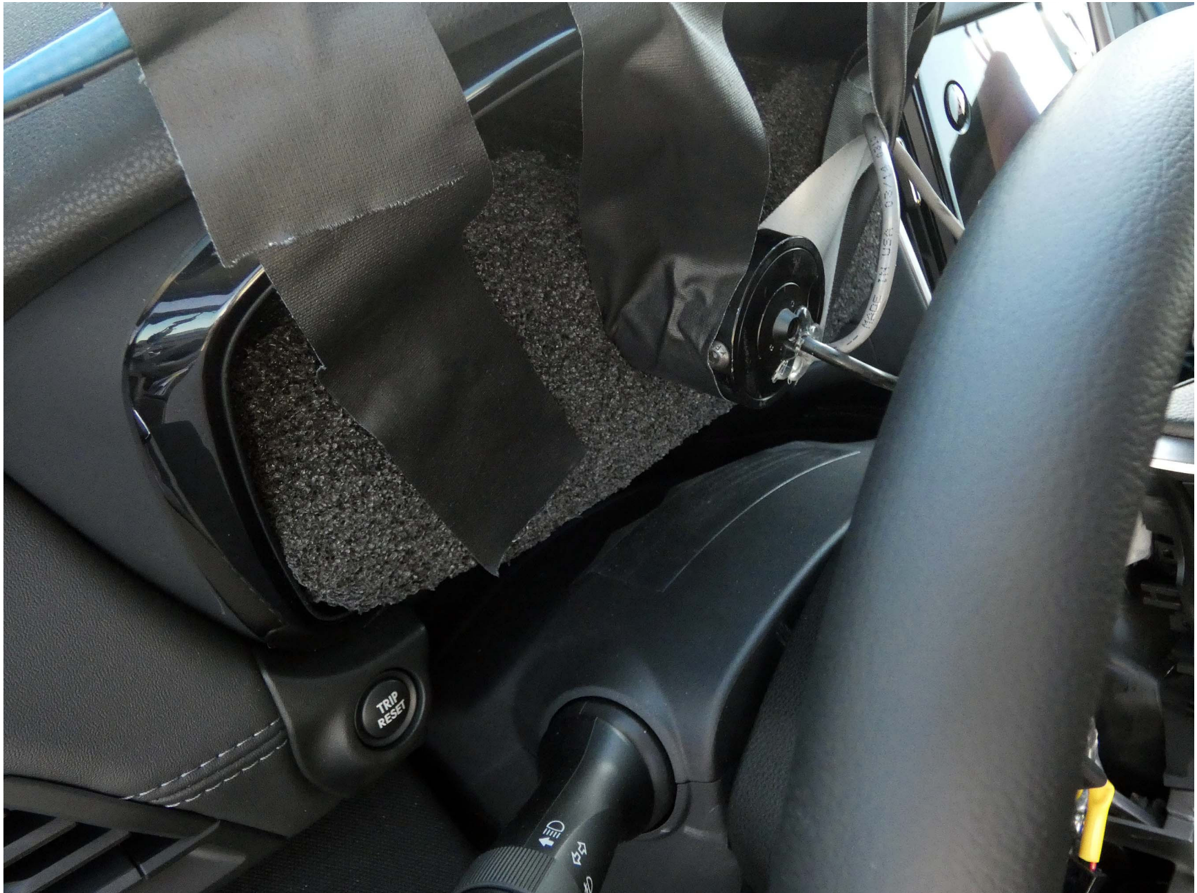
Figure A12. Sensor for Detecting Visual Alerts
