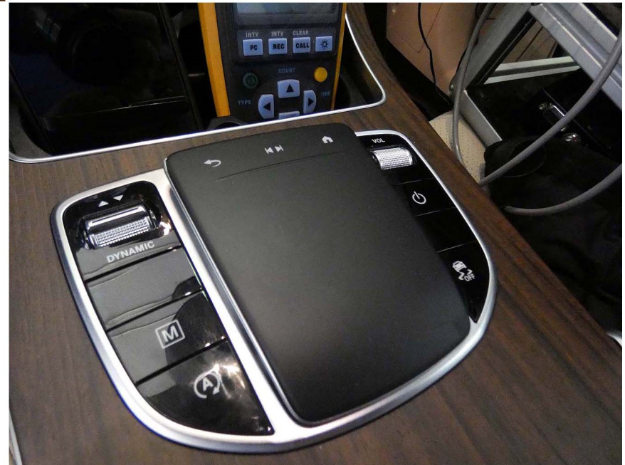
Figure A13. Controls for Changing System Parameters
