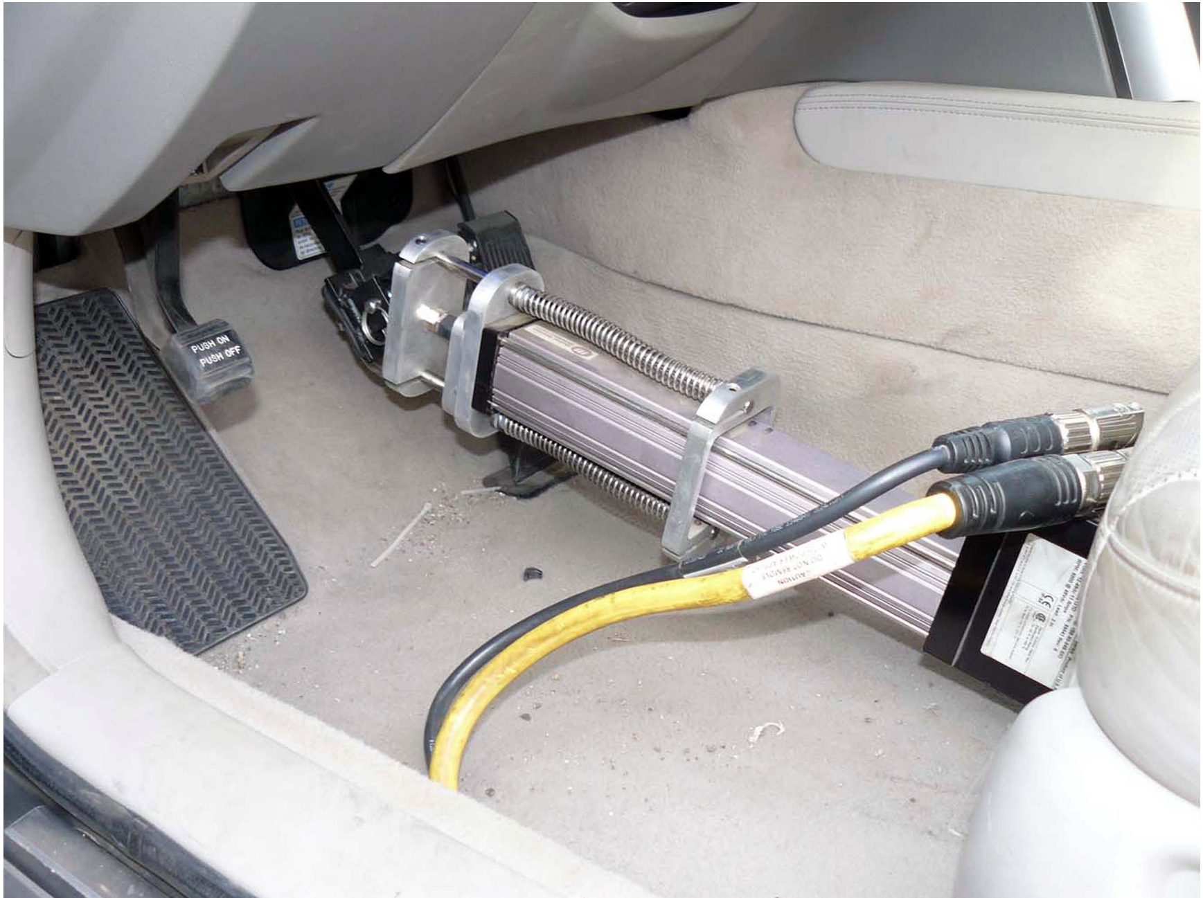
Figure A11. Brake Actuation System Installed in Principal Other Vehicle
