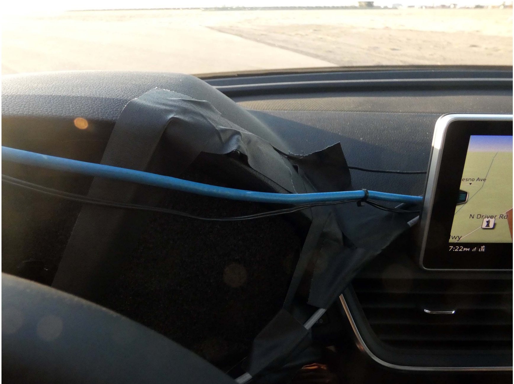
Figure A9. Sensor for Detecting Auditory Alerts
