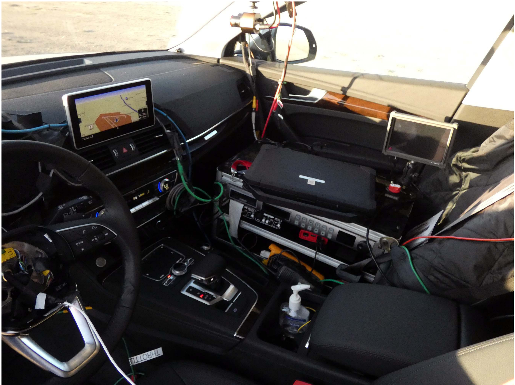
Figure A11. Computer Installed in Subject Vehicle
