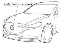
If "Front Radar Sensor Blocked" is displayed in the multi-information display of the instrument cluster, clean the area around the radar sensor (front).
