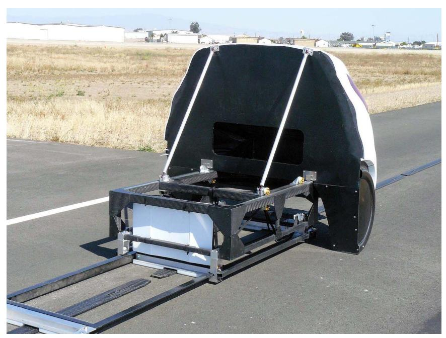
Figure A7. Load Frame/Slider of SSV
