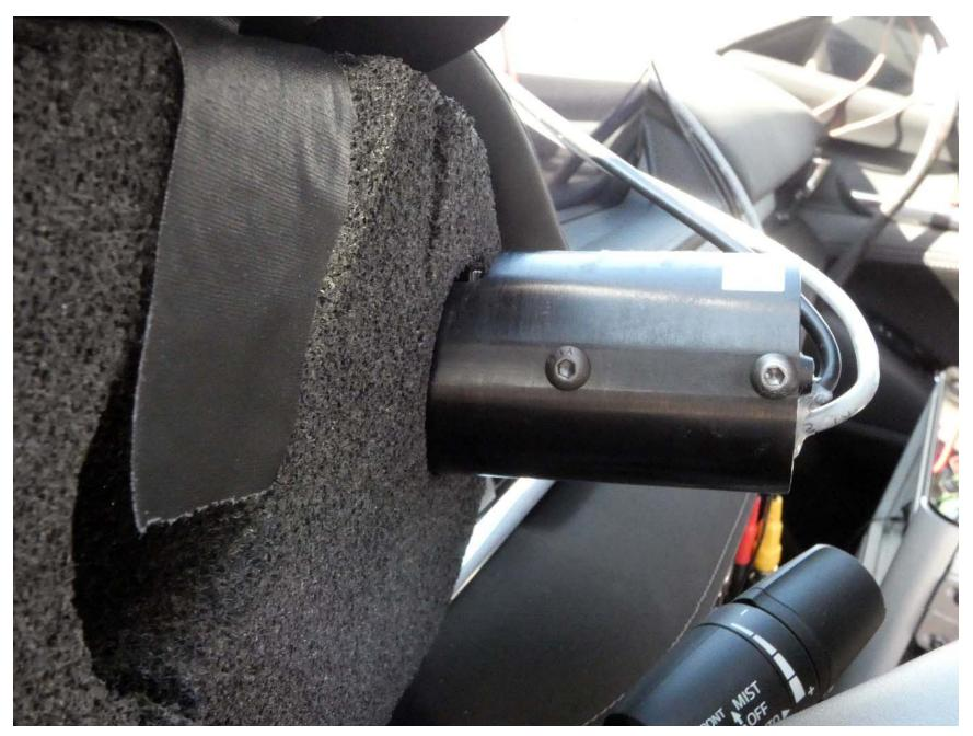
Figure A12. Sensor for Detecting Visual Alerts
