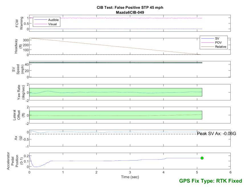
Figure D48. Time History for CIB Run 49, SV Encounters Steel Trench Plate, SV 45 mph
