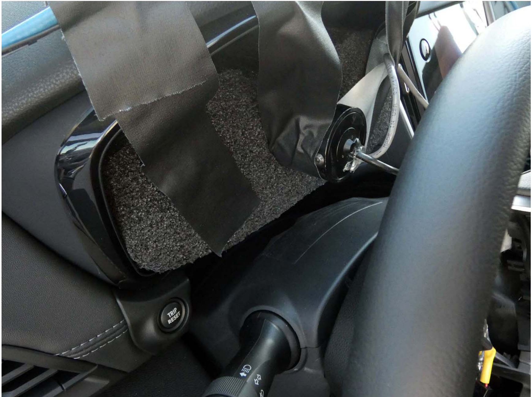
Figure A12. Sensor for Detecting Visual Alerts
