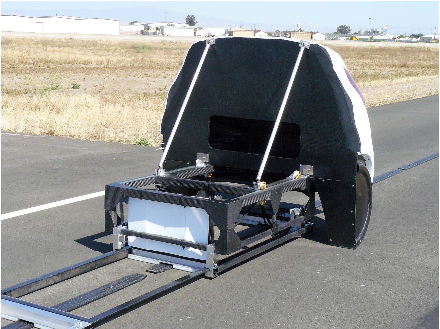
Figure A7. Load Frame/Slider of SSV
