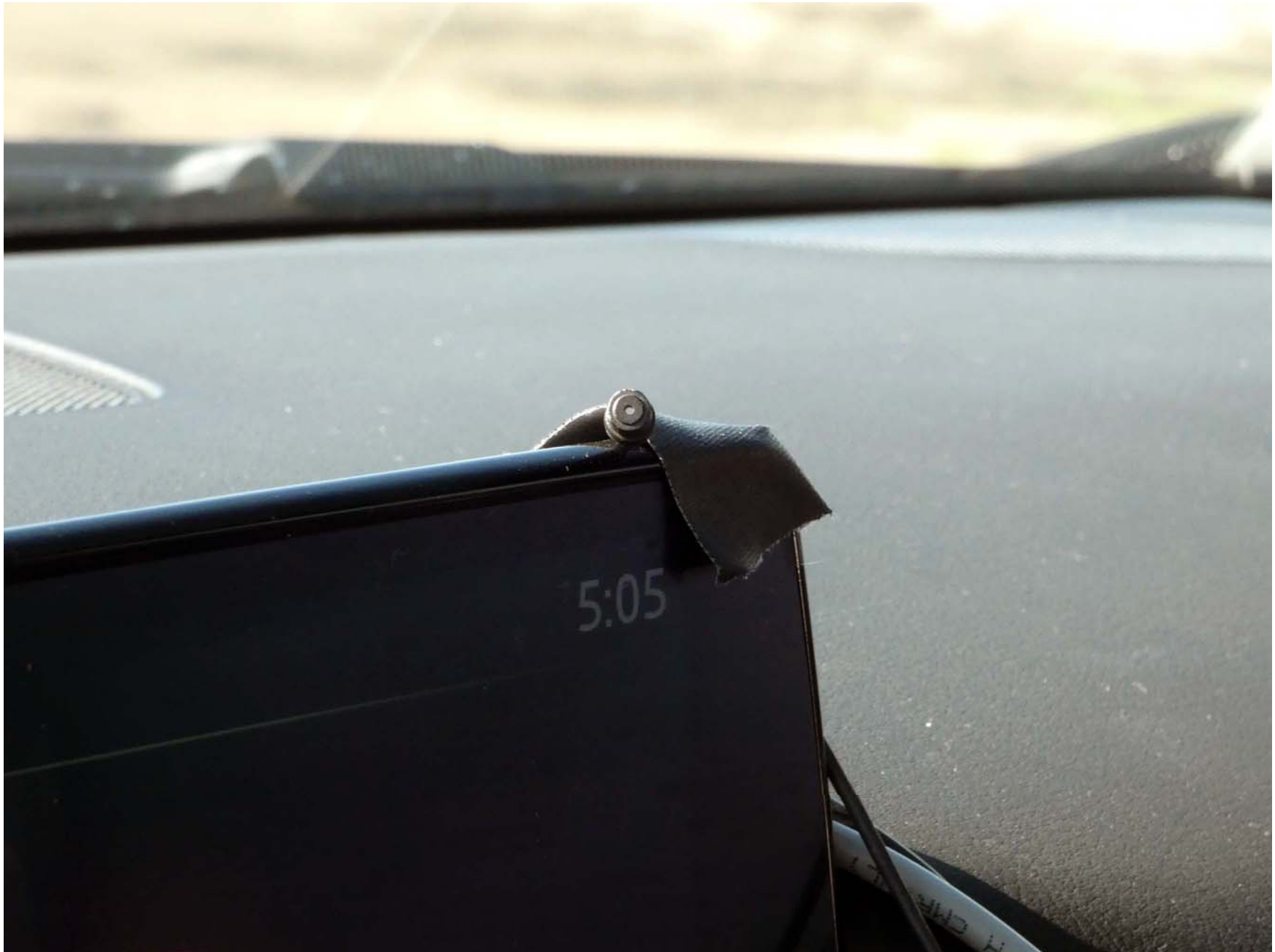
Figure A11. Sensor for Detecting Auditory Alerts
