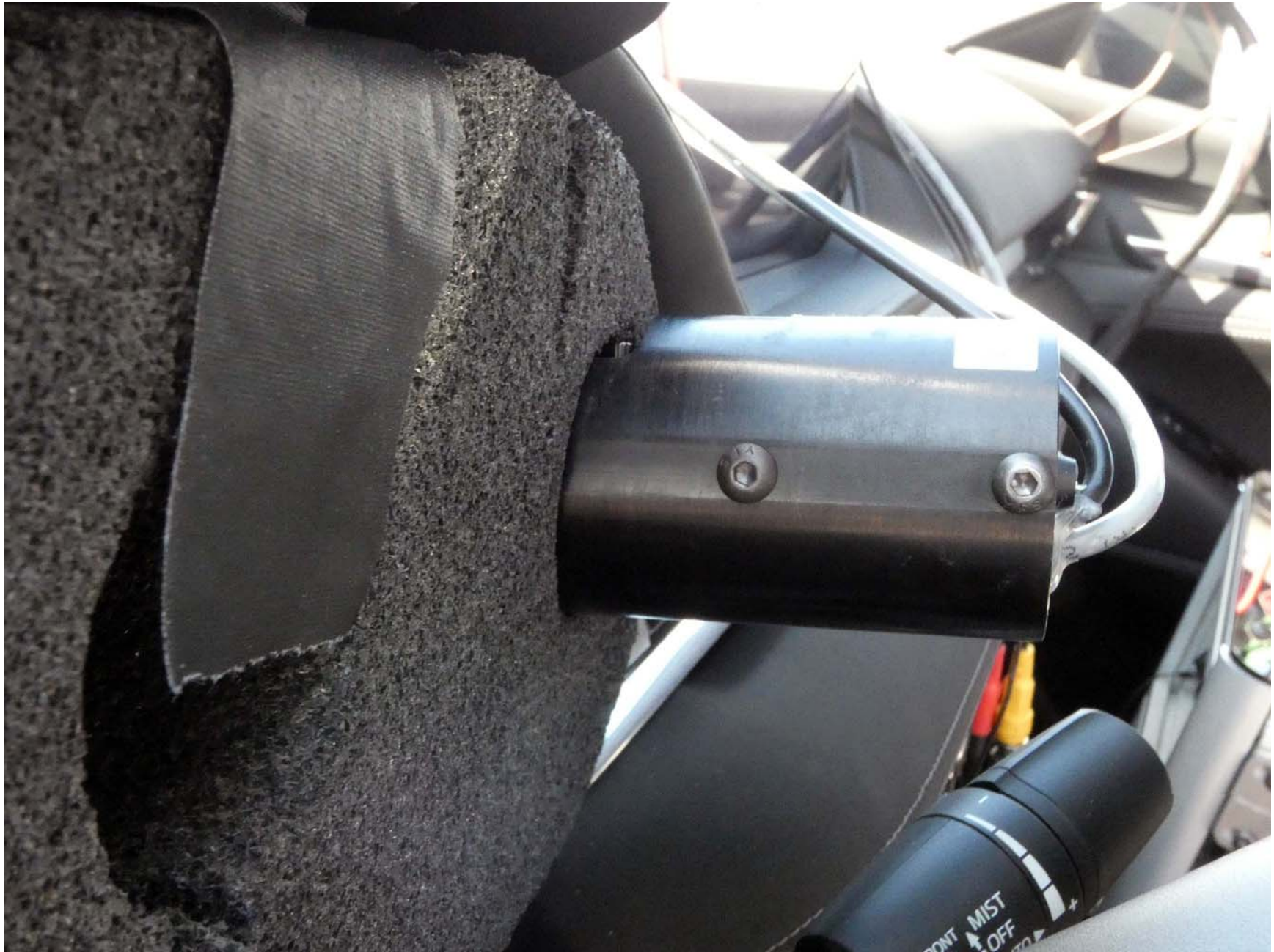
Figure A12. Sensor for Detecting Visual Alerts
