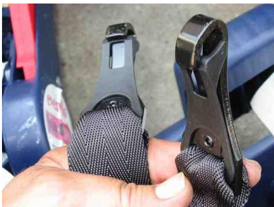
LATCH Lower anchor attachments
