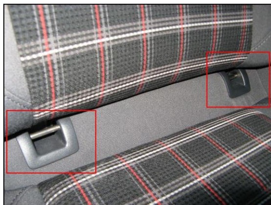
Lower seat anchorage points within vehicle
