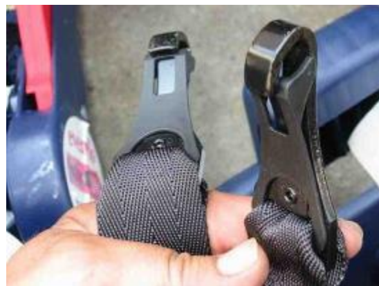
LATCH Lower anchor attachments
