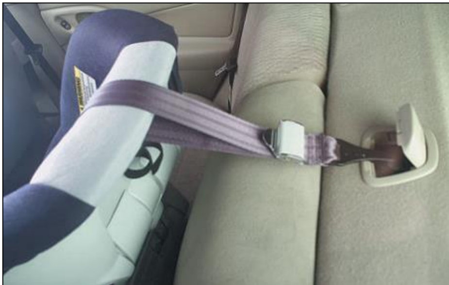
LATCH system top tether attached
