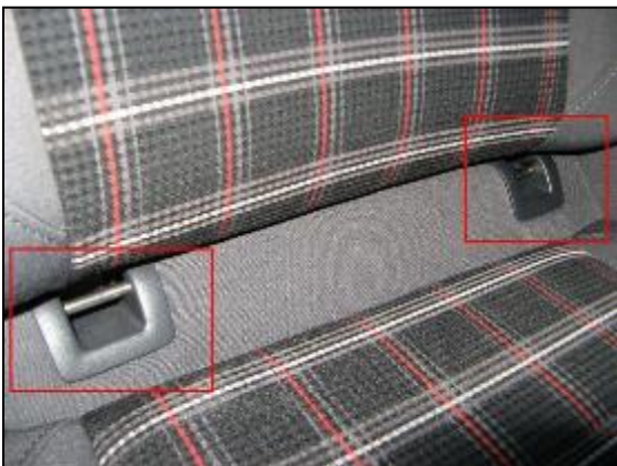
Lower seat anchorage points within vehicle
