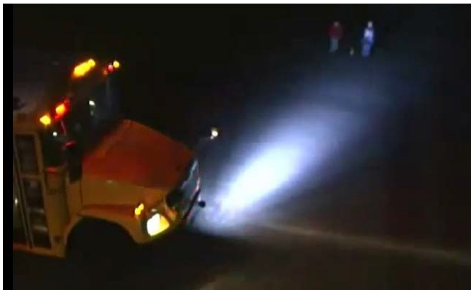
Figure 6: Photograph of the Gardian Angel bus lighting system in operation (Photo provided by Gardian Angel LLC)
