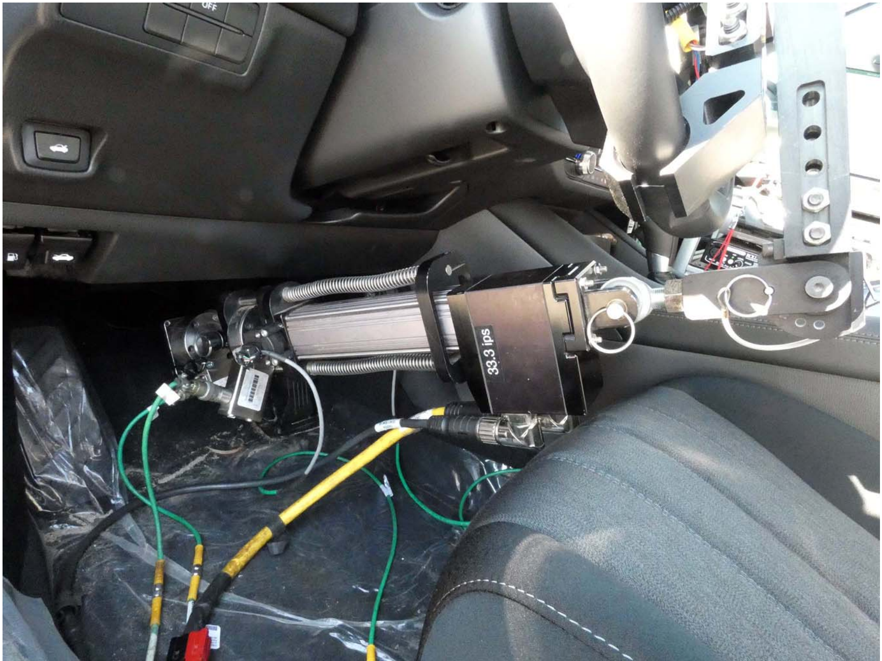
Figure A15. Brake Actuator Installed in POV System A-17
