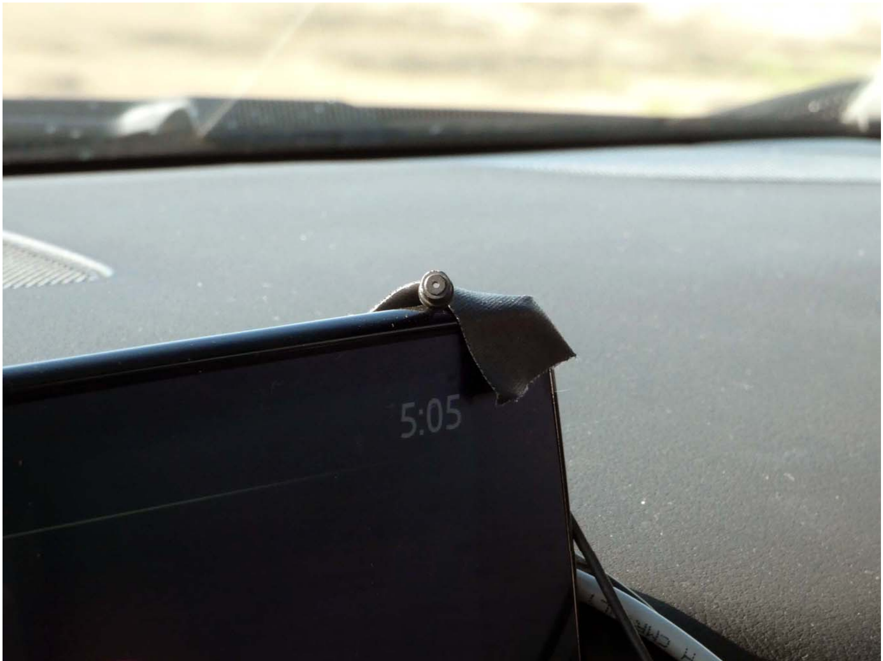
Figure A11. Sensor for Detecting Auditory Alerts
