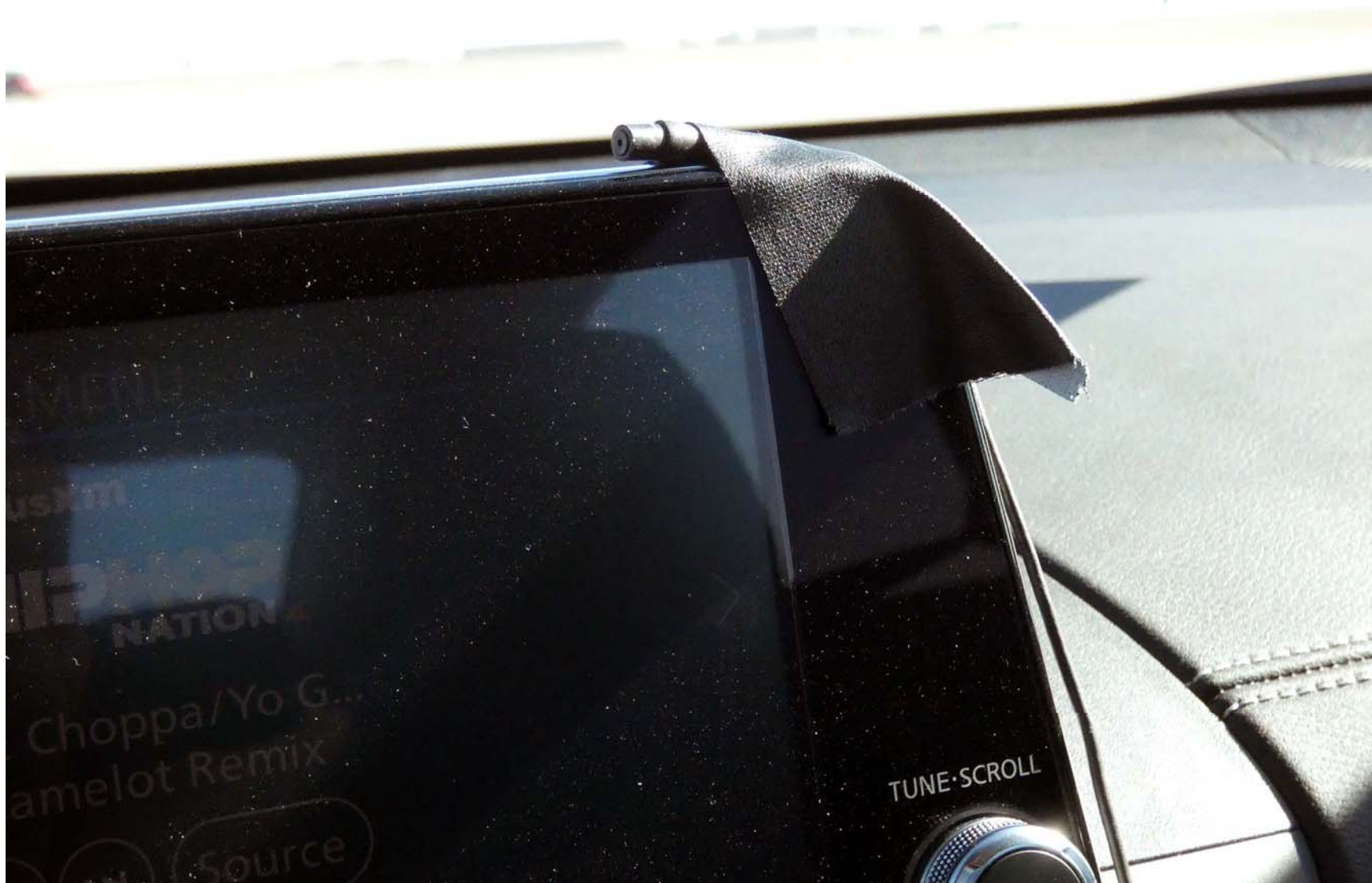
Figure A12. Sensor for Detecting Auditory Alerts
