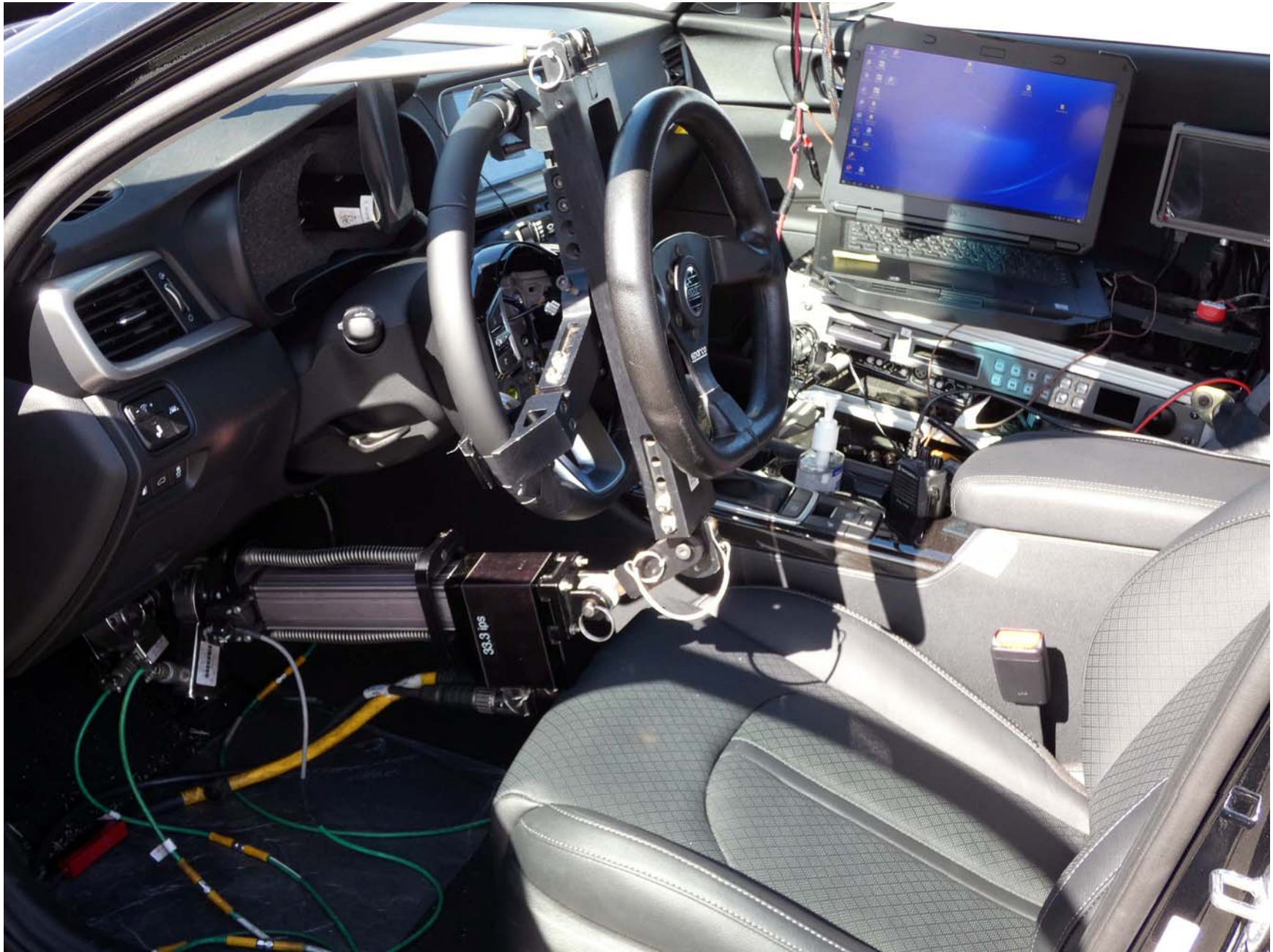
Figure A13. Computer and Brake Actuator Installed in Subject Vehicle
