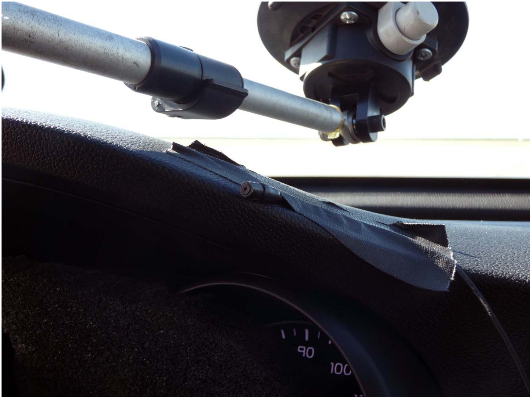
Figure A11. Sensor for Detecting Auditory Alerts
