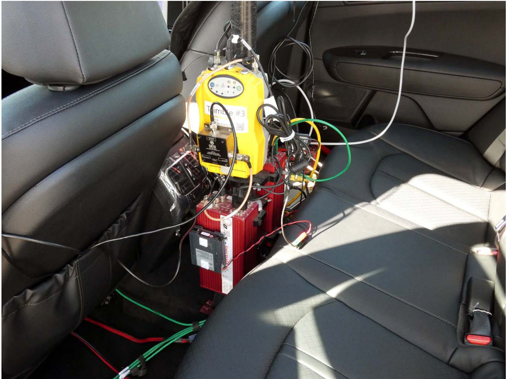
Figure A10. DGPS, Inertial Measurement Unit, and MicroAutoBox Installed in Subject Vehicle
