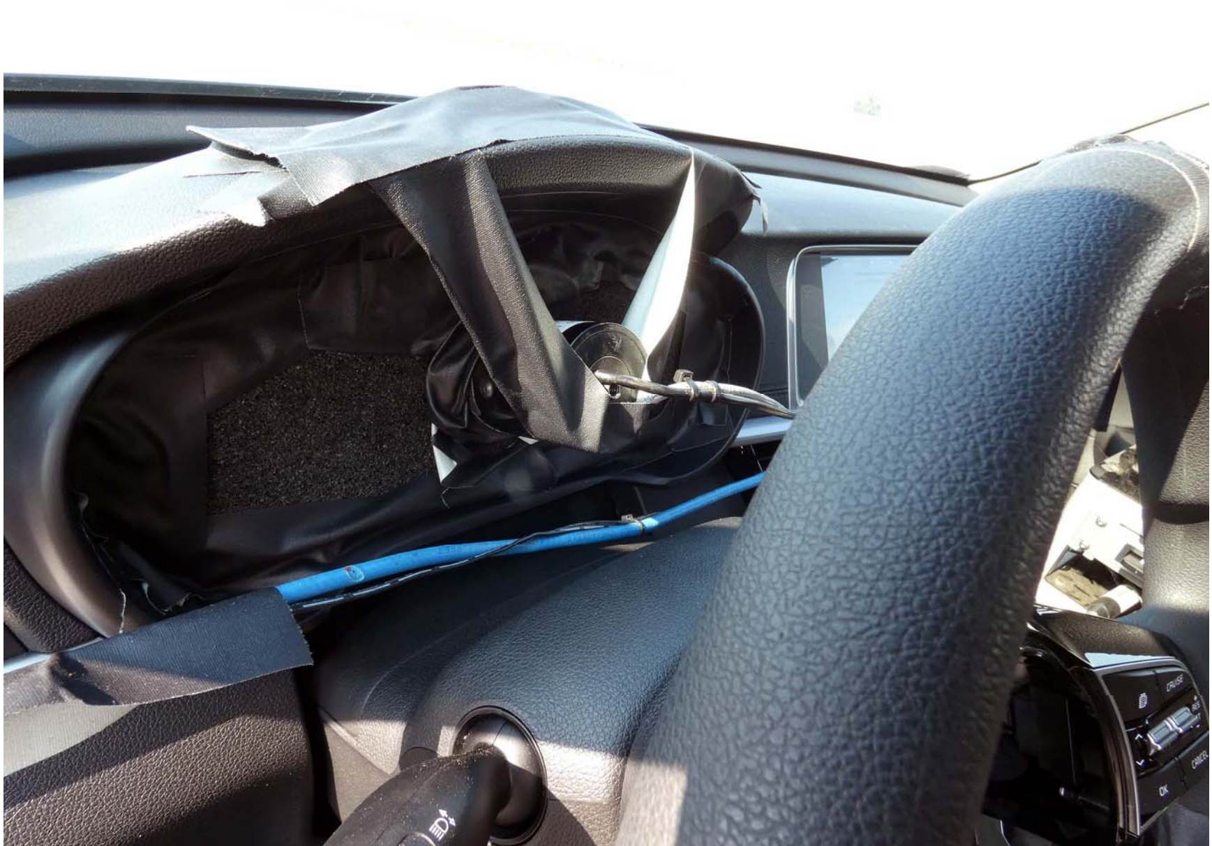
Figure A7. Sensor for Detecting Visual Alerts
