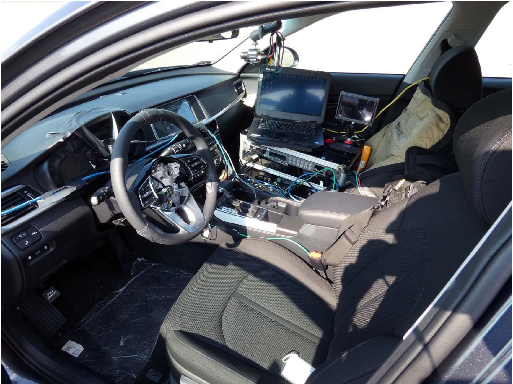
Figure A9. Computer Installed in Test Vehicle
