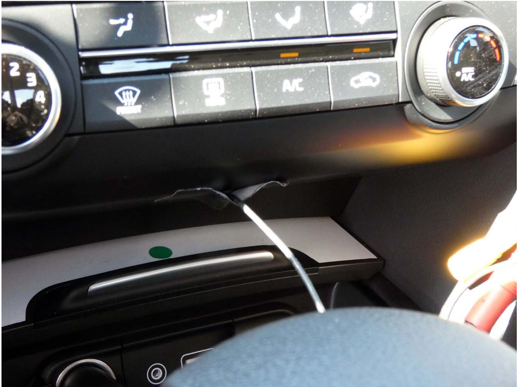
Figure A8. Sensor for Detecting Auditory Alerts
