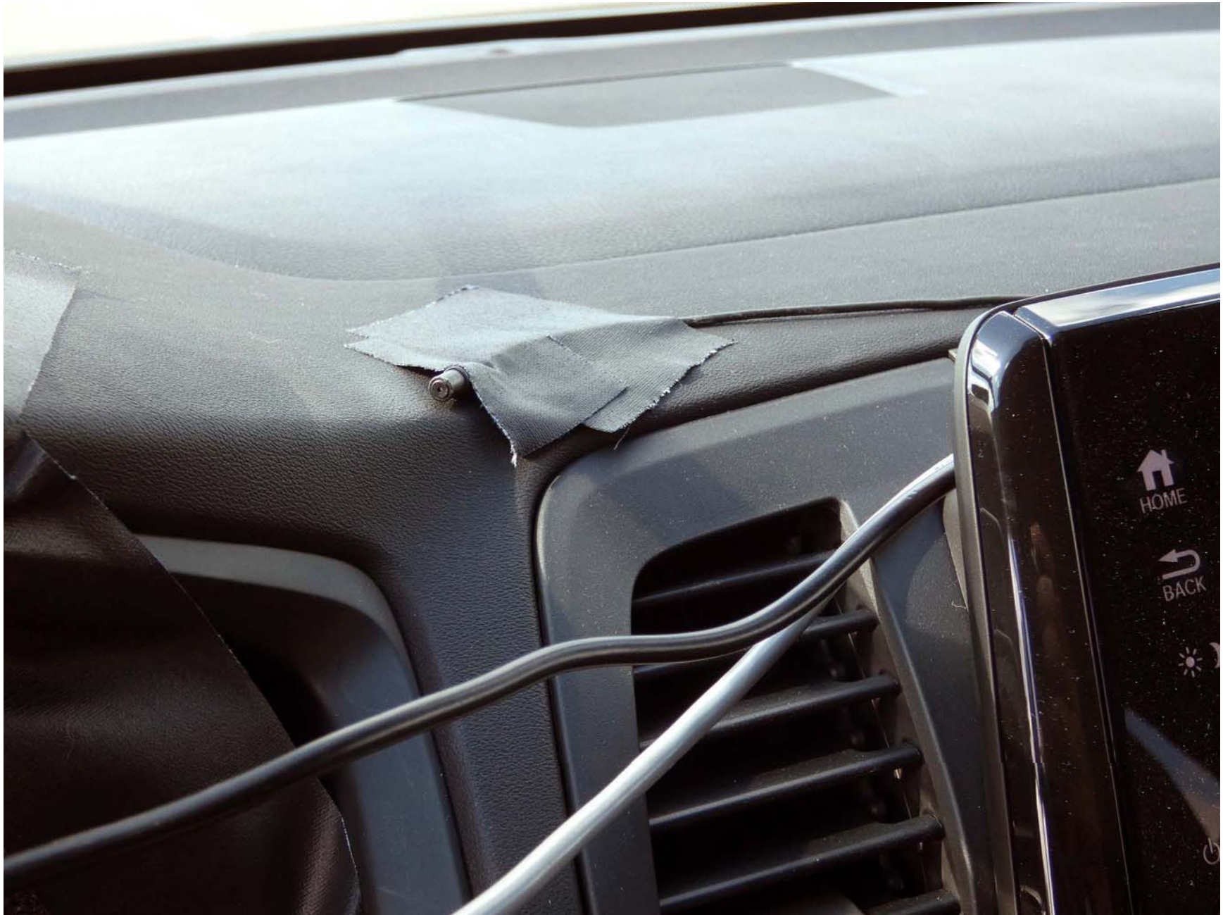
Figure A11. Sensor for Detecting Auditory Alerts
