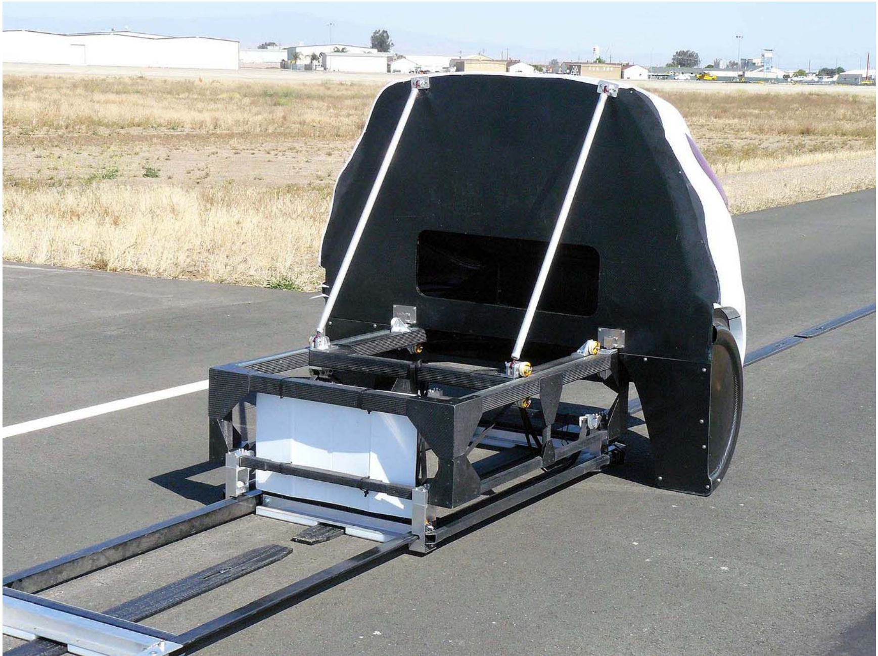
Figure A7. Load Frame/Slider of SSV
