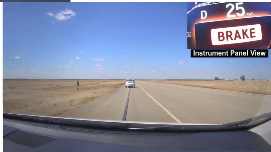
Figure A17. CMBS (AEB) Visual Alert Shown as Inset in Out-the-Window View
