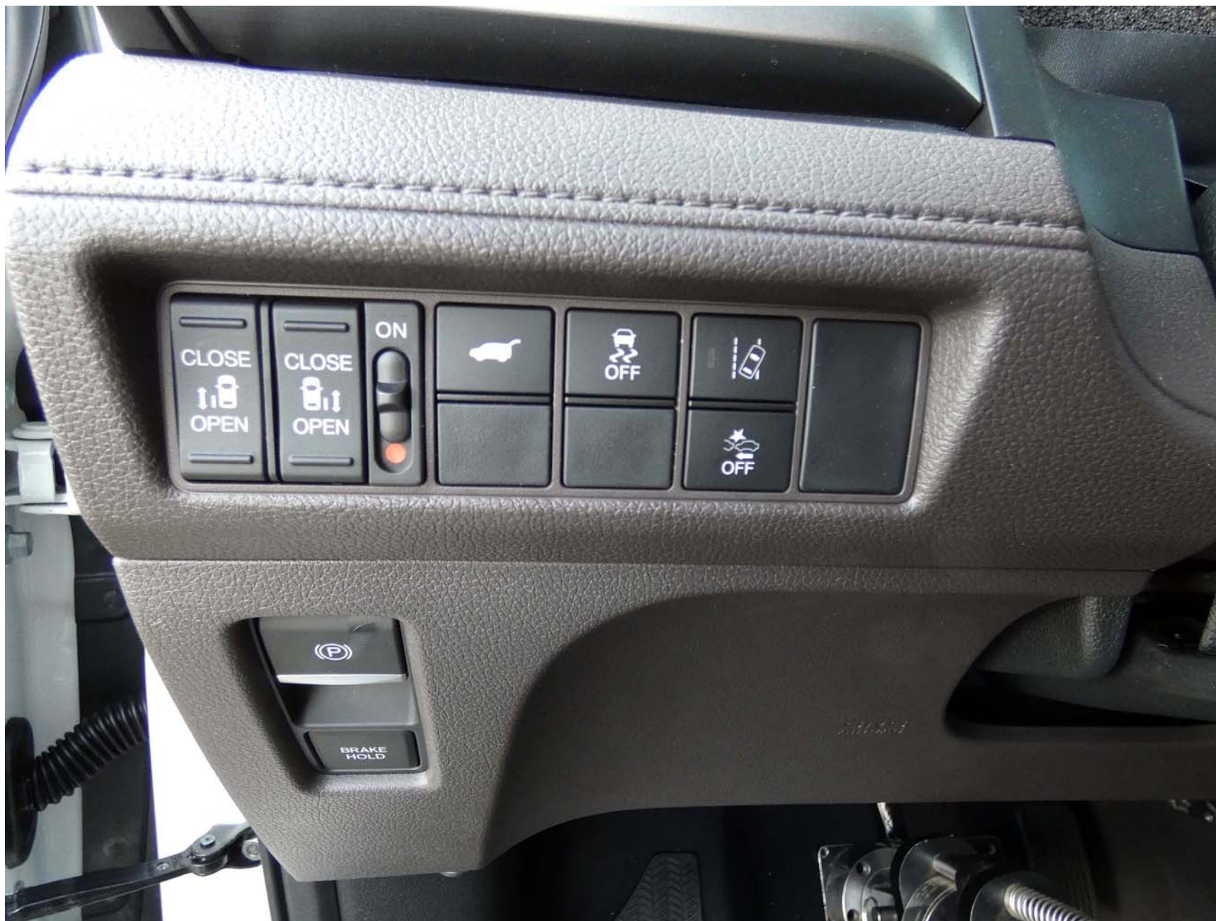
Figure A18. CMBS (AEB) On/Off Switch
