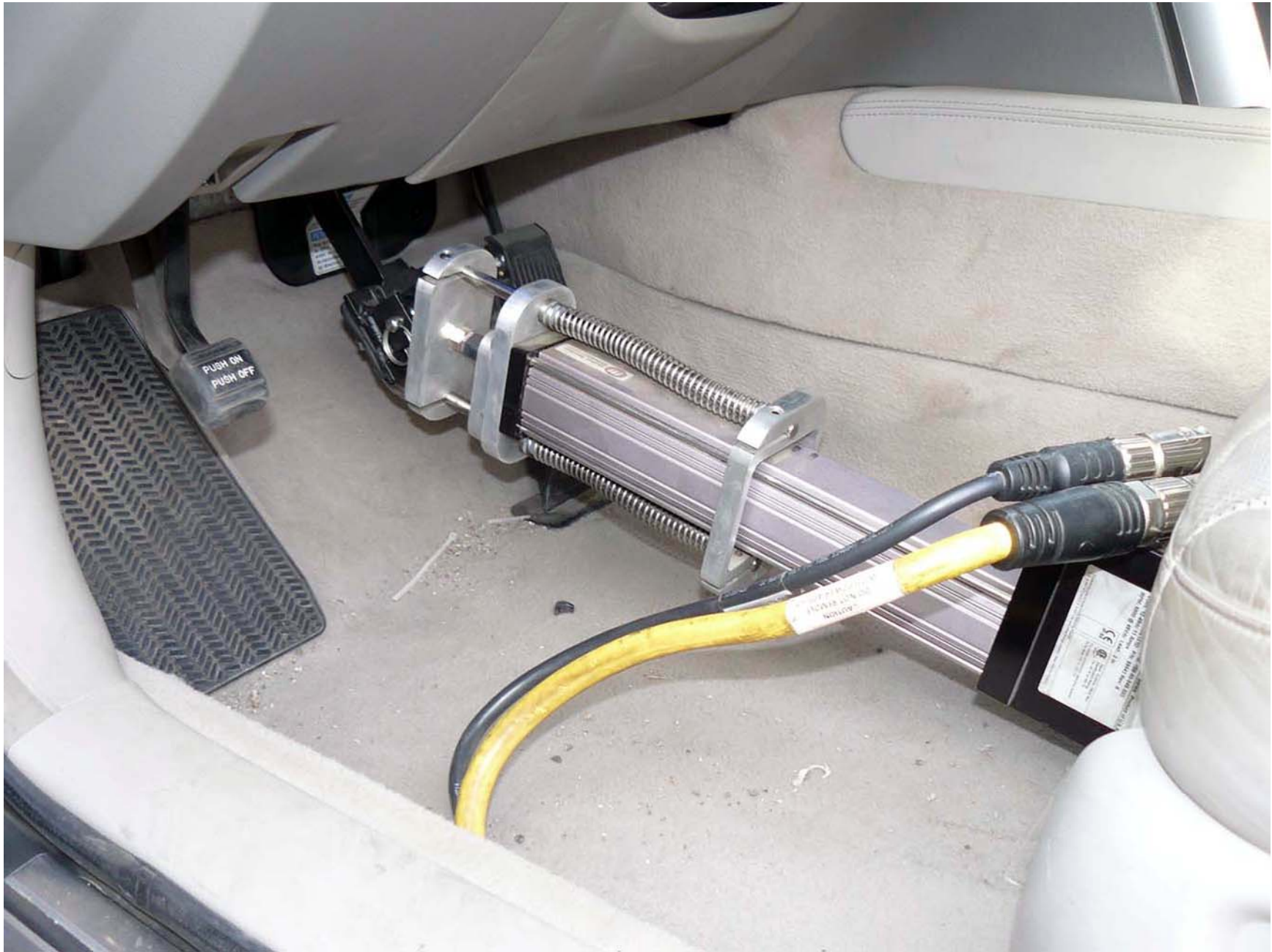
Figure A14. Brake Actuator Installed in POV System A-16
