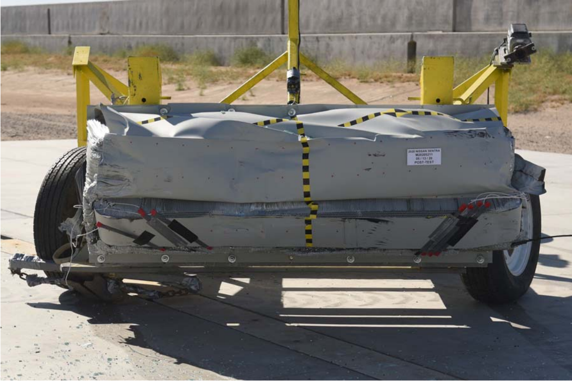
FIGURE 85. Post-Test Front View of MDB Impactor Face
