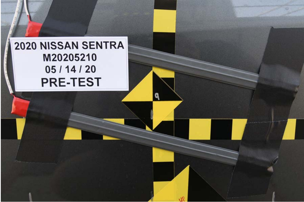
FIGURE 19. Pre-Test Close-Up View of Impact Point Target
