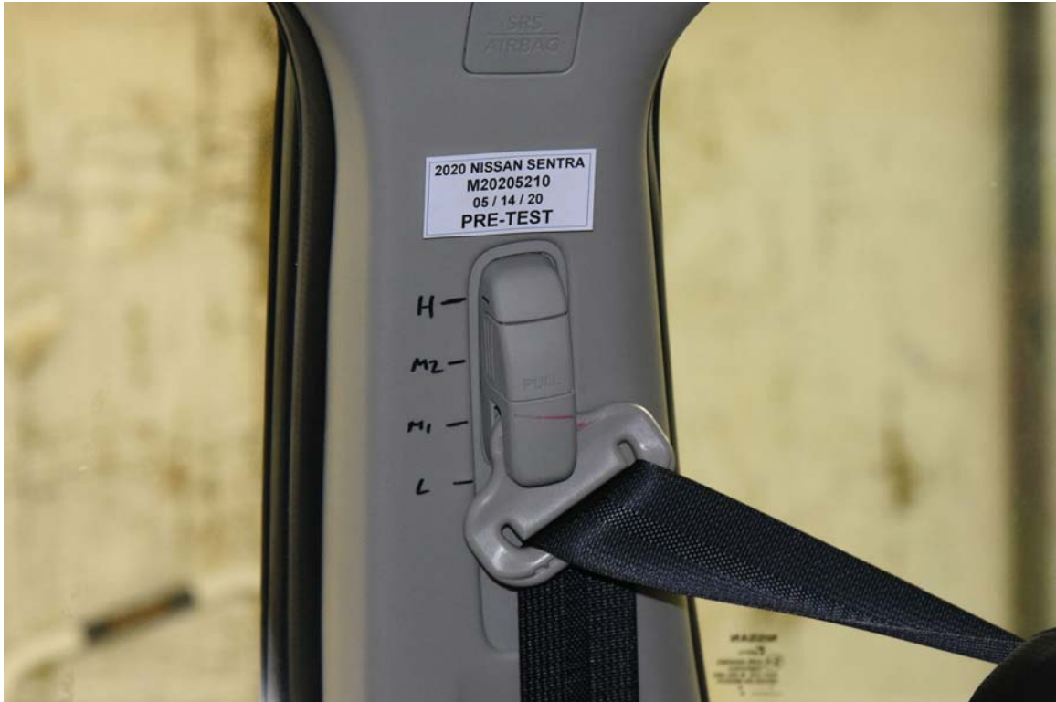
FIGURE 33. Pre-Test View of Belt Anchorage for Dummy
