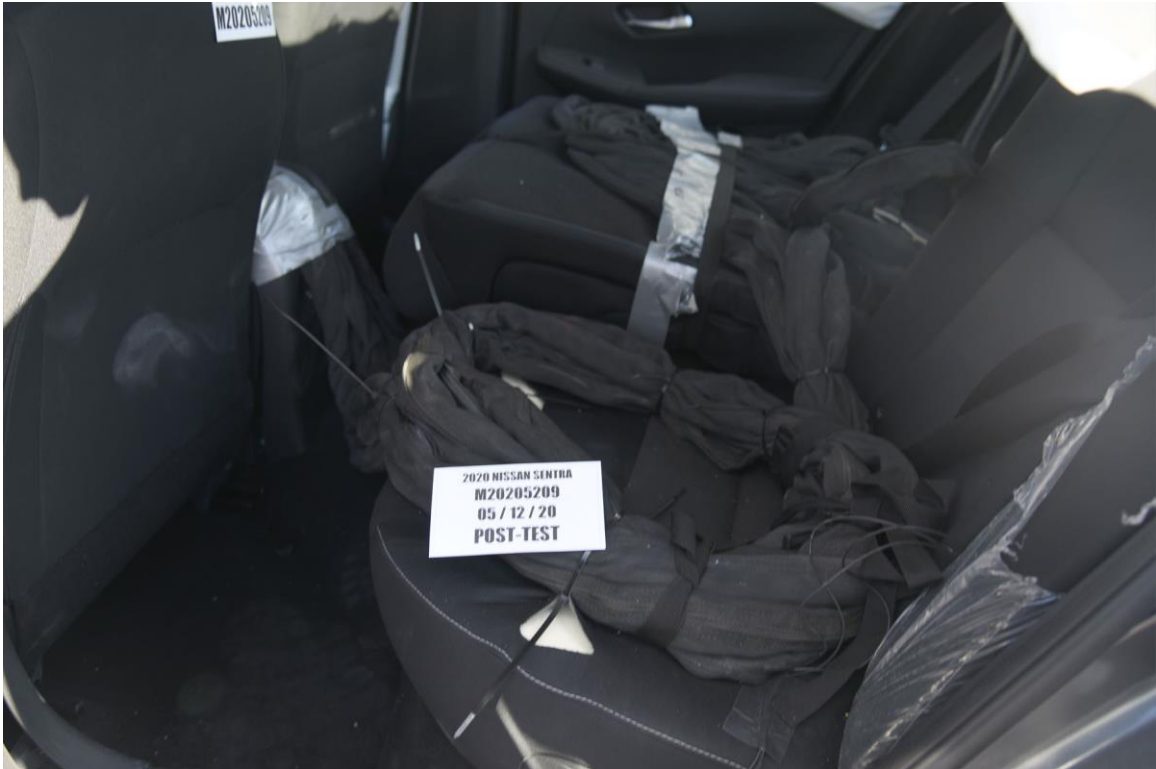
FIGURE 29. Post-Test Dummy Cable Routing
