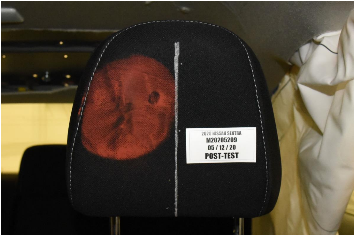
FIGURE 50. Post-Test Driver Dummy Contact with Headrest
