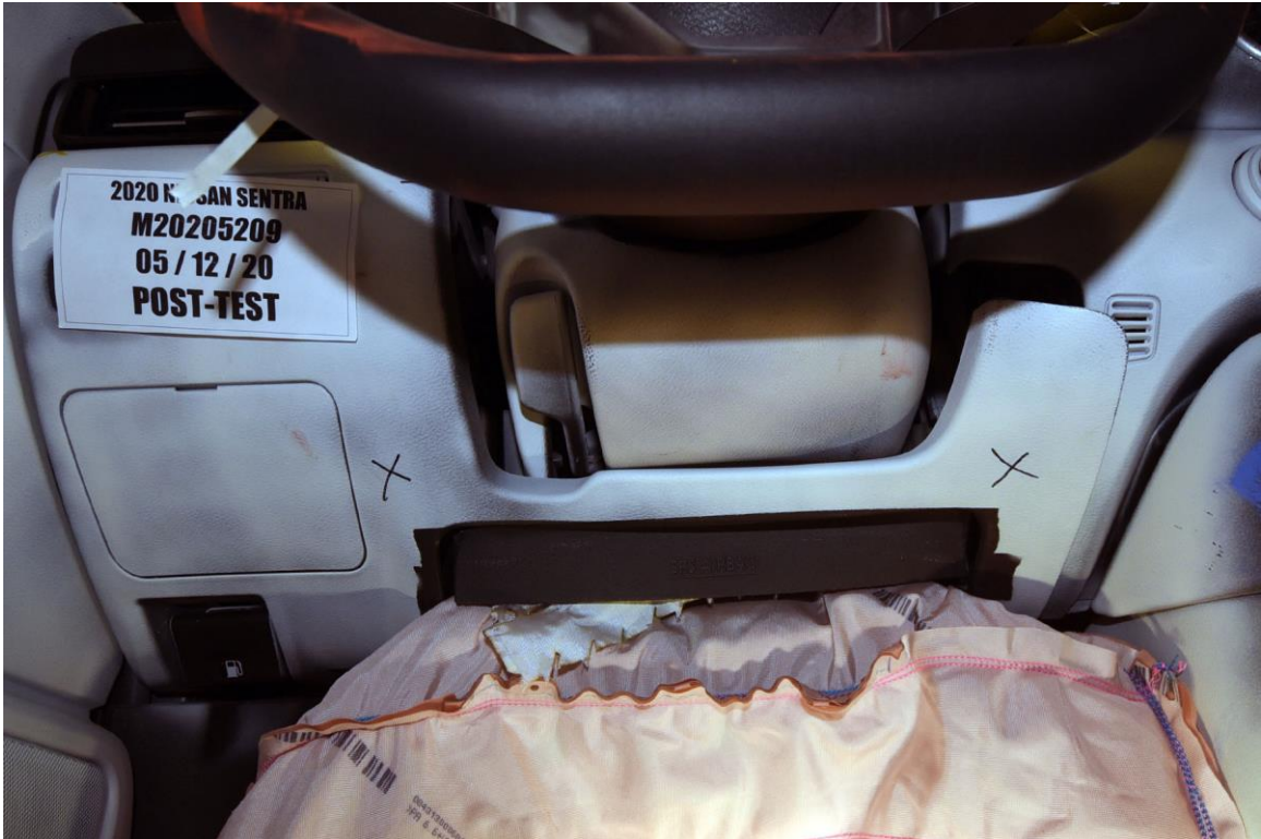
FIGURE 45. Post-Test Driver's Side Knee Bolster
