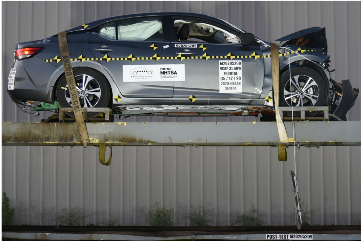
FIGURE 77. Vehicle at 0° on Static Rollover Device
