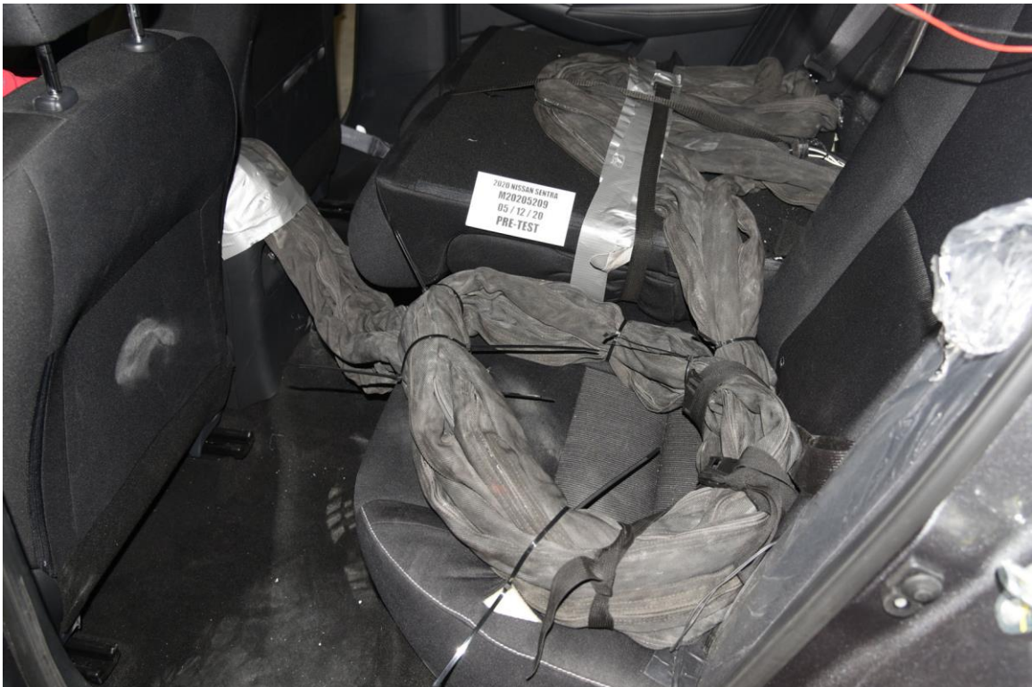
FIGURE 28. Pre-Test Dummy Cable Routing
