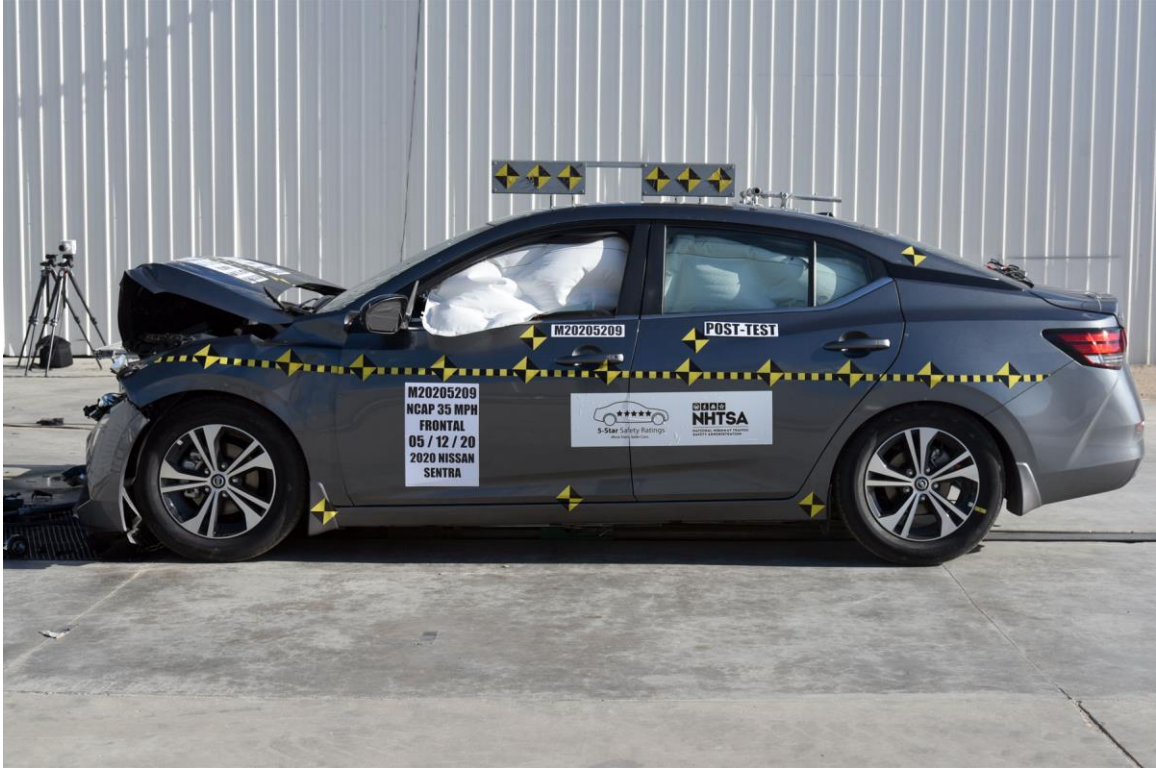
FIGURE 11. Post-Test Left View of Test Vehicle
