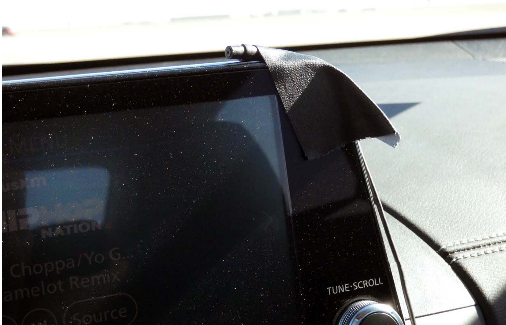
Figure A10. Sensor for Detecting Auditory Alerts
