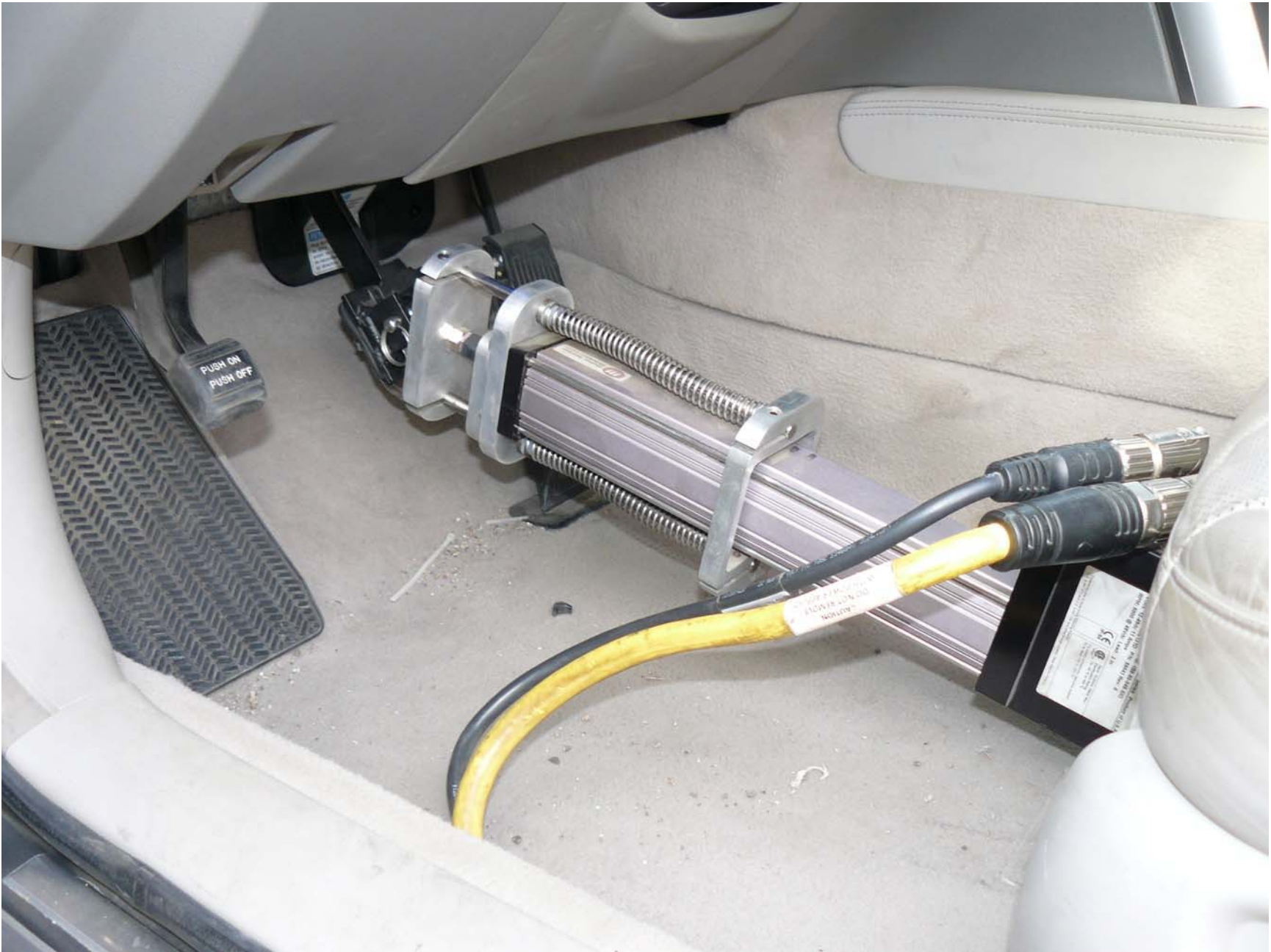
Figure A12. Brake Actuation System Installed in Principal Other Vehicle
