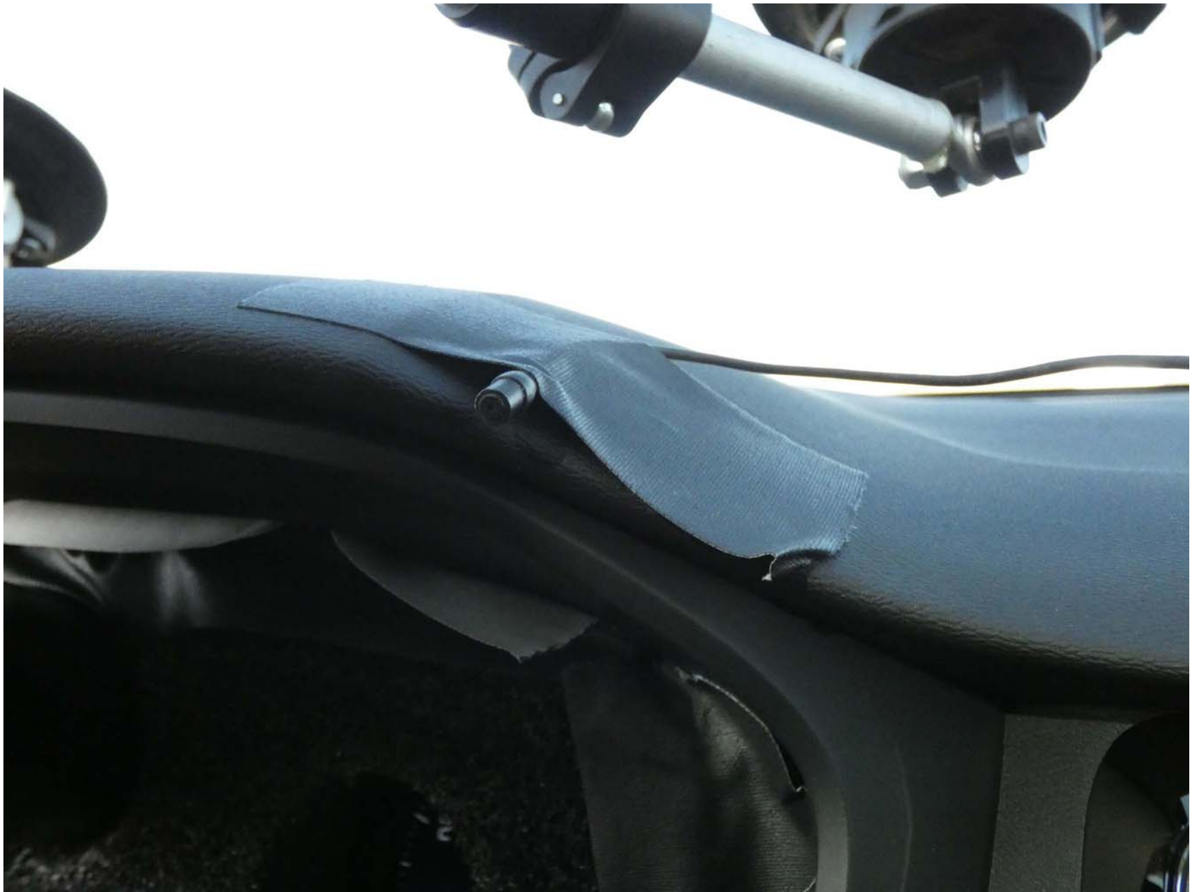
Figure A10. Sensor for Detecting Auditory Alerts
