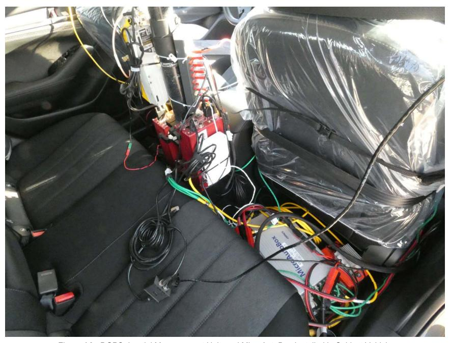
Figure A8. DGPS, Inertial Measurement Unit, and MicroAutoBox Installed in Subject Vehicle
