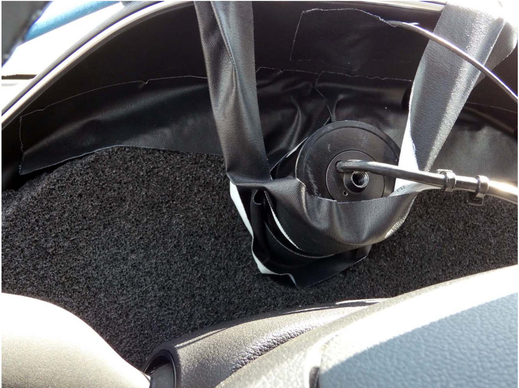
Figure A9. Sensor for Detecting Visual Alerts
