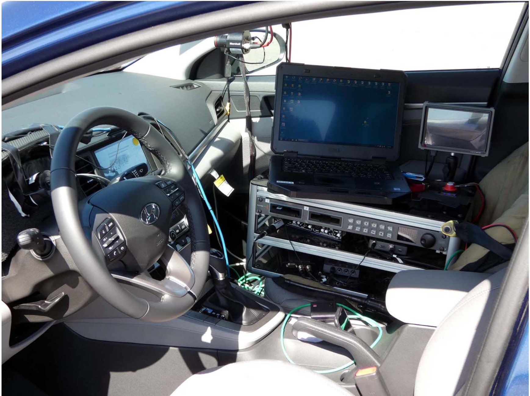
Figure A11. Computer Installed in Subject Vehicle
