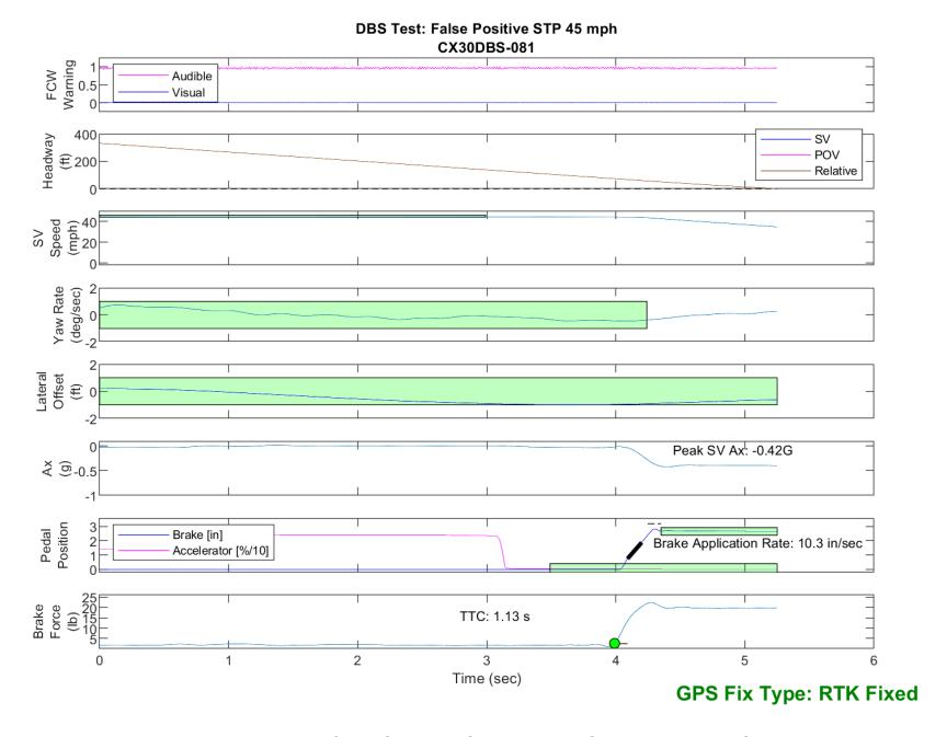
Figure E68. Time History for DBS Run 81, SV Encounters Steel Trench Plate, SV 45 mph
