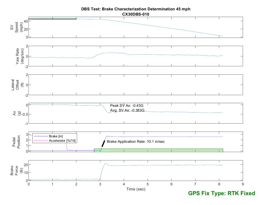
Figure E78. Time History for DBS Run 10, Brake Characterization Determination 45 mph
