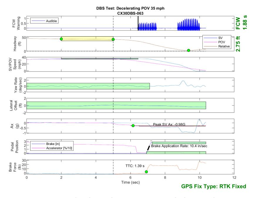
Figure E40. Time History for DBS Run 63, SV Encounters Decelerating POV, SV 35 mph, POV 35 mph
