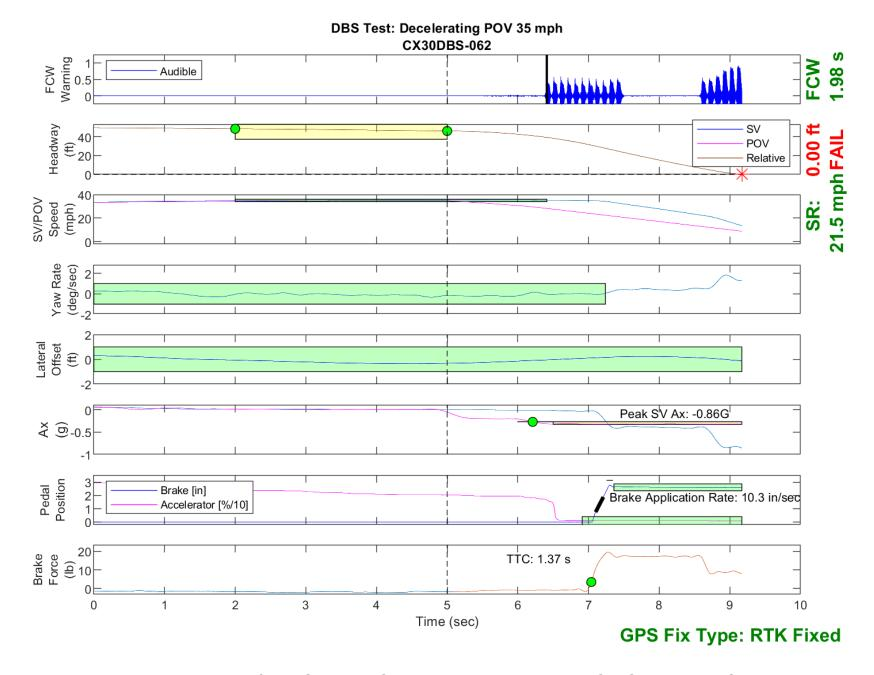
Figure E39. Time History for DBS Run 62, SV Encounters Decelerating POV, SV 35 mph, POV 35 mph
