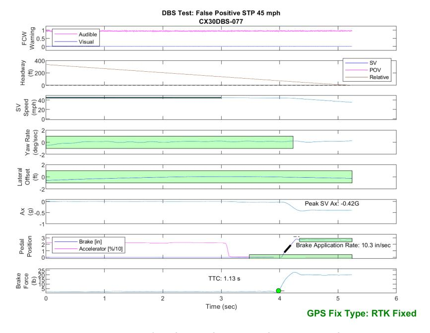
Figure E64. Time History for DBS Run 77, SV Encounters Steel Trench Plate, SV 45 mph
