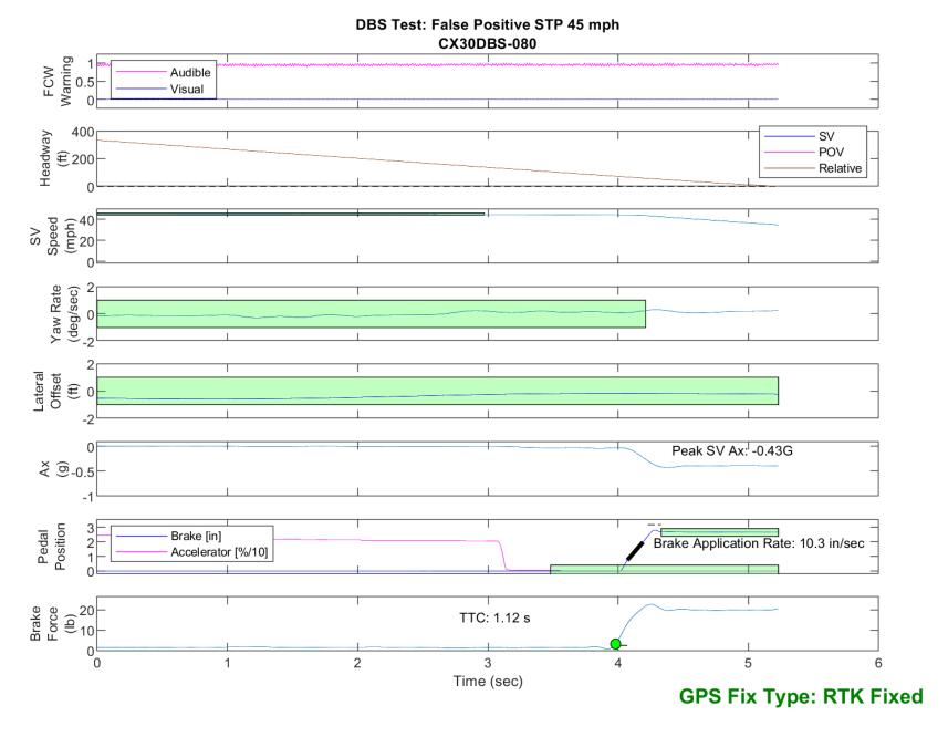
Figure E67. Time History for DBS Run 80, SV Encounters Steel Trench Plate, SV 45 mph
