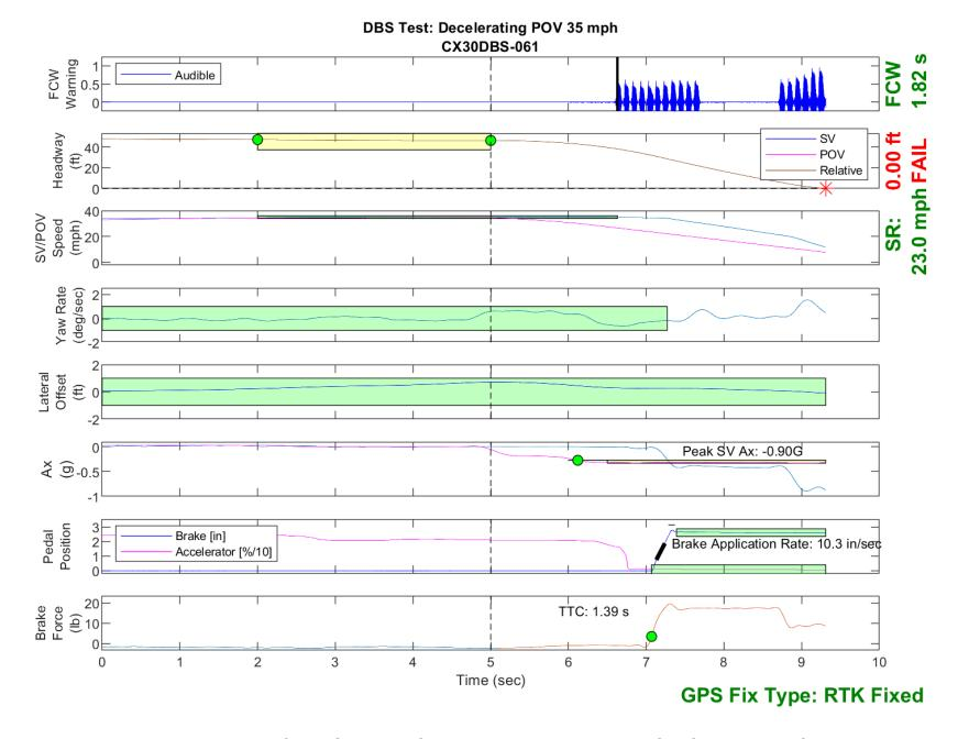
Figure E38. Time History for DBS Run 61, SV Encounters Decelerating POV, SV 35 mph, POV 35 mph
