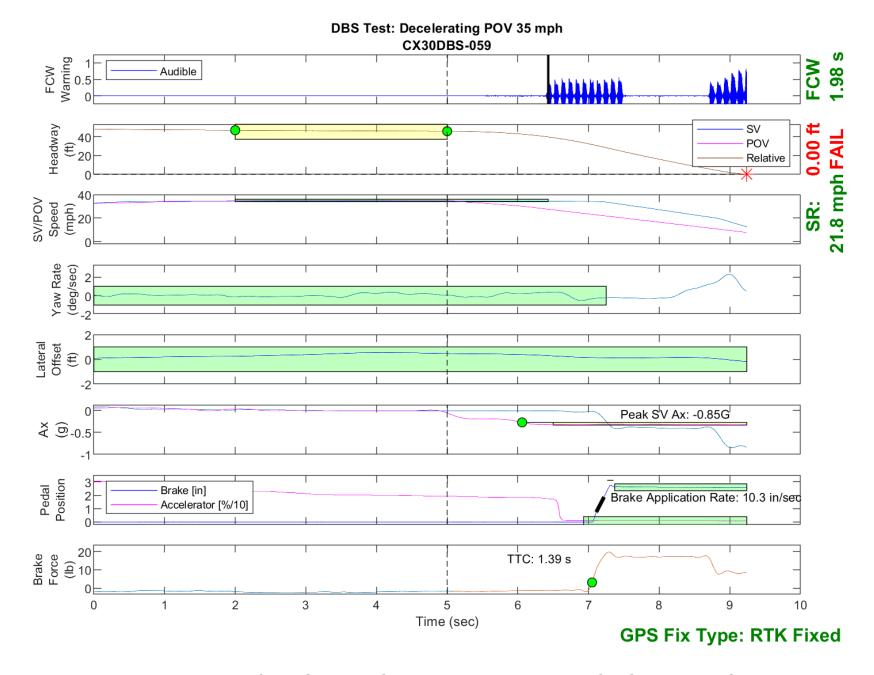
Figure E37. Time History for DBS Run 59, SV Encounters Decelerating POV, SV 35 mph, POV 35 mph
