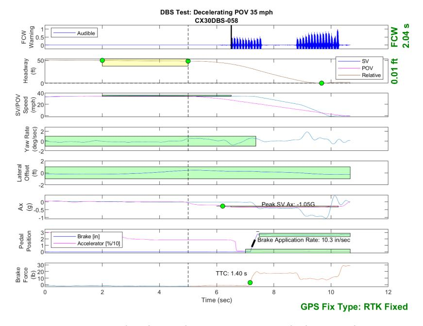
Figure E36. Time History for DBS Run 58, SV Encounters Decelerating POV, SV 35 mph, POV 35 mph
