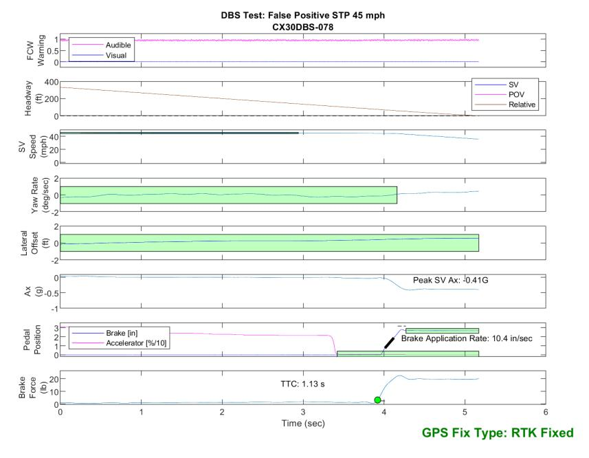
Figure E65. Time History for DBS Run 78, SV Encounters Steel Trench Plate, SV 45 mph
