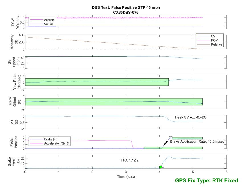
Figure E63. Time History for DBS Run 76, SV Encounters Steel Trench Plate, SV 45 mph
