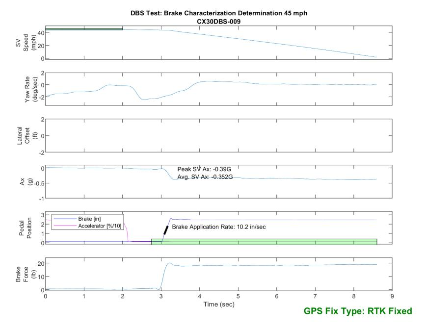
Figure E77. Time History for DBS Run 9, Brake Characterization Determination 45 mph
