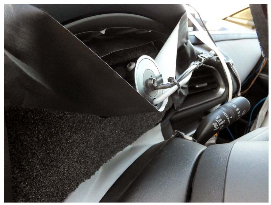
Figure A11. Sensor for Detecting Visual Alerts A-13
