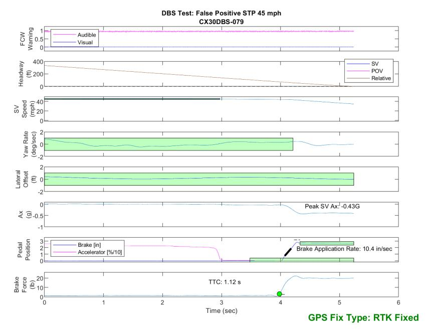
Figure E66. Time History for DBS Run 79, SV Encounters Steel Trench Plate, SV 45 mph
