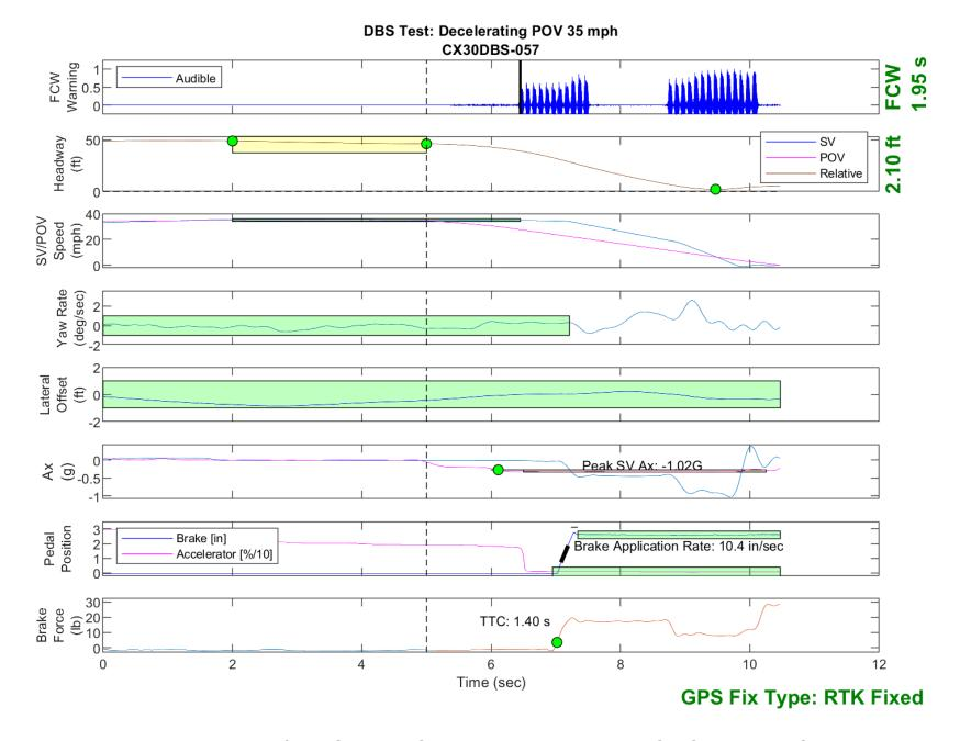
Figure E35. Time History for DBS Run 57, SV Encounters Decelerating POV, SV 35 mph, POV 35 mph
