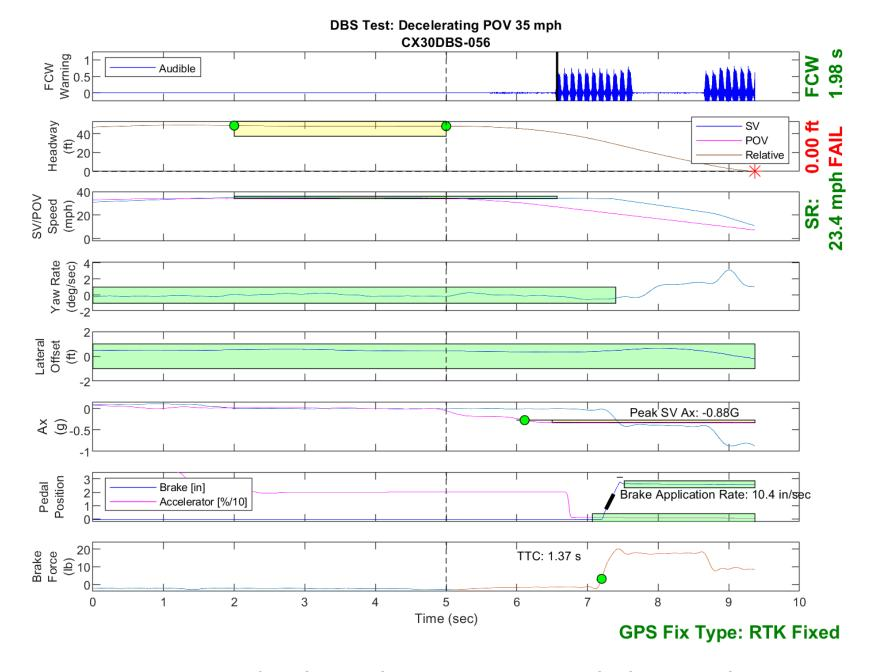
Figure E34. Time History for DBS Run 56, SV Encounters Decelerating POV, SV 35 mph, POV 35 mph
