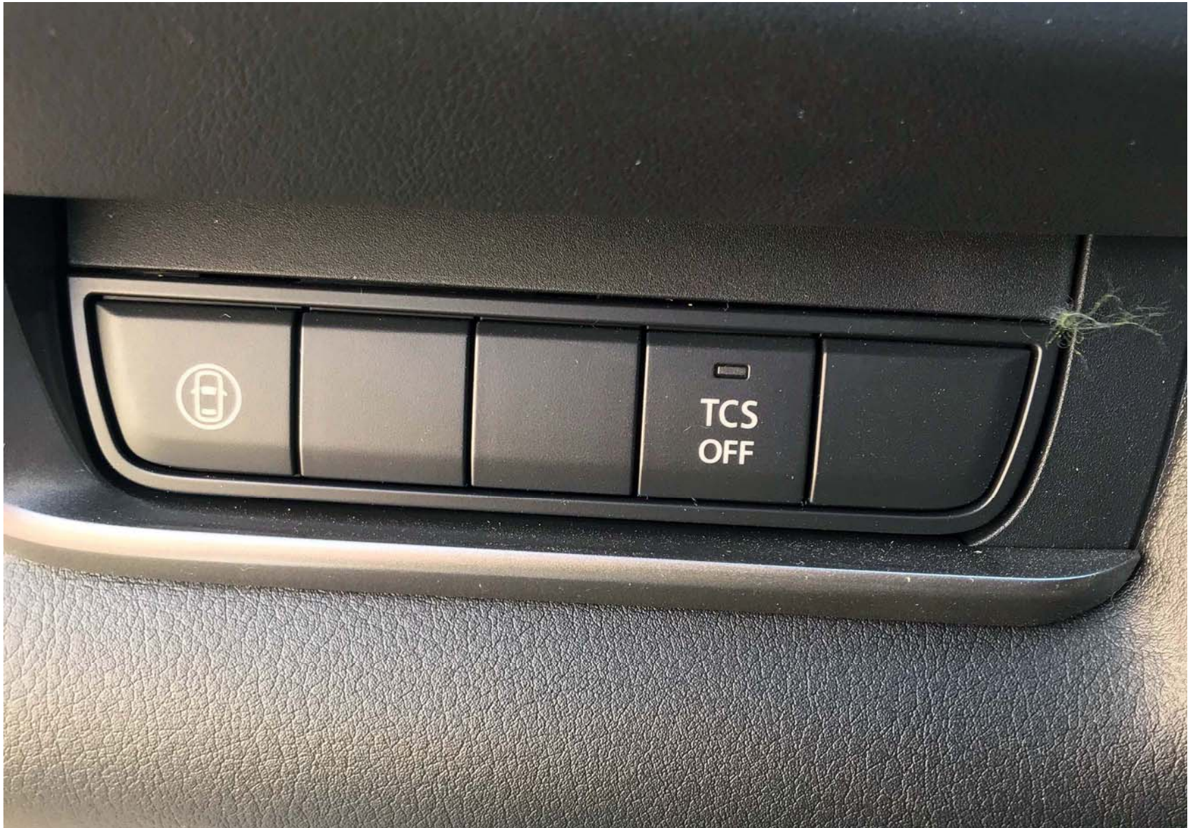
Figure A12. Switch to Enable/Disable i-ACTIVESENSE System Including LDW
