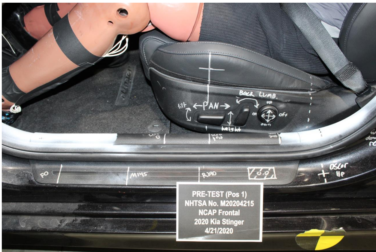
Figure A-36: Pre-Test Driver's Seat Fore-Aft Markings
