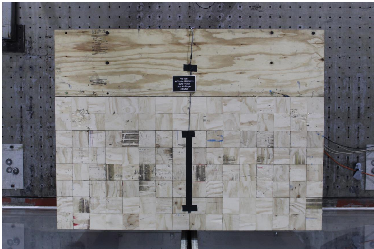
Figure A-2: Pre-Test Load Cell Wall
