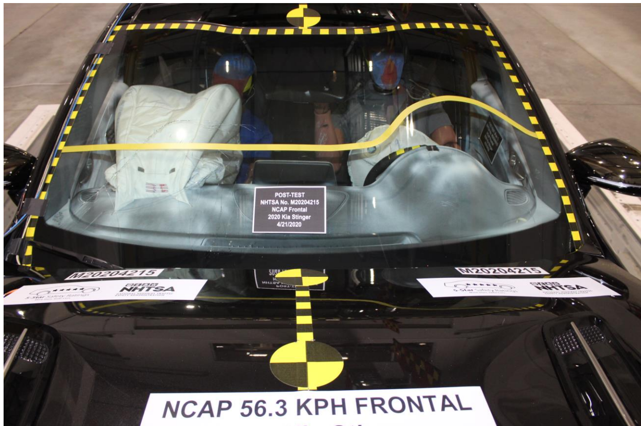
Figure A-19: Post-Test Windshield View
