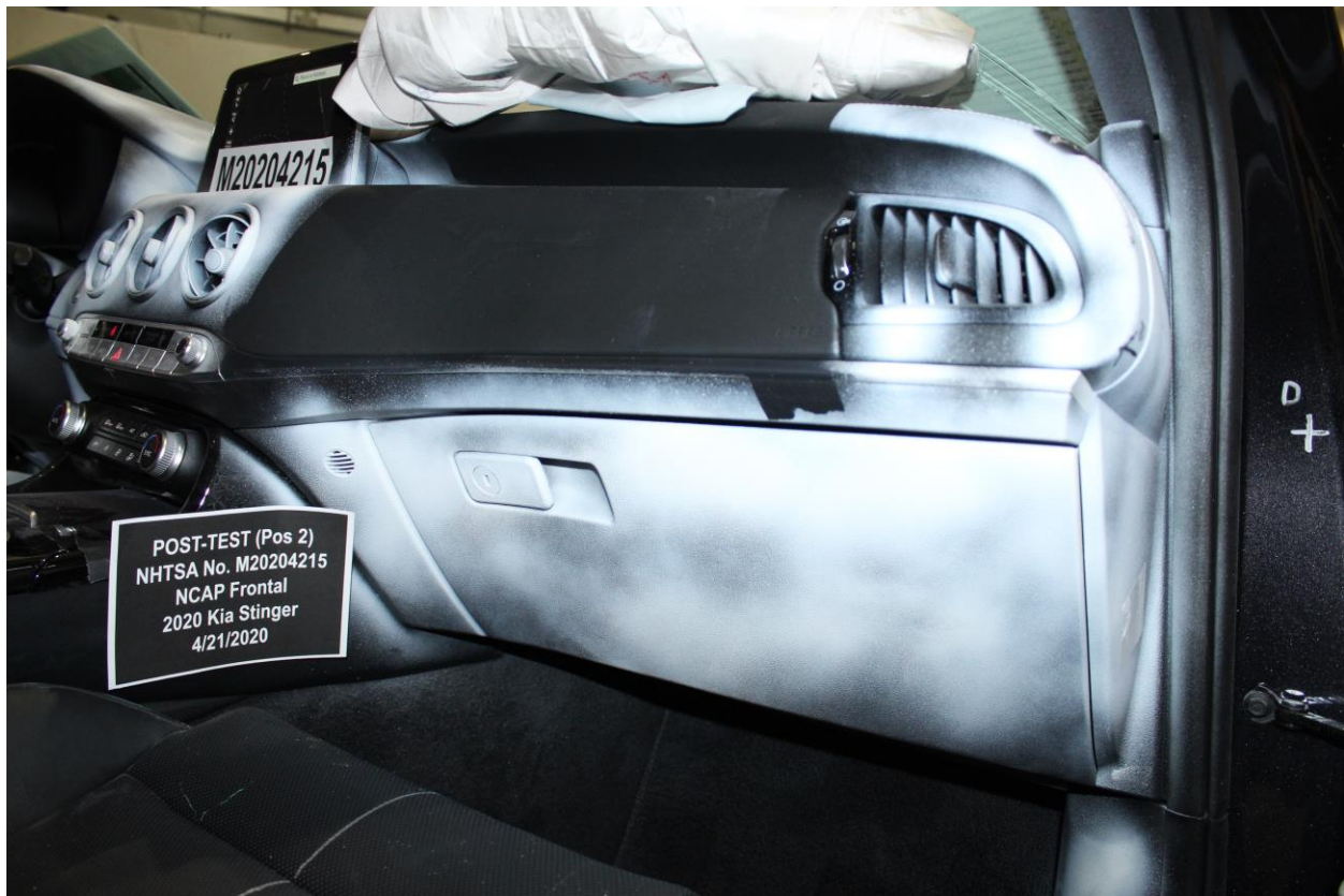
Figure A-68: Post-Test Passenger's Side Knee Bolster
