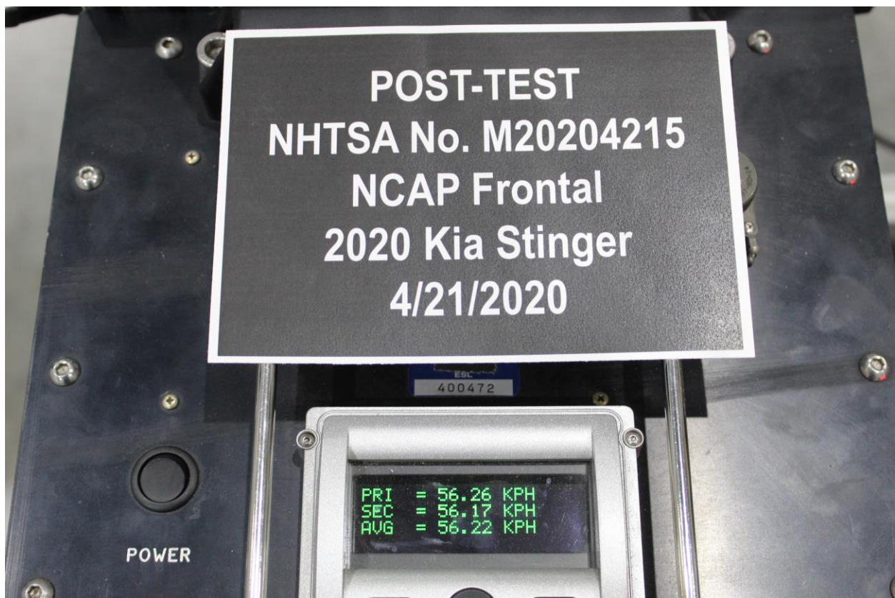
Figure A-76: Post-Test Speed Trap Read-Out
