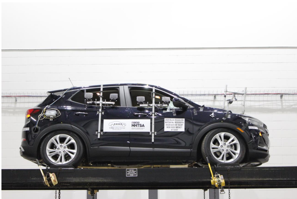
Figure A-100: FMVSS No. 301 Static Rollover 360 Degrees
