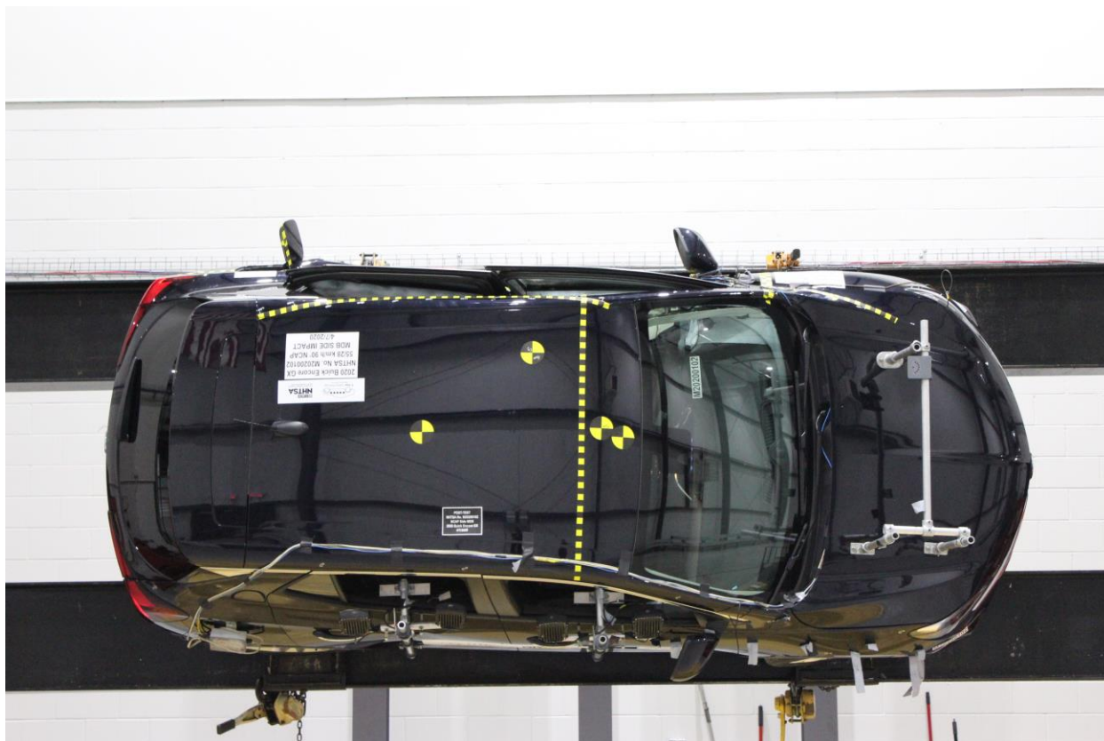
Figure A-99: FMVSS No. 301 Static Rollover 270 Degrees
