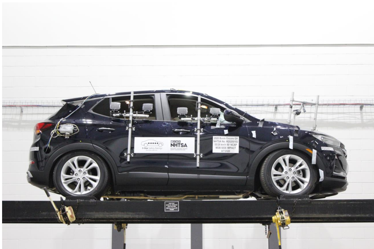
Figure A-96: FMVSS No. 301 Static Rollover 0 Degrees
