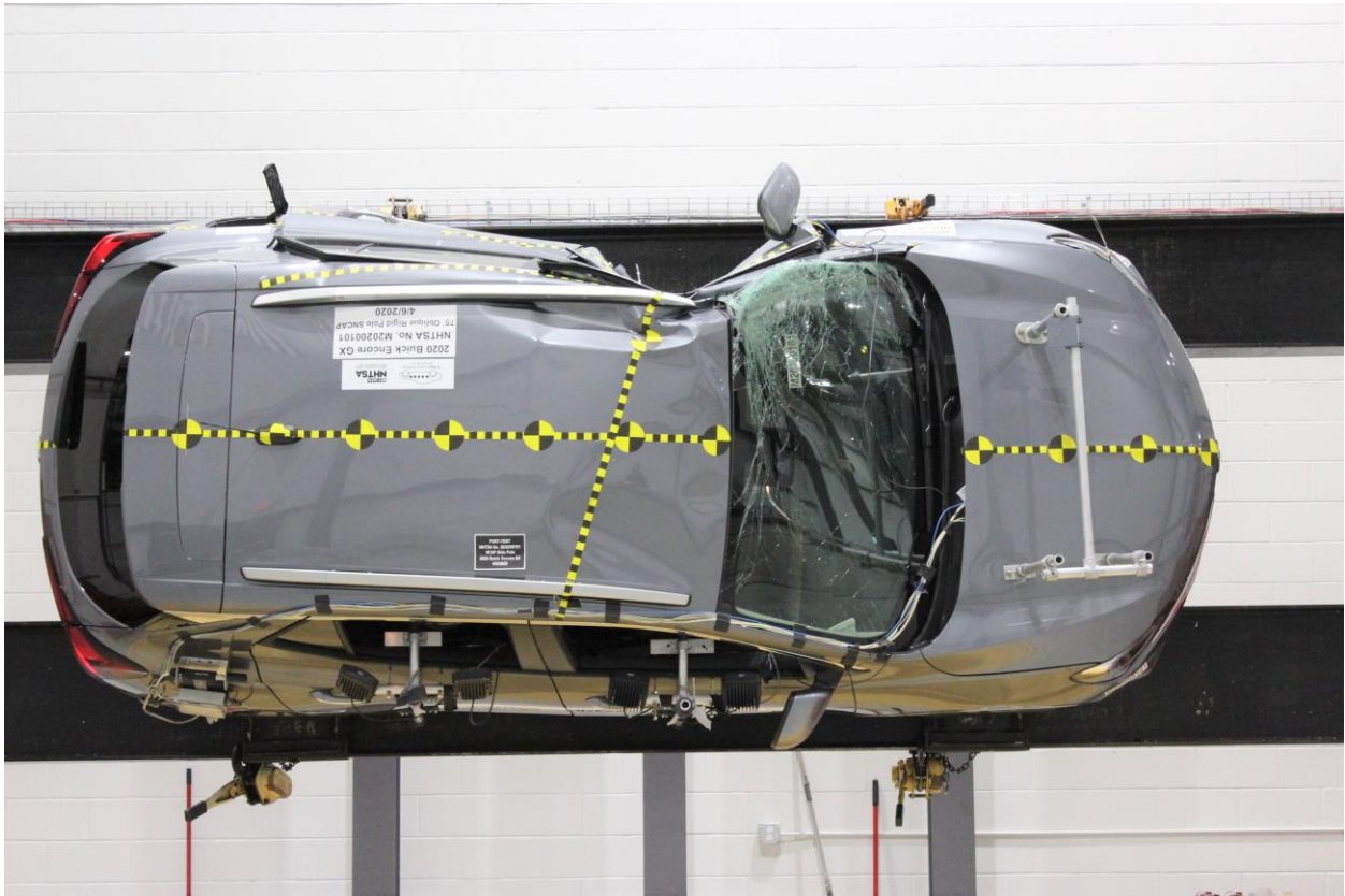
Figure A-66: FMVSS No. 301 Static Rollover 270 Degrees
