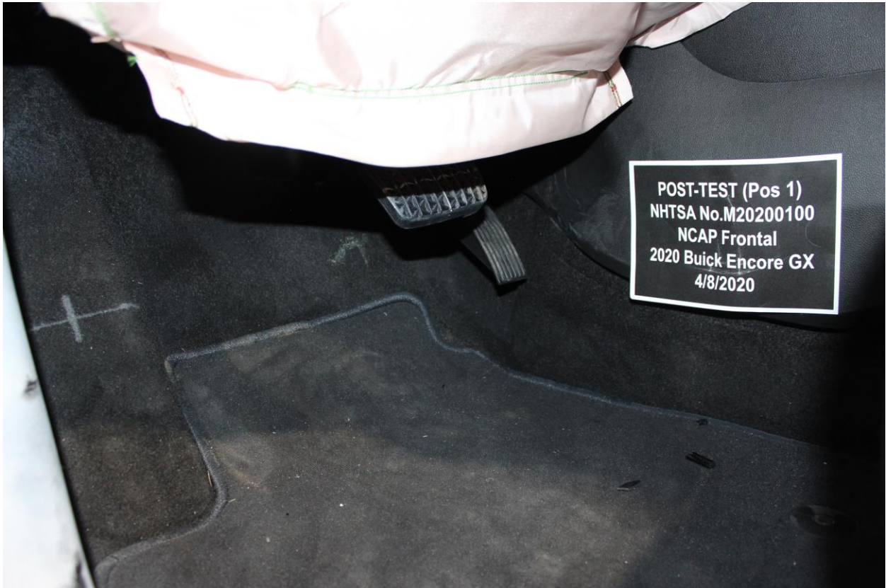
Figure A-47: Post-Test Driver's Side Floorpan
