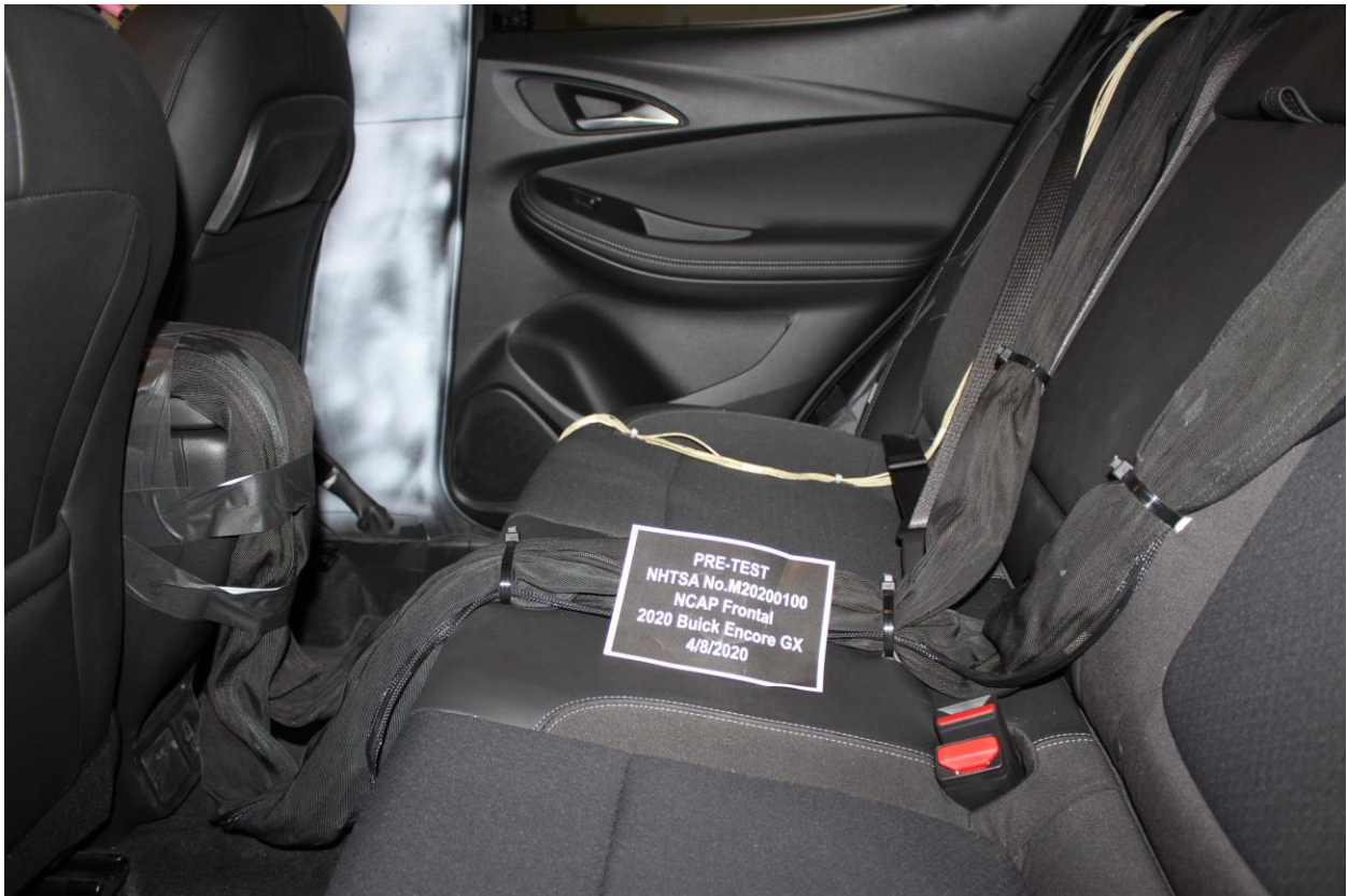
Figure A-28: Pre-Test Dummy Cable Routing
