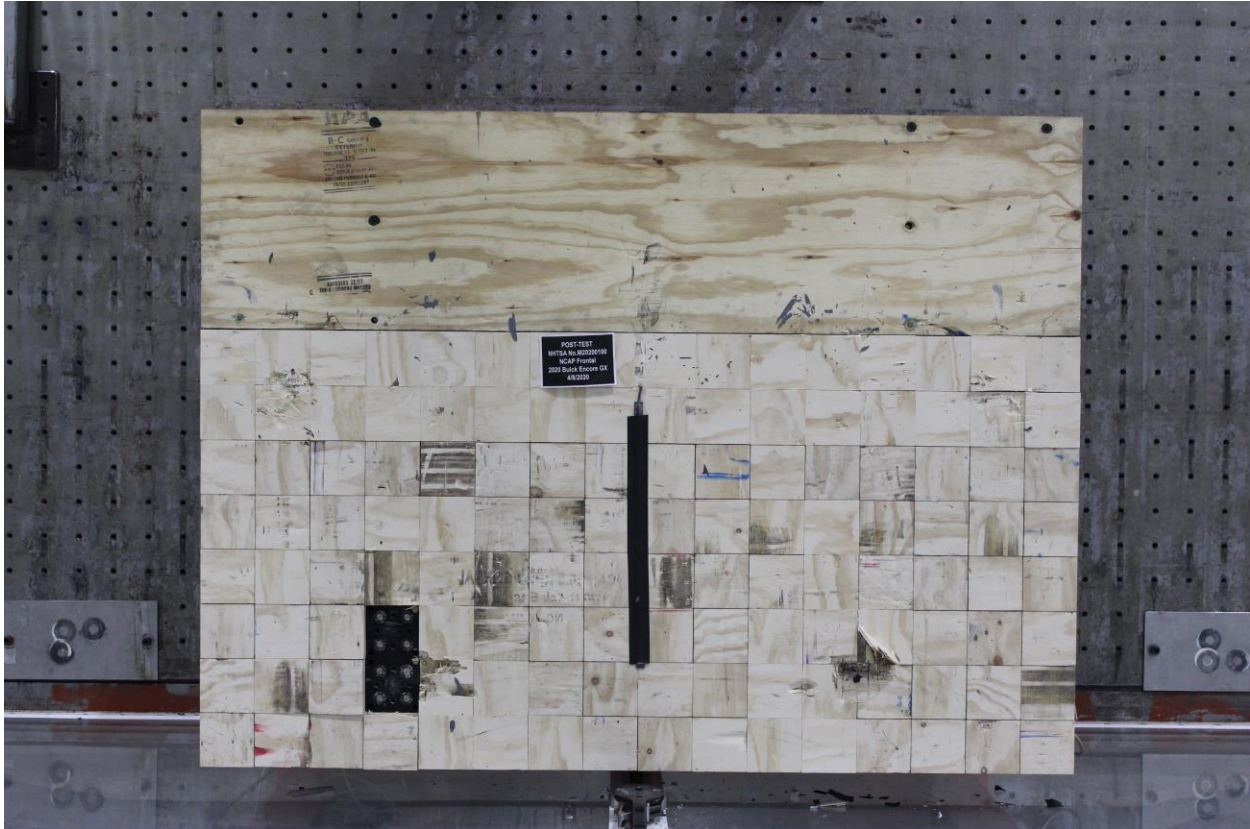
Figure A-3: Post-Test Load Cell Wall
