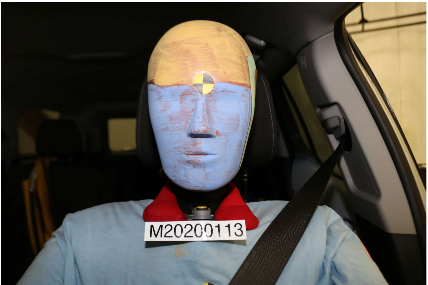
Photo No. 031 - Pre-Test Frontal View of Driver Dummy Head and Shoulders in Relation to Head Restraint
