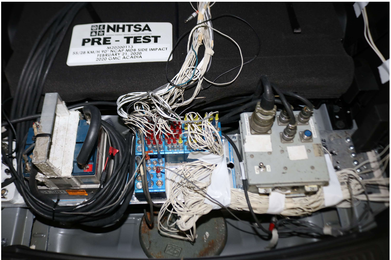
Photo No. 094 - Pre-Test Ballast View
