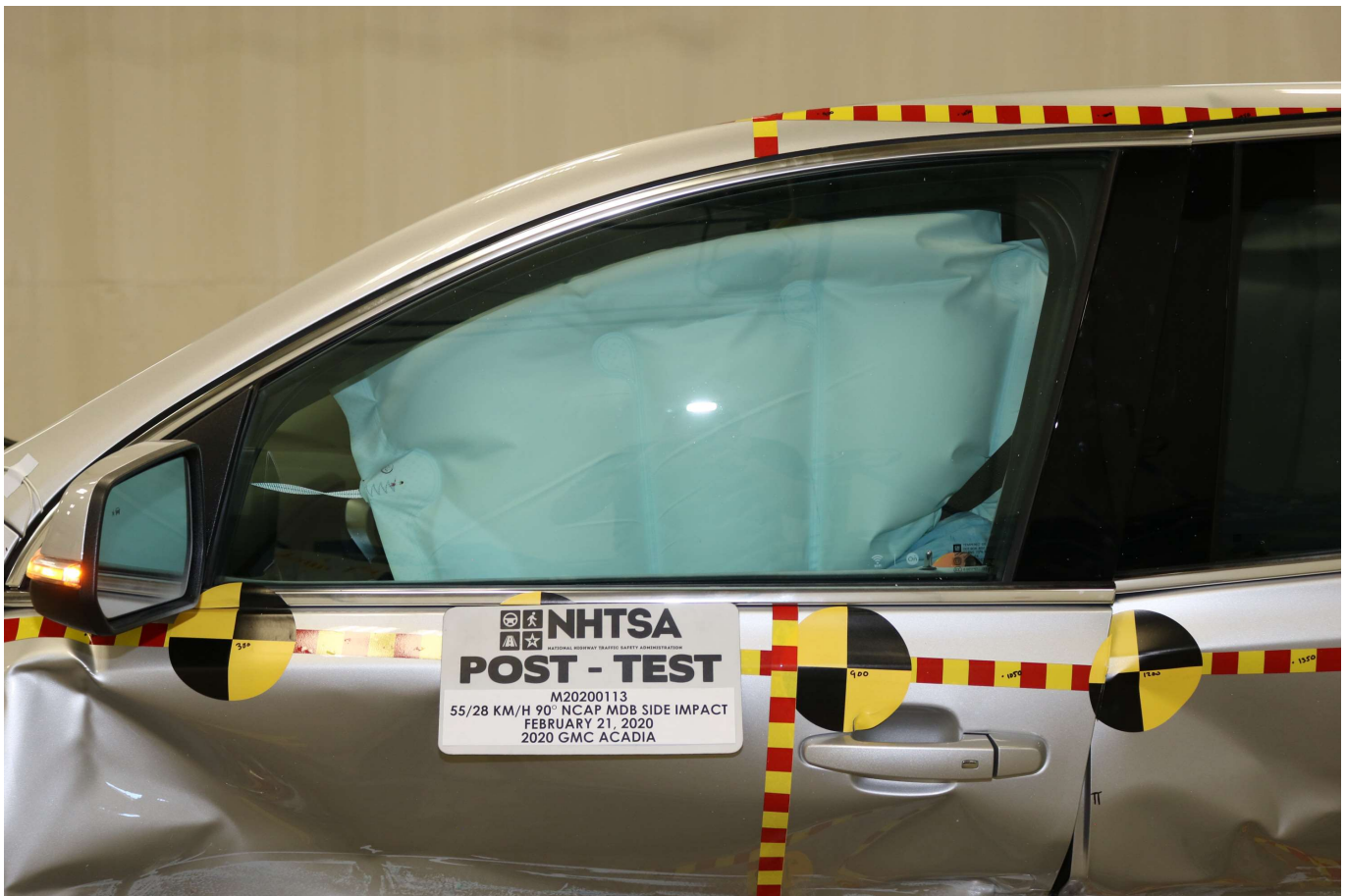
Photo No. 029 - Post-Test Left Side View of Driver Dummy Shoulder and Door Top View
