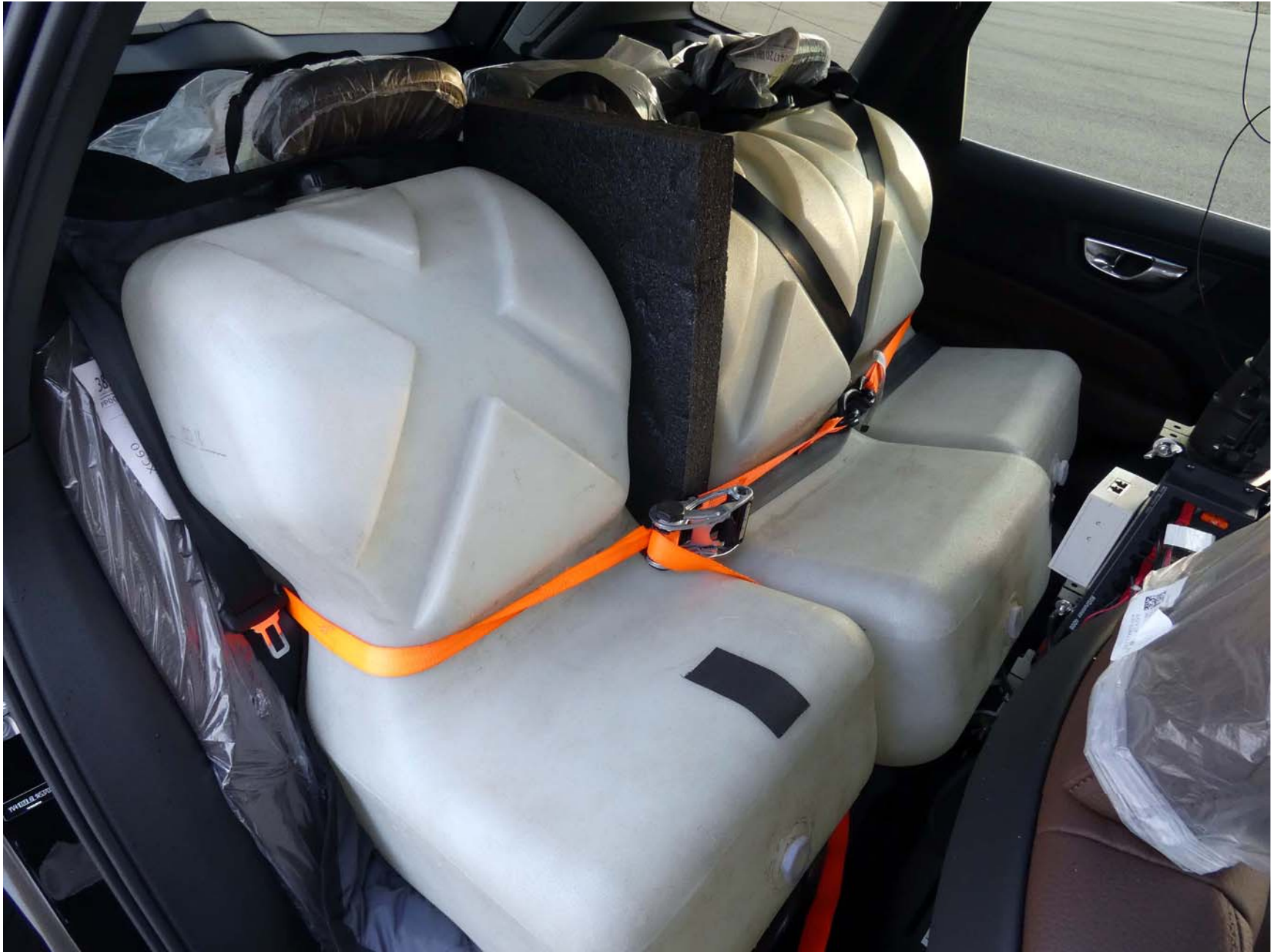
Figure A10. Ballast Condition
