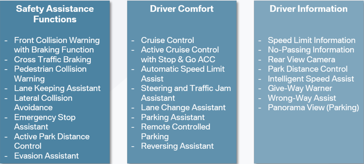
Figure 2. Advanced Driver Assistance Systems in the iNEXT.
