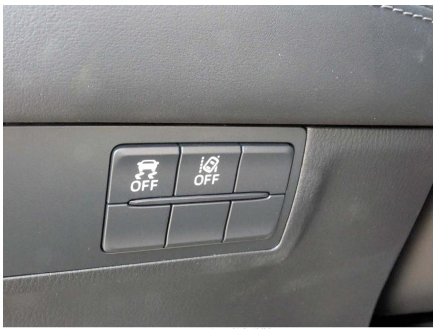
Figure A12. LDW (LDWS) On/Off Switch
