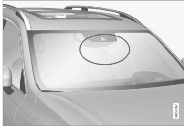
The area marked in the illustration must be cleaned regularly and kept free of decals, objects, solar film, etc.
