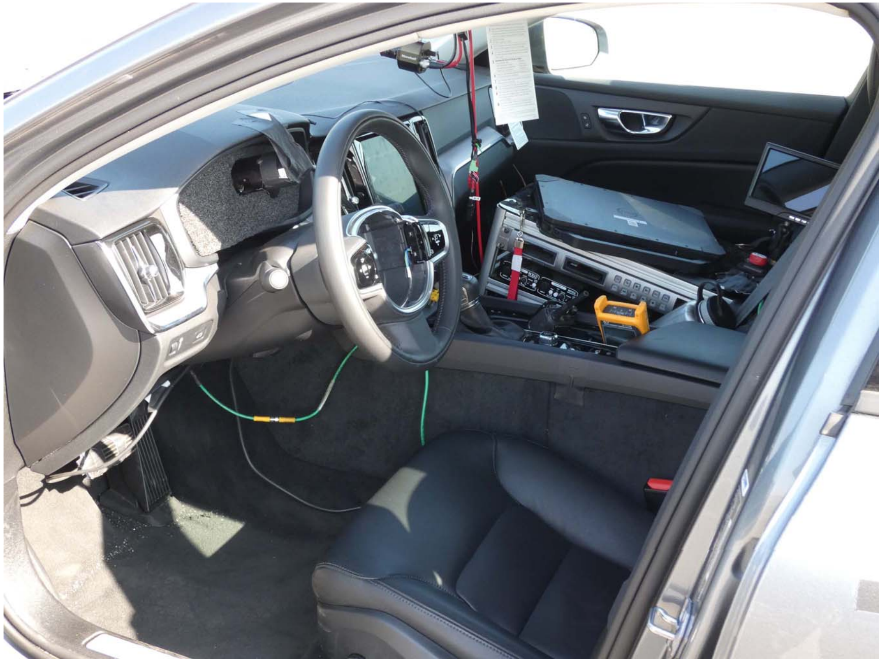
Figure A13. Computer Installed in Subject Vehicle
