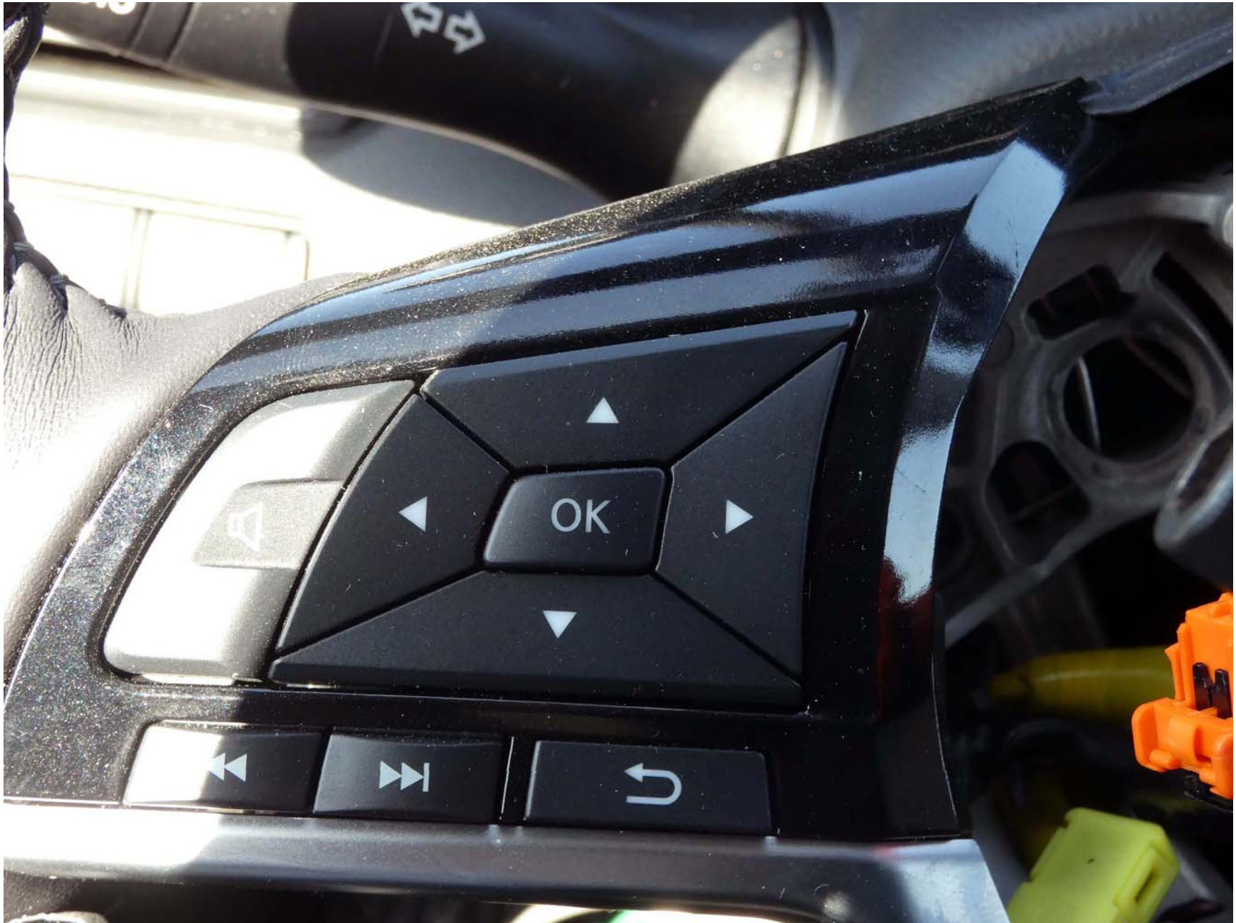
Figure A16. Controls for Changing Vehicle Parameters
