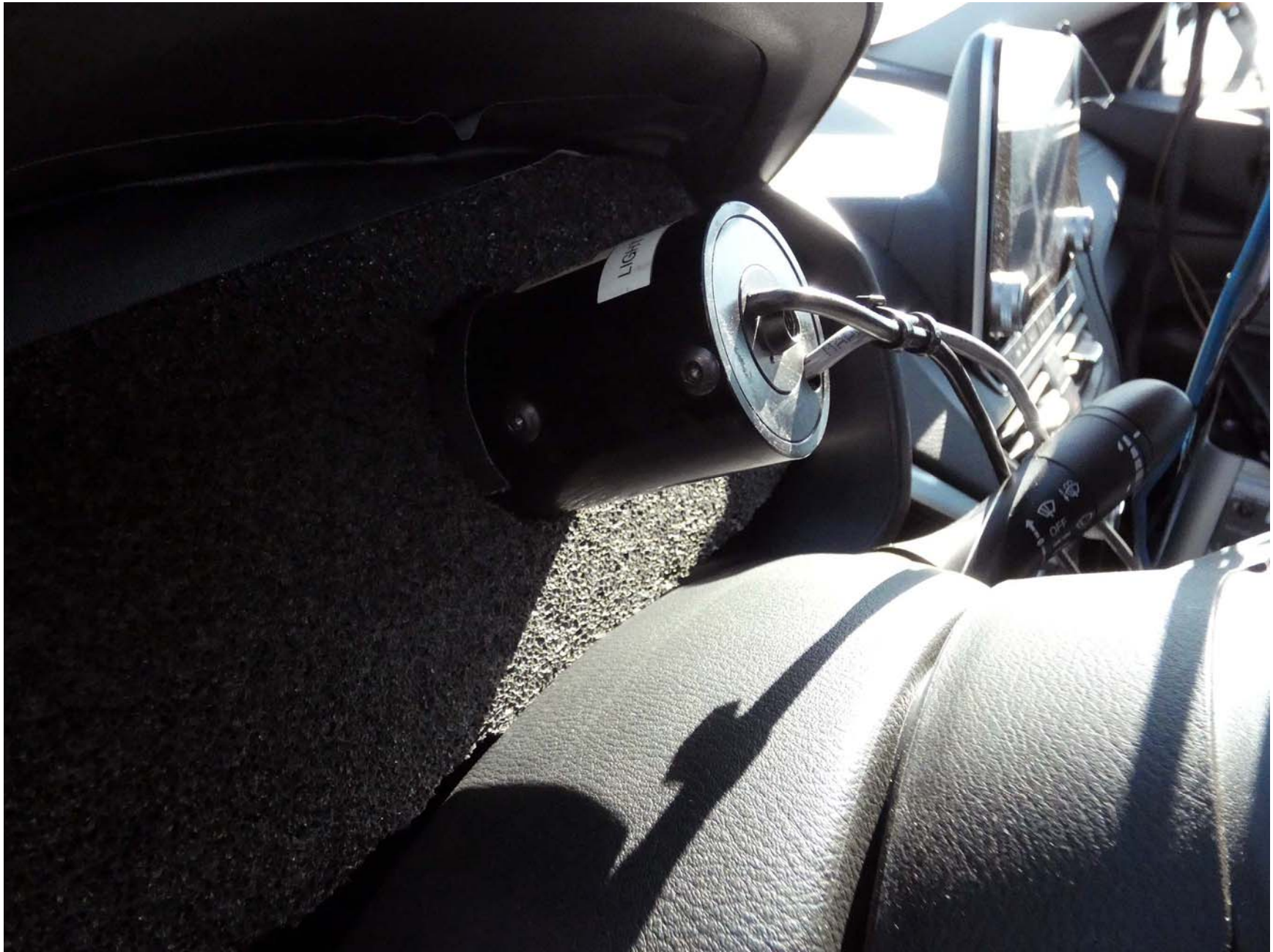
Figure A11. Sensor for Detecting Visual Alerts
