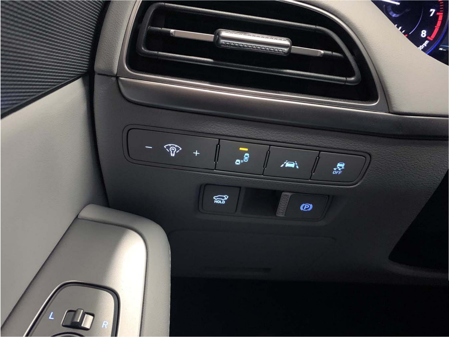
Figure A11. LKA (LDW) On/Off Switch
