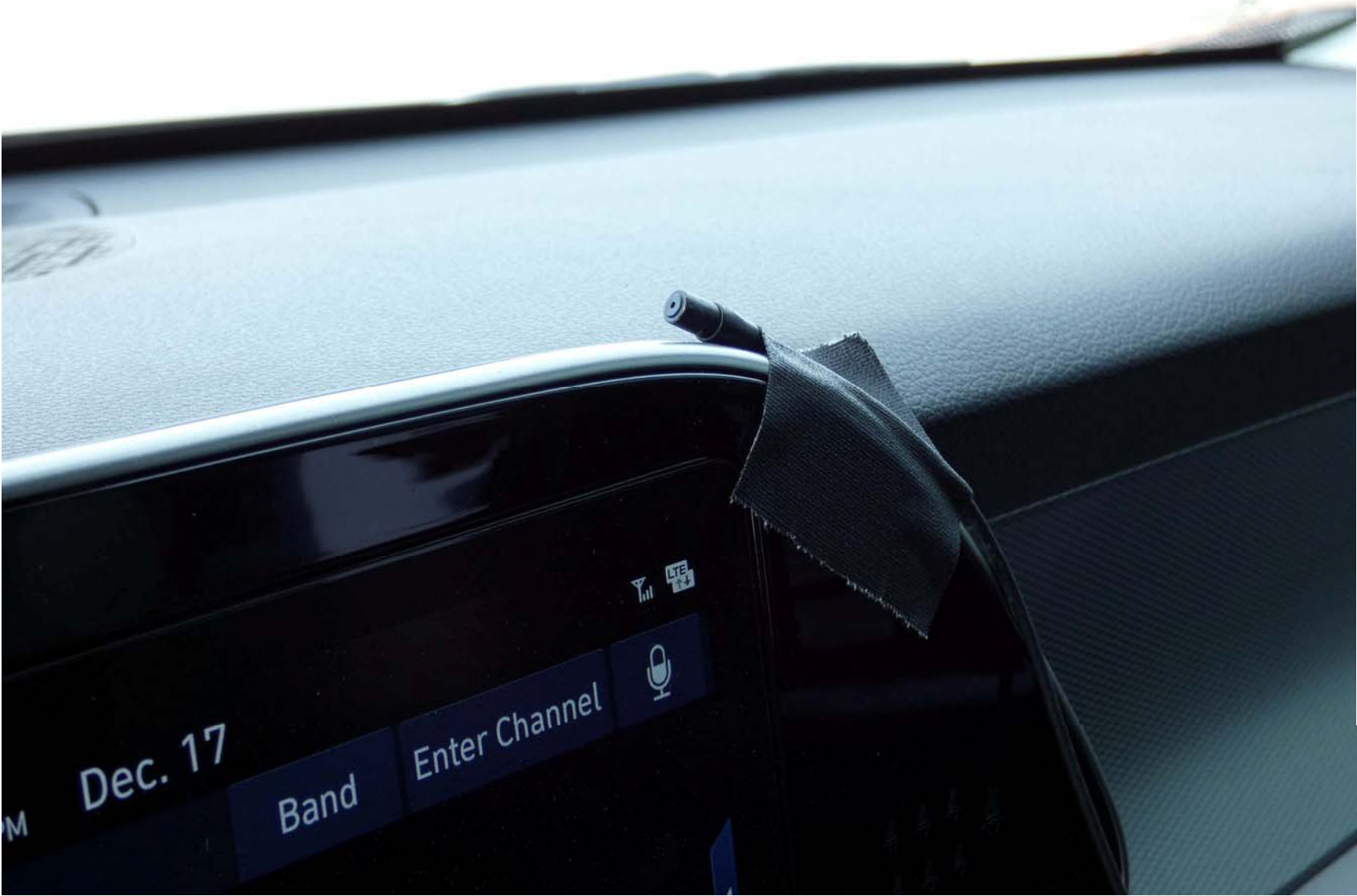
Figure A8. Sensor for Detecting Auditory Alerts
