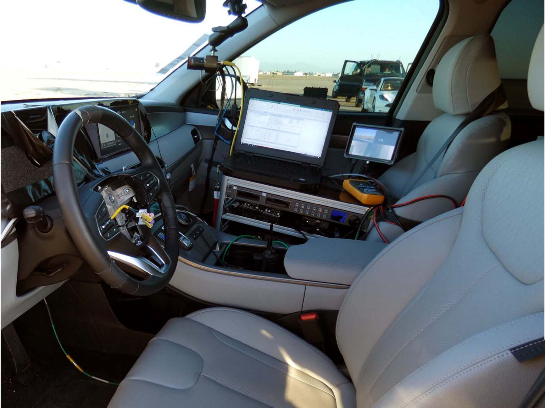
Figure A7. Computer Installed in Test Vehicle
