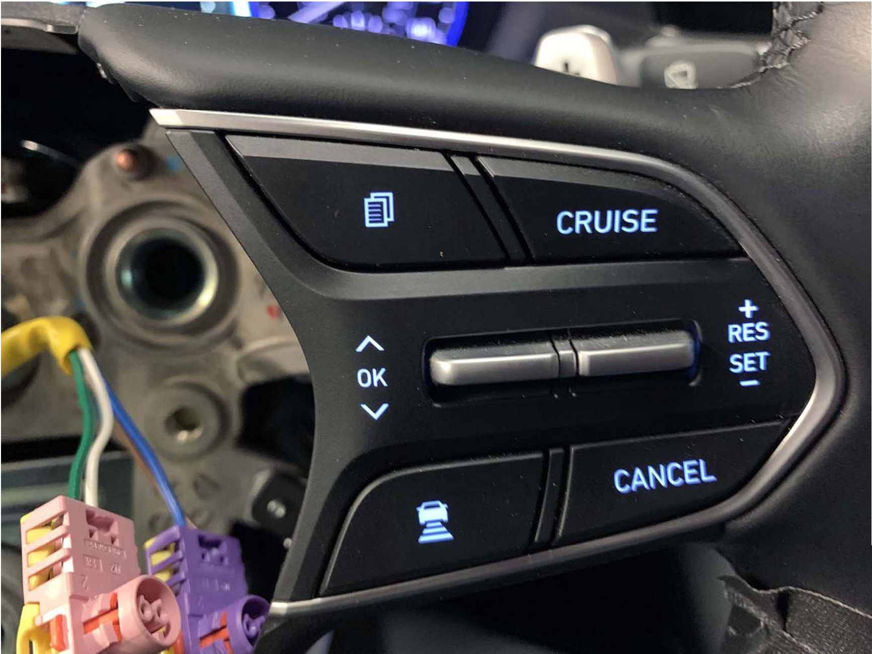
Figure A12. Steering Wheel Mounted Controls for Interacting with LKA (LDW) Settings
