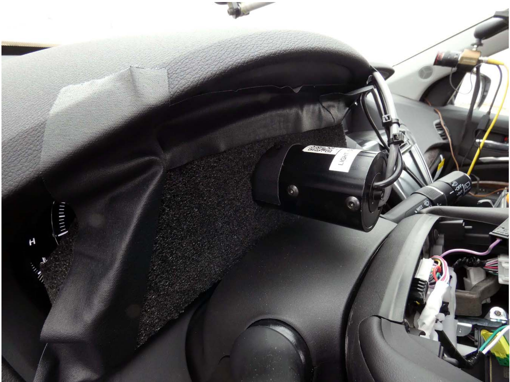
Figure A11. Sensor for Detecting Auditory Alerts
