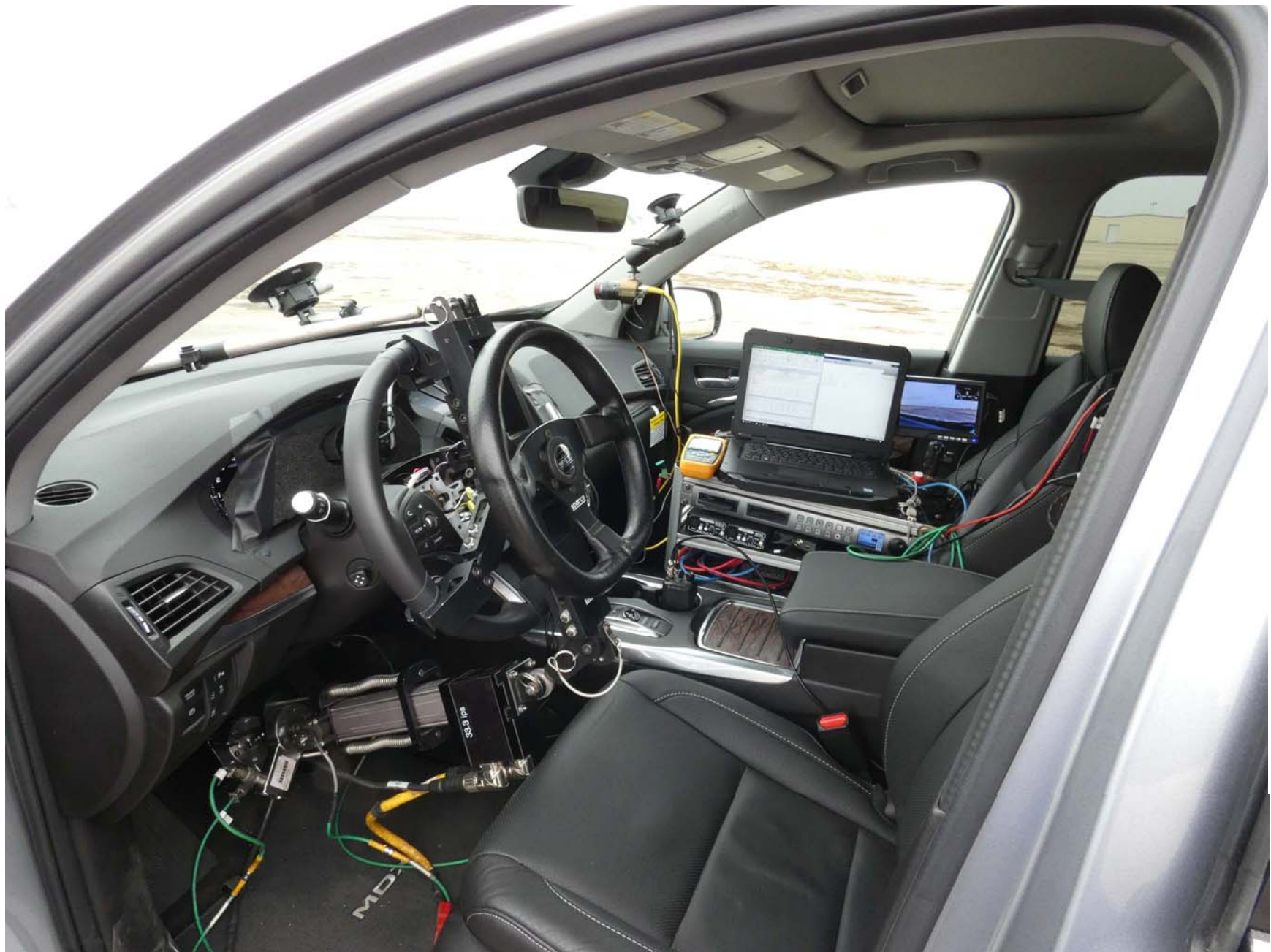
Figure A14. Computer and Brake Actuator Installed in Subject Vehicle
