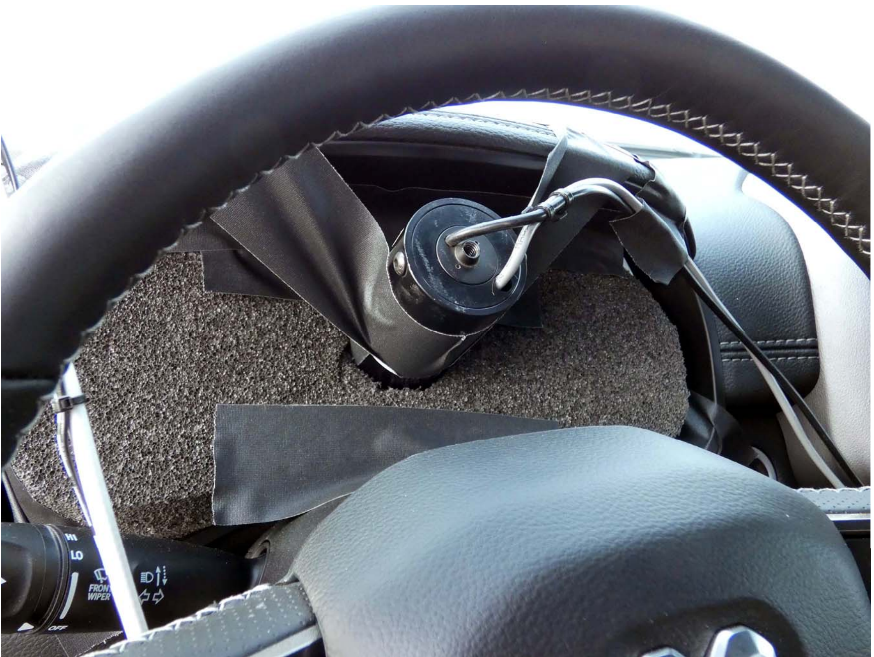
Figure A9. Sensor for Detecting Visual Alerts
