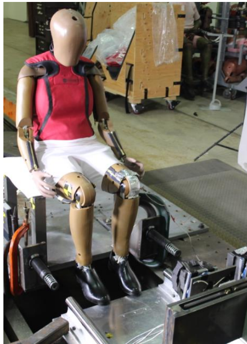
Figure 87. Front oblique view of pre-test dummy position
