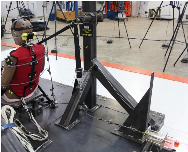
Figure 136. Shoulder belt load limiting mechanism
