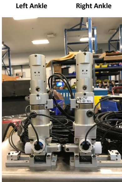
Figure 111. Y-axis potentiometer orientation
