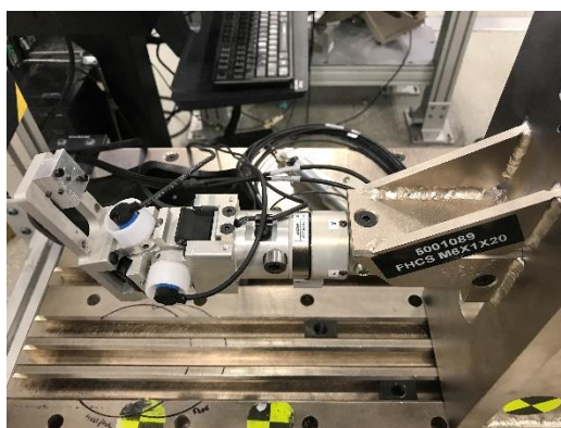
Figure 113. Lower leg mounted on rigid fixture
