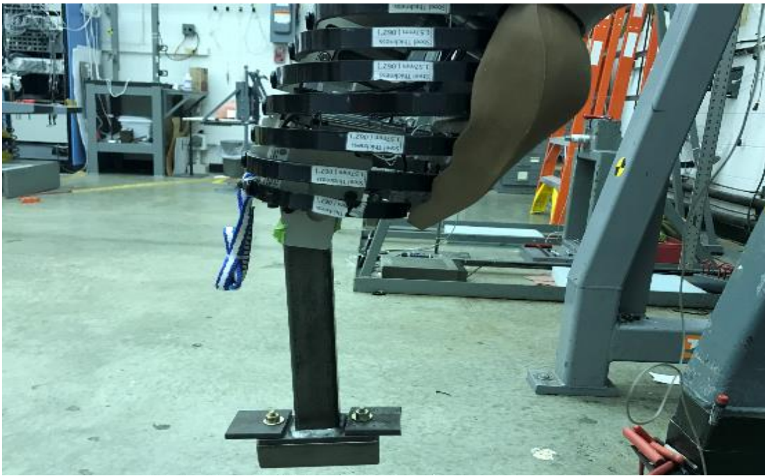
Figure 83. Mounted Head and Neck Structural Replacements
