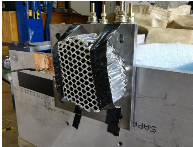
Figure 95. Pre-crushed Hexcel affixed on the impactor
