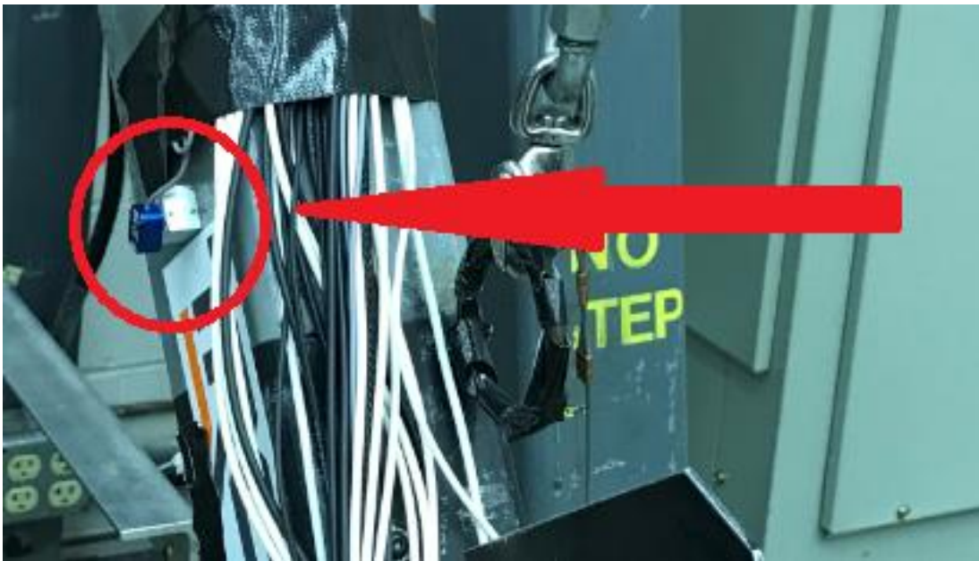
Figure 77. Pendulum ARS Mounted about the Y-axis
