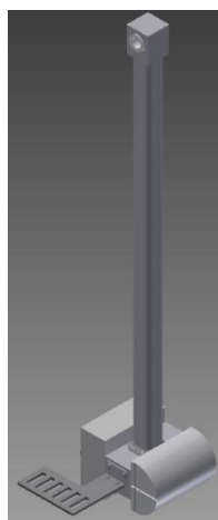
Figure 106. Example of dynamic impactor for THOR-05F ankle and foot tests (not to scale)
