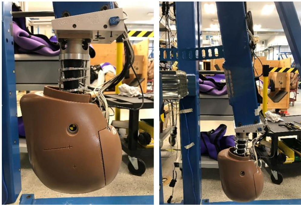
Figure 25. Neck flexion neck to neck plate alignment (left); Neck flexion test setup (right)
