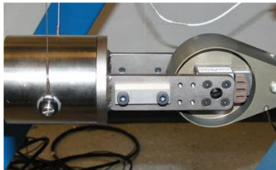
Figure 104. Alignment probe and distribution bracket impact surfaces
