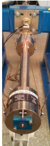
Figure 103. Lateral alignment of impact location
