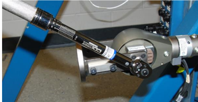
Figure 101. Knee joint bolt torque setting
