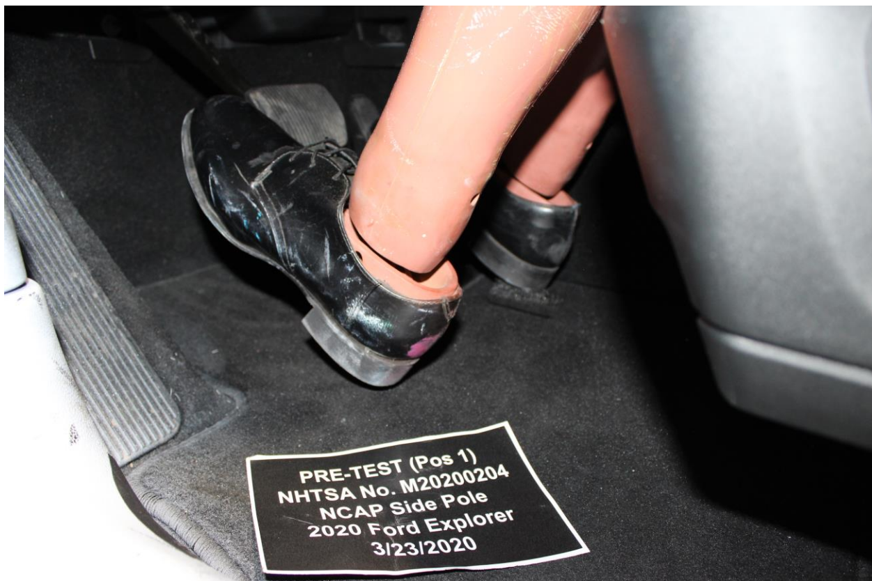
Figure A-32: Pre-Test Placement of Dummy's Feet
