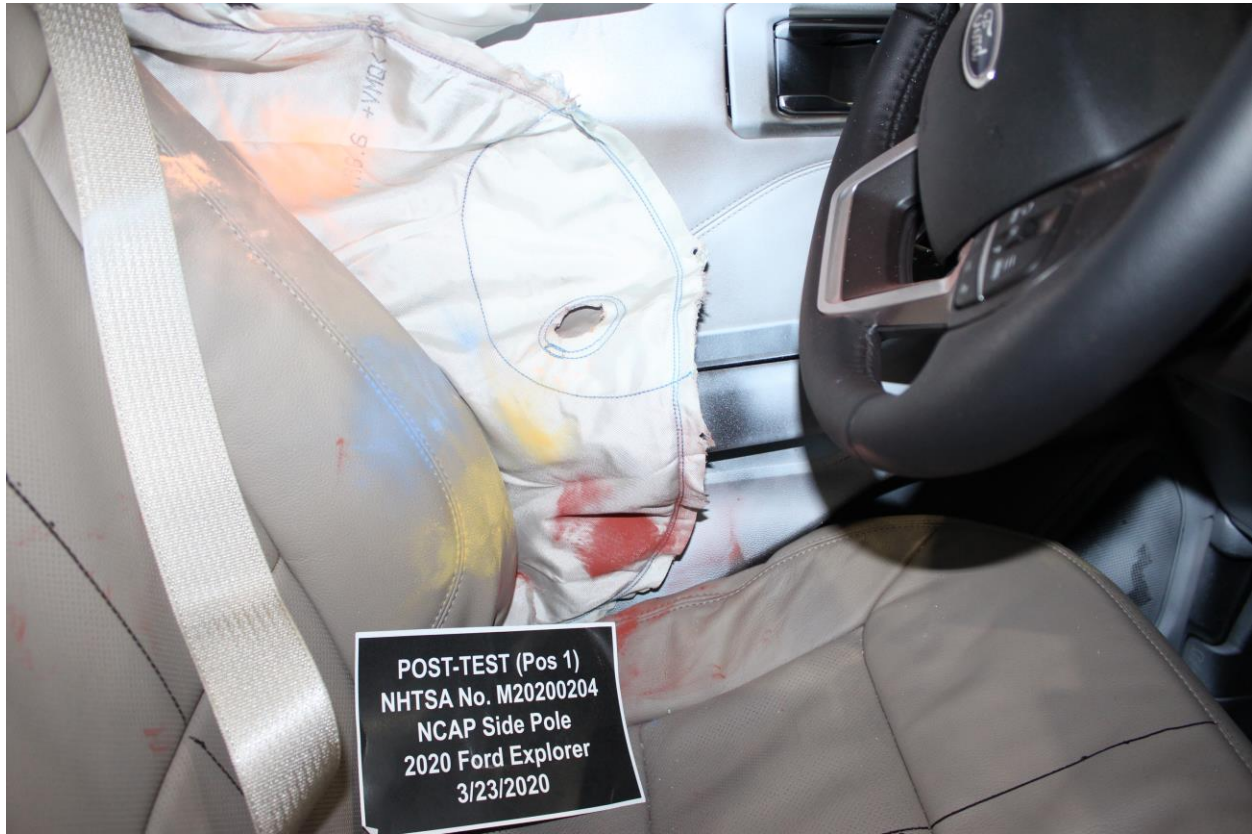
Figure A-49: Post-Test Dummy Close-Up Torso Contact with Side Airbag View
