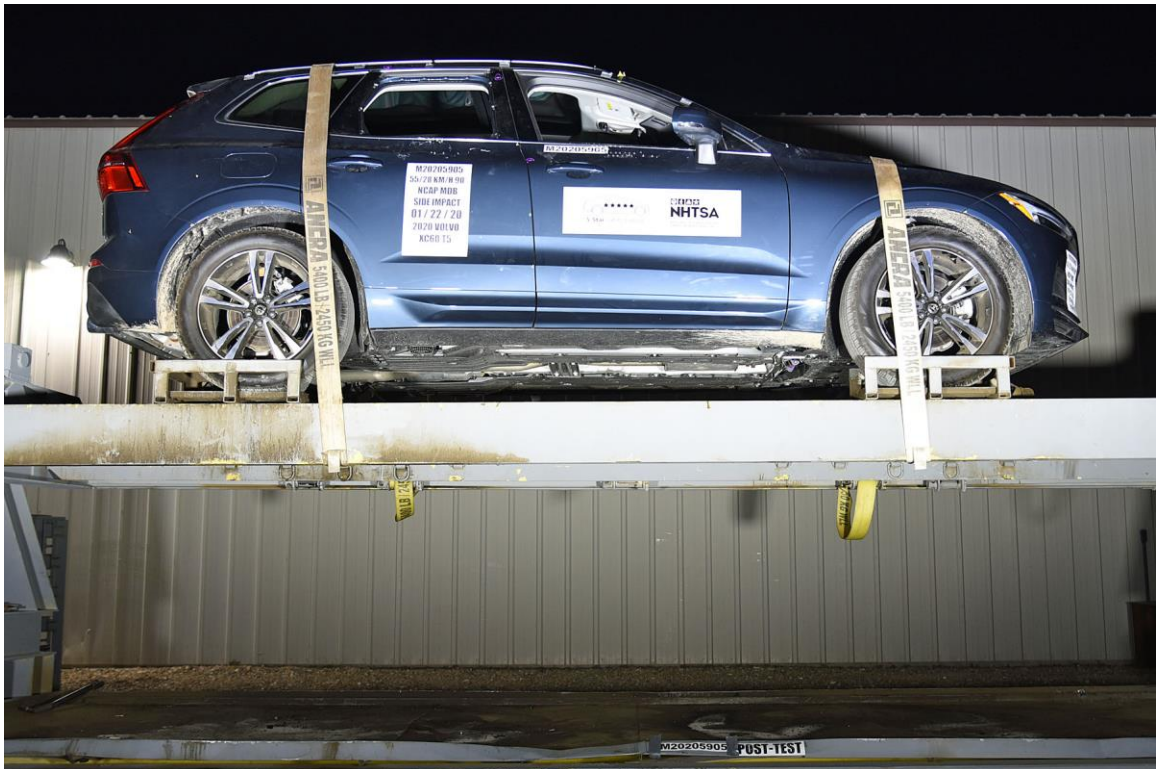
FIGURE 96. FMVSS No. 301 Static Rollover 0 Degrees
