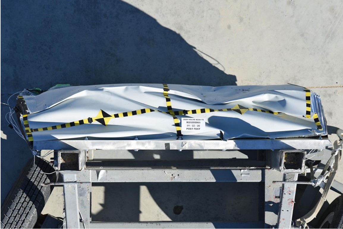
FIGURE 87. Post-Test Top View of MDB Impactor Face
