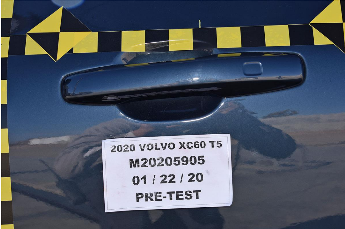
FIGURE 21. Pre-Test Left Front Door Latch Close-Up
