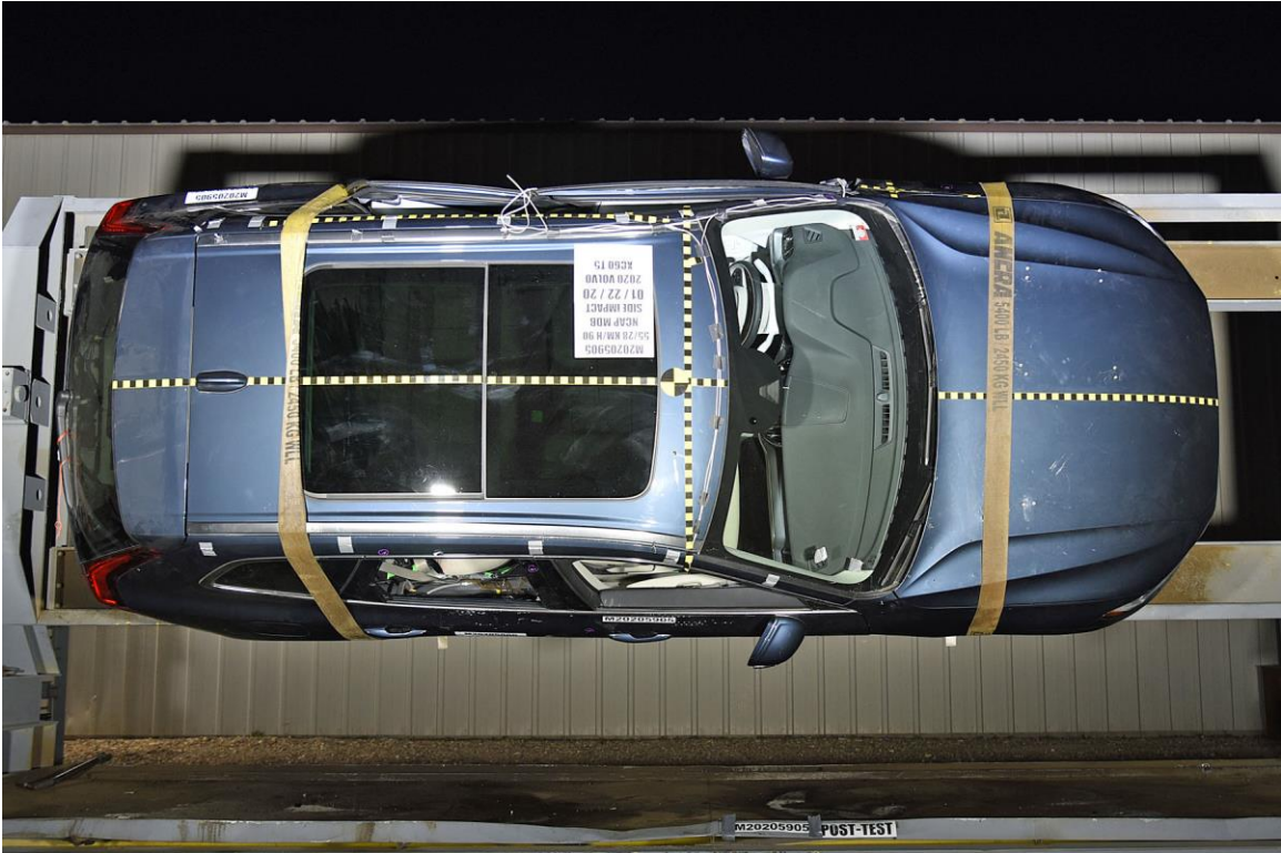
FIGURE 97. FMVSS No. 301 Static Rollover 90 Degrees
