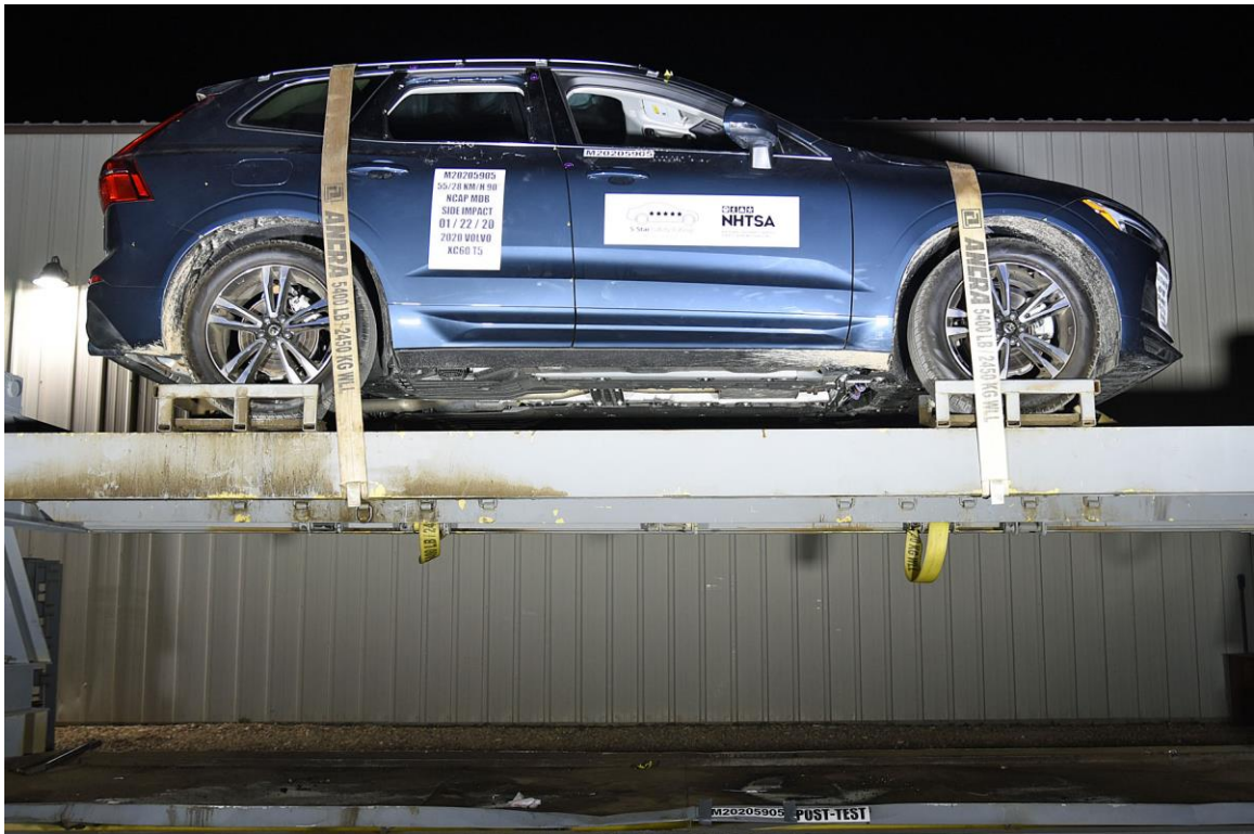
FIGURE 100. FMVSS No. 301 Static Rollover 360 Degrees
