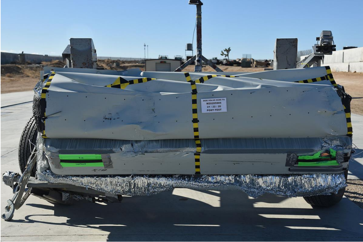
FIGURE 85. Post-Test Front View of MDB Impactor Face
